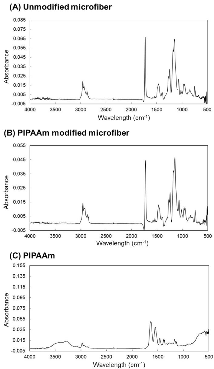
**Figure S3.** FT-IR spectra of (A) unmodified microfibers, (B) PIPAAm modified microfibers, and (C) PIPAAm.
