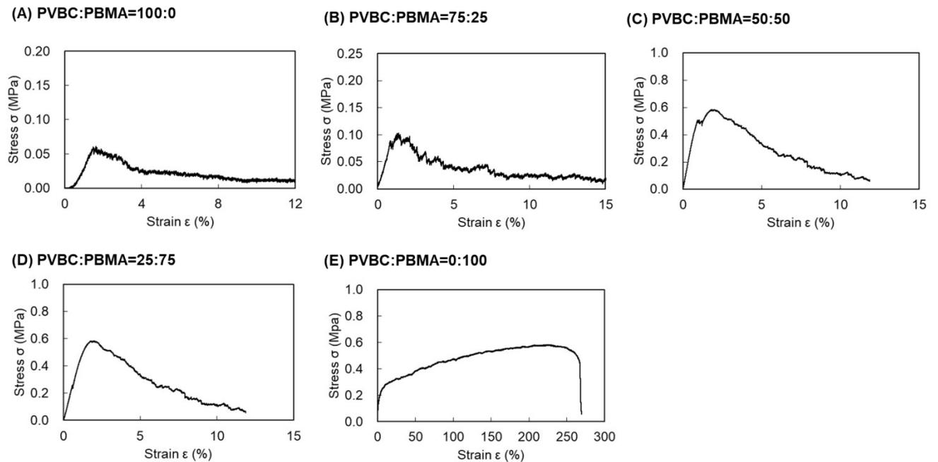
**Figure S1.** Stress-strain curves of the prepared fibers. (A) PVBC:PBMA = 100:0, (B) PVBC:PBMA = 75:25, (C) PVBC:PBMA = 50:50, (D) PVBC:PBMA = 25:75, and (E) PVBC:PBMA = 0:100.
