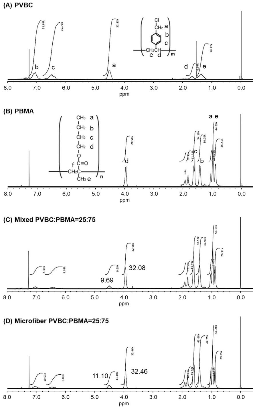
**Figure S2.**  $^1\text{H}$  NMR spectra in  $\text{CDCl}_3$ , (A) PVBC, (B) PBMA, (C) mixed PVBC and PBMA at a composition of 25:75, and (D) microfiber composed of PVBC and PBMA at a composition of 25:75.
