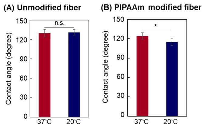
**Figure S4** Contact angle values of microfibers (PVBC:PBMA = 25:75) measured by a sessile drop method before (A) and after (B) PIPAAm modification. (\*  $0.01 < p < 0.05$ ; n.s. indicates differences that are not significant with  $p > 0.05$ ,  $n = 5$ ).
