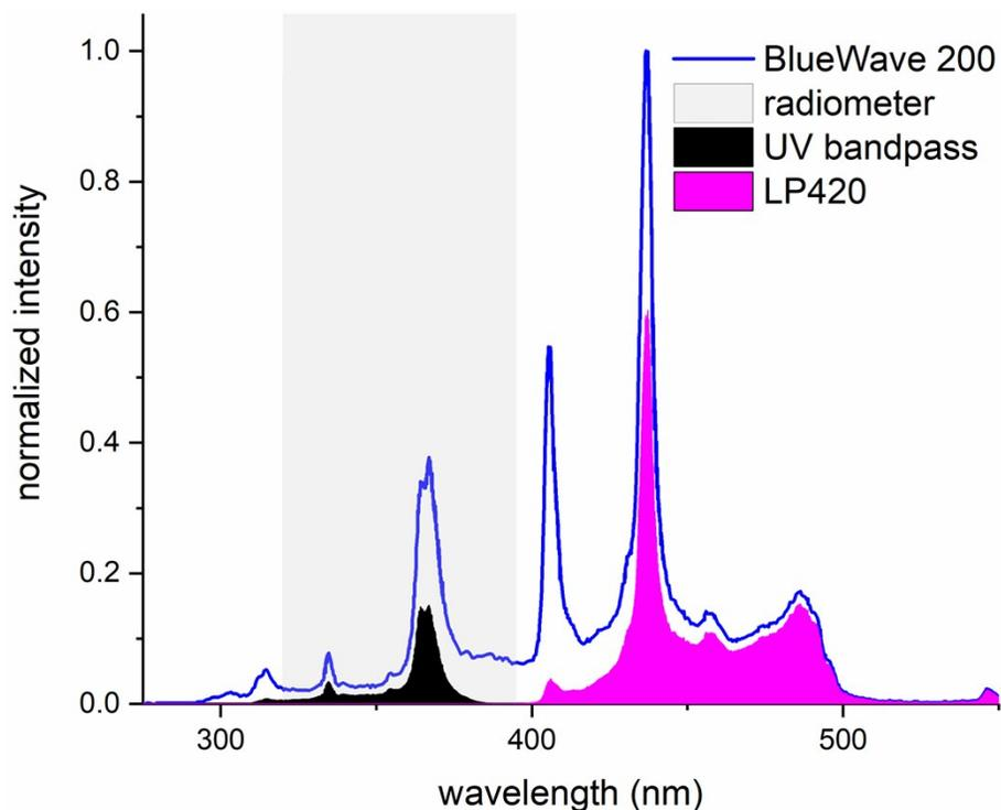
**Fig. S4** Spectra of Dymax BlueWave 200 curing lamp and corresponding filtered outputs using UV bandpass (BP305-390) and LP420 filters.
