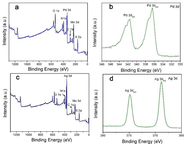
**Fig. S3** XPS full spectrum of PPy@MoS<sub>2</sub>@Pd (a) and PPy@MoS<sub>2</sub>@Ag(c), (b) XPS spectra of Pd 3d of PPy@MoS<sub>2</sub>@Pd and (d) XPS spectra of Ag 3d of PPy@MoS<sub>2</sub>@Ag.
