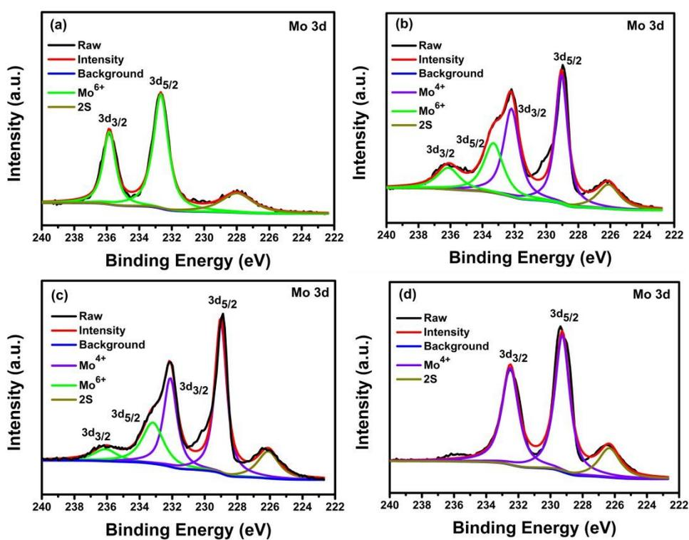
**Fig. S6** XPS spectra of the Mo 3d for PPy@MoS<sub>2</sub> composites at different reaction time: (a) 3 h, (b) 6 h, (c) 12 h, and (d) 24h.
