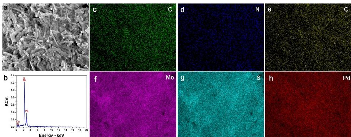
**Fig. S5** SEM images and the corresponding EDS elemental mappings of C, N, O, Mo, S and Pd in PPy@MoS<sub>2</sub>@Pd.
