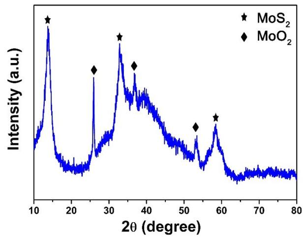
**Fig. S9** XRD of diffraction patterns of C@MoO<sub>2</sub>@MoS<sub>2</sub>-50.
