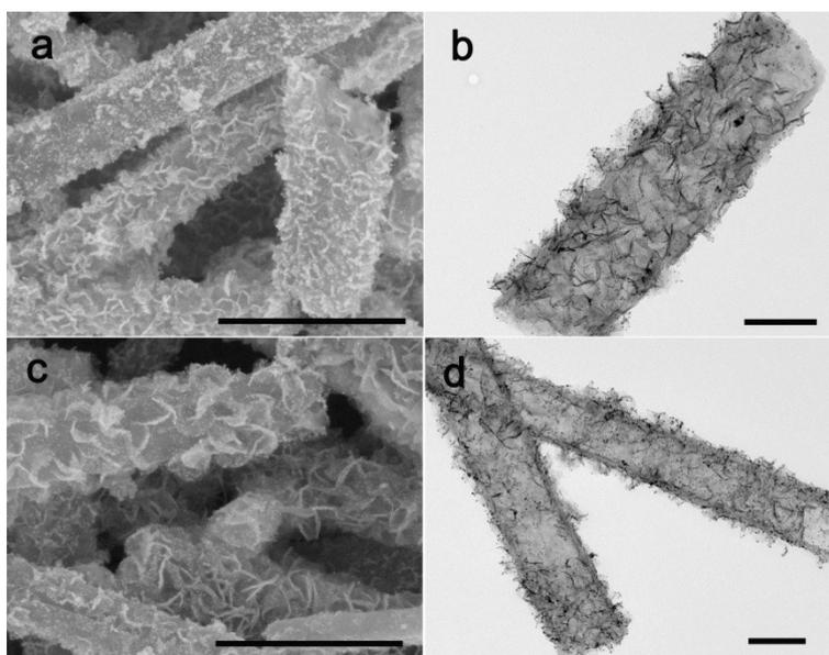
**Fig. S2** SEM and TEM images of PPy@MoS<sub>2</sub>@Au, 2 mg (a, b) and 4 mg (c, d). Scale bars: 1  $\mu$ m in (a, c), and 200 nm in (b, d).
