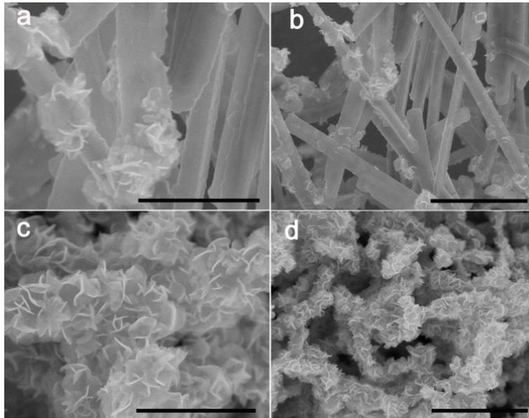
**Fig. S8** SEM images of C@MoO<sub>2</sub>@MoS<sub>2</sub>-100 (a, b) and C@MoO<sub>2</sub>@MoS<sub>2</sub>-50 with the MoO<sub>2</sub>@C as precursor (c, d) Scale bars: 1  $\mu$ m in (a, c) and 2  $\mu$ m in (b, d).
