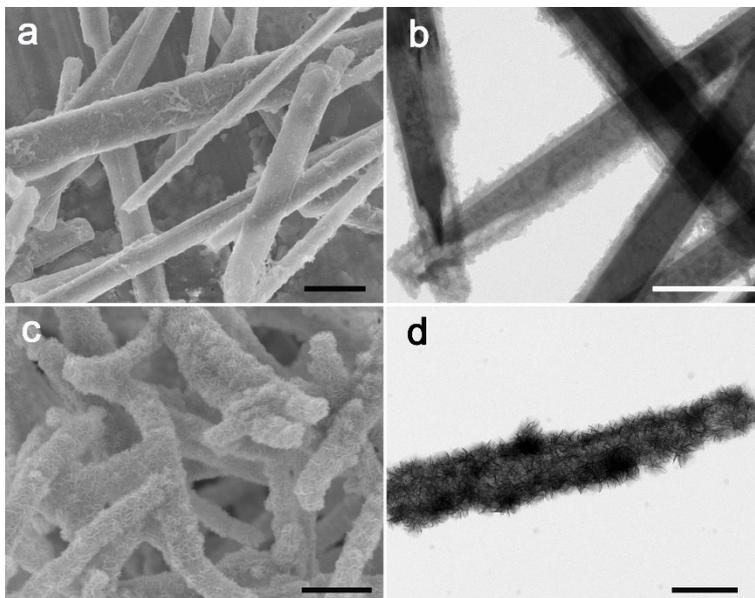
**Fig. S1** SEM and TEM images of MoO<sub>3</sub>@PANI (a, b) and PANI@MoS<sub>2</sub> (c, d). Scale bars: 1  $\mu$ m in (a, c) and 500 nm in (b, d).
