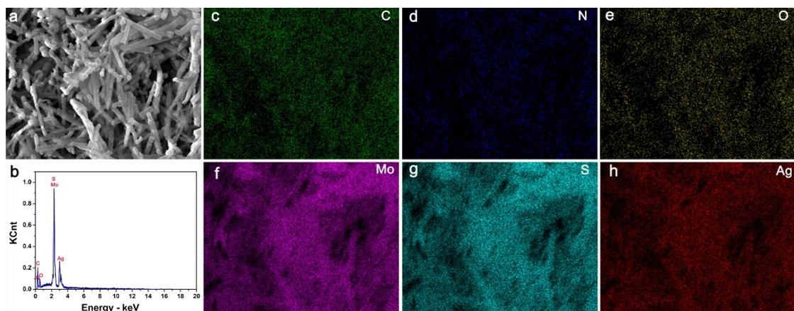
**Fig. S4** SEM images and the corresponding EDS elemental mappings of C, N, O, Mo, S and Ag in PPy@MoS<sub>2</sub>@Ag.
