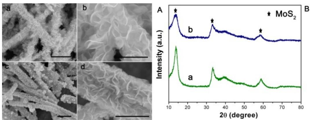
**Fig. S10** (A) SEM images of PPy@MoS<sub>2</sub> with MoO<sub>3</sub>@PPy-50  $\mu$ L (a, b) and 150  $\mu$ L (c, d). Scale bars: 1  $\mu$ m in (a, c), and 500 nm in (b, d). (B) XRD of diffraction patterns PPy@MoS<sub>2</sub>-50  $\mu$ L(a); 150  $\mu$ L (b).
