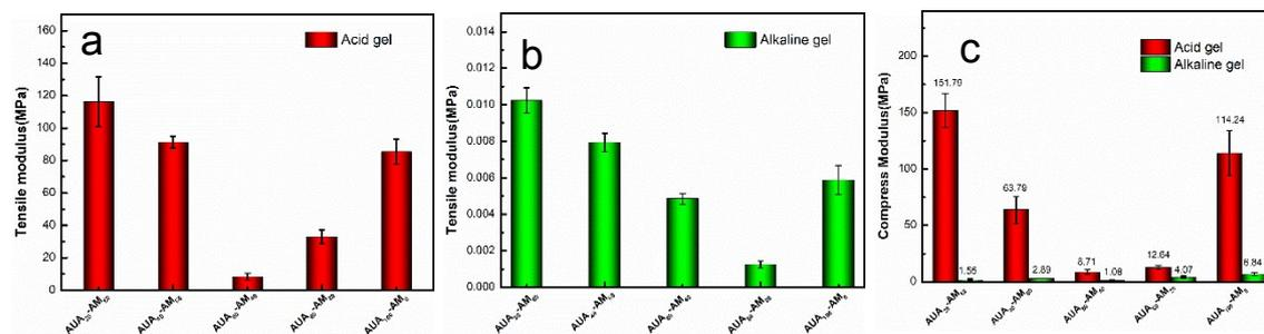
**Fig.S2** Tensile and compressive modulus of acid gel and alkaline gel;(a) Tensile modulus of acid gel; (b) Tensile modulus of alkaline gel; (c) Comparison of Compression modulus of acid gel and alkaline gel.
