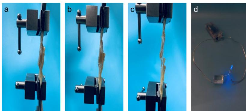
**Fig.S4** (a-c) Hydrogel adhesion test process; (d) Hydrogel can light the bulb at 3V
