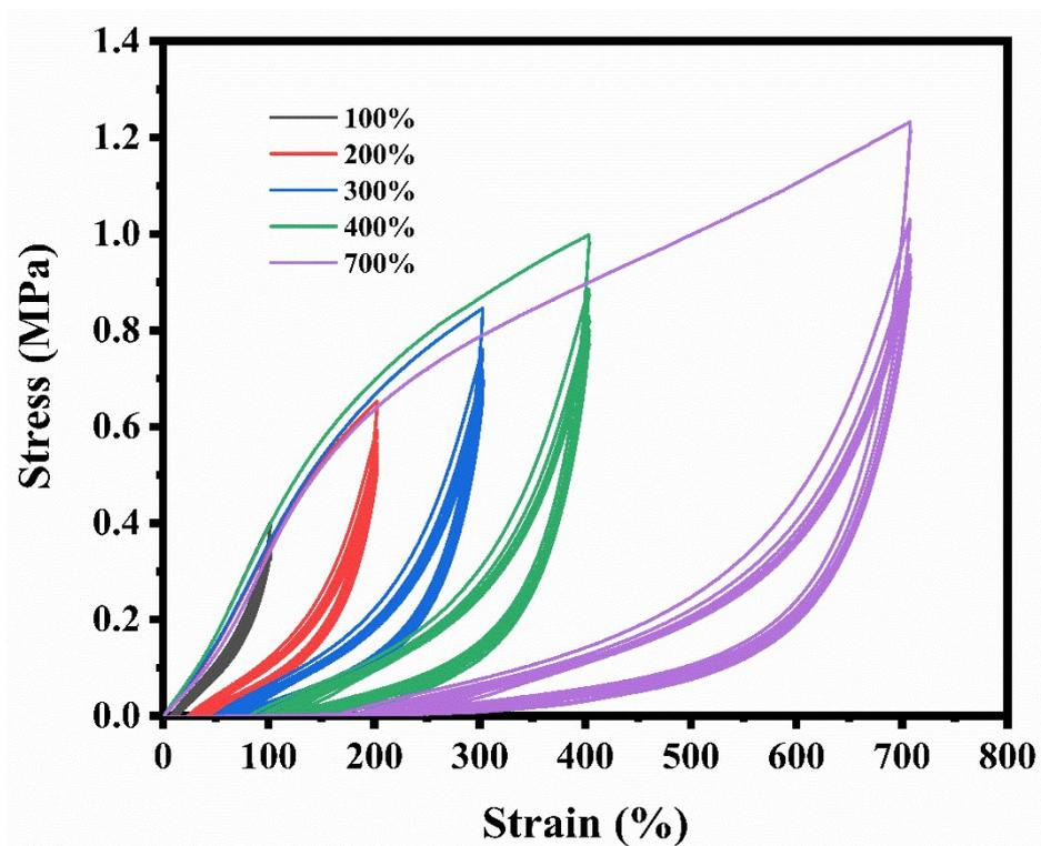
**Figure S6.** Stress-strain curves of PNAGA-30 & LiCl hydrogels under various strains cycles (a total of ten cycles).
