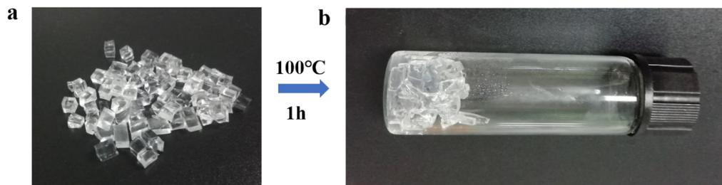
**Figure S3.** (a) The fragments of PNAGA-30 hydrogels. (b) The fragments were packed in sealed bottles and heated in 100 °C oil bath at atmospheric pressure for 1 h.
