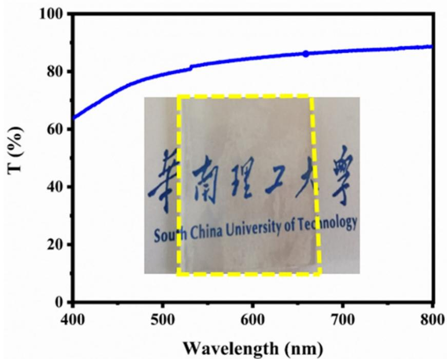
**Figure S5.** Optical transmittance of the PNAGA-30&1.2wt%LiCl hydrogels versus wavelength (the words under hydrogel sheet were indicated by yellow dotted lines for clear observation).
