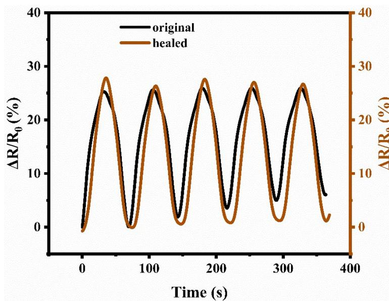
**Figure S7.** Relative resistance changes of the original and self-healed PNAGA-30 & LiCl hydrogel-based strain sensors at a large strain of 400% for five cycles.
