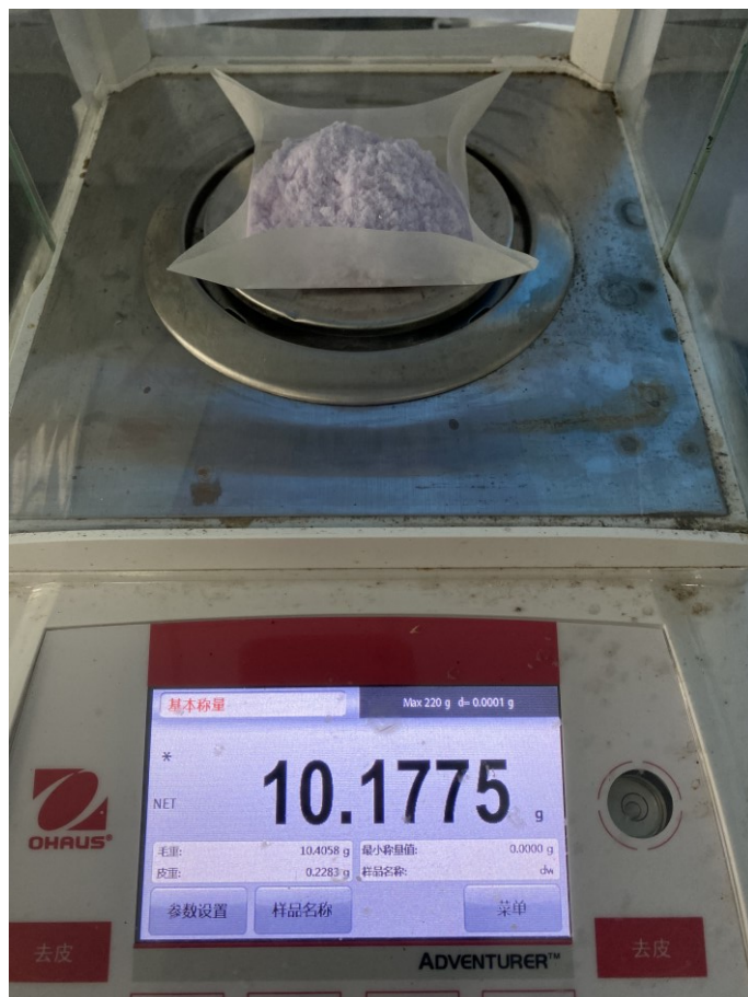
Fig. S1 Gram-scale synthesis of Nd-DTPA via a green and mild method through the reaction of \text{Nd}_2\text{O}_3 and DTPA.
