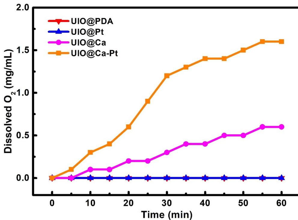
**Fig. S14.** Oxygen concentration changes of UIO@PDA, UIO@Pt, UIO@Ca and UIO@Ca-Pt solutions in the absence of  $H_2O_2$ .
