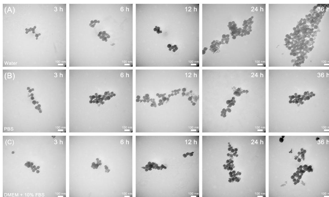
**Fig. S11.** TEM images of UIO@Ca-Pt after incubating with water (A), PBS (B) or DMEM containing 10% FBS (C) for 3, 6, 12, 24 or 48 h.
