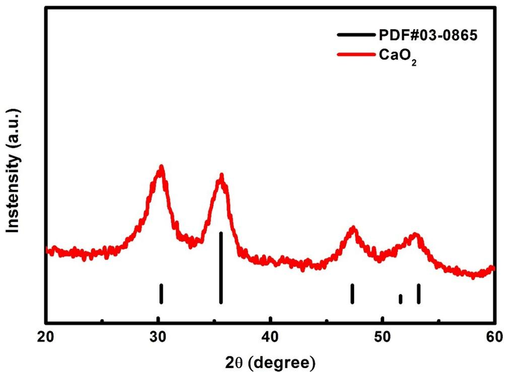
Fig. S5. XRD patterns of  $\text{CaO}_2$  NPs.
