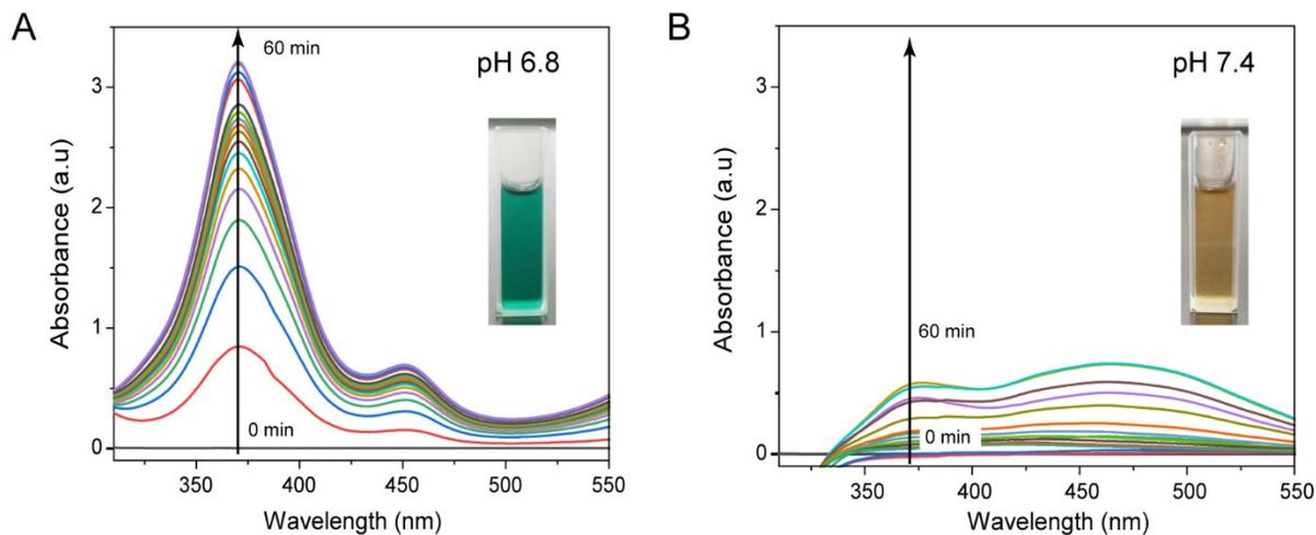
**Figure S4.** Analysis of pH-responsive membrane selective permeability based on oxidized TMB color absorbance intensity evaluation at 370 nm as the product of cascade reactions of Cis/GOD@Bz-V (GOD: 50 mU/mL) after being incubated in PBS solution in the presence of glucose (1 mg/mL), HRP (150 mU/mL), and TMB (100  $\mu$ M) at pH 7.4 or pH 6.8. The inset digital images show the color of the solution at pH 6.8 7.4 after 1 h of incubation.
