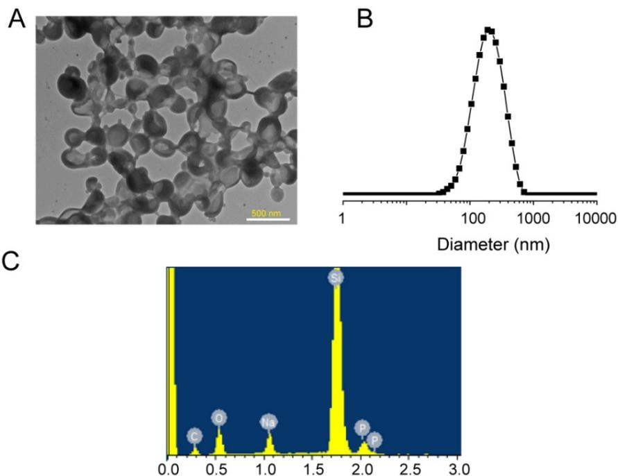
**Figure S1.** (A) TEM image, (B) size distribution by DLS and (C) SEM element analysis of PEG<sub>113</sub>-*b*-P(BzMA<sub>120</sub>-*co*-PEMA<sub>21</sub>) vesicle.
