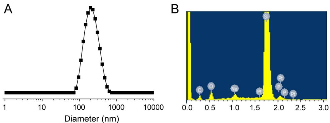
**Figure S2.** (A) Size distribution test by DLS. (B) SEM element analysis of cisplatin and GOD-co-loaded PEG<sub>113</sub>-*b*-P(BzMA<sub>120</sub>-*co*-PEMA<sub>21</sub>) polymersomes (Cis/GOD@Bz-V).
