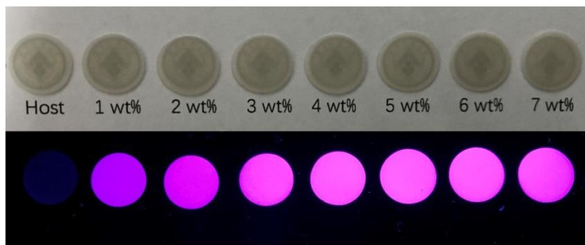
**Fig. S3** Photographs of BSMS-PiG plates with different phosphor doping concentrations under fluorescent light and 365 nm UV light, respectively.
