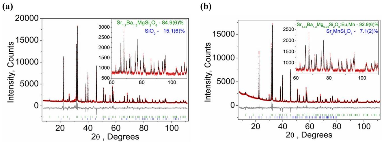
**Fig. S1** Difference Rietveld plot of: (a)  $\text{Sr}_{1.7}\text{Ba}_{1.3}\text{MgSi}_2\text{O}_8$ ; (b)  $\text{Sr}_{1.64}\text{Ba}_{1.3}\text{Eu}_{0.06}\text{Mg}_{0.94}\text{Mn}_{0.06}\text{Si}_2\text{O}_8$ .
