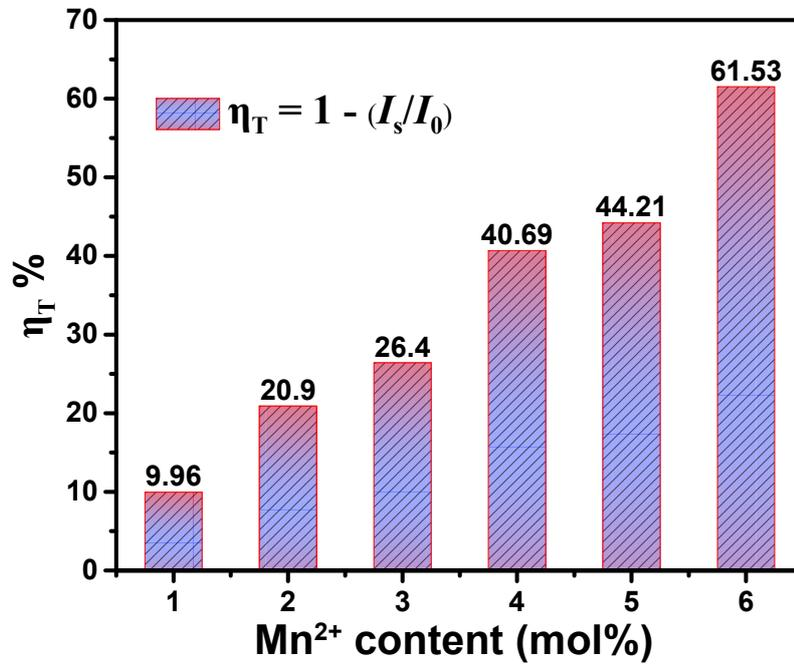
**Fig. S5** Variation in  $\eta_T$  for  $\text{Ba}_{1.3} \text{Sr}_{1.7} \text{MgSi}_2 \text{O}_8: 6\% \text{Eu}^{2+}, y\% \text{Mn}^{2+}$  ( $1 \leq y \leq 6$ ) with  $\text{Mn}^{2+}$  concentration
