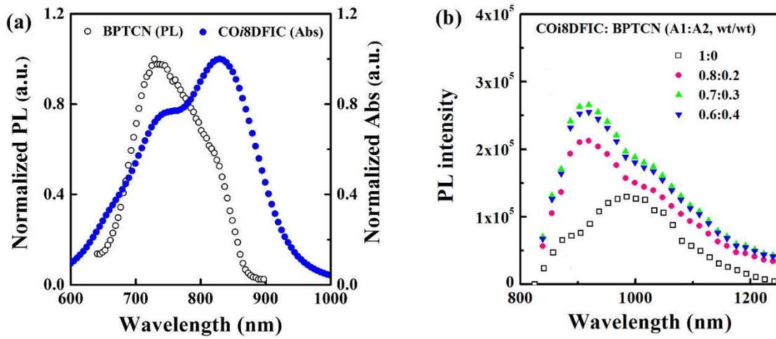
**Fig. S7.** UV-Vis-NIR absorption spectra of the thin films of COi8DFIC (A1), **BPTCN** (A2) and their blends (wt/wt), spin-cast on quartz glass from 10 mg mL<sup>-1</sup> CHCl<sub>3</sub> solution (total concentration) at a speed of 2000 rpm.
