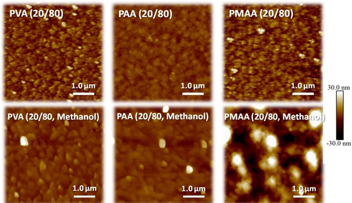
**Fig. S5** C-AFM topography images of the PEDOT:PSS/soft polymers blends (20/80) before and after methanol treatment.
