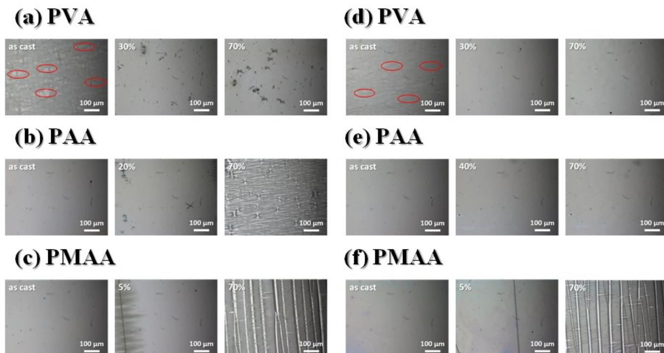
**Fig. S4** OM images of the PEDOT:PSS/soft polymer blends (20/80) thin film at different tensile strains: (a) to (c) for Original, (d) to (f) for Methanol.
