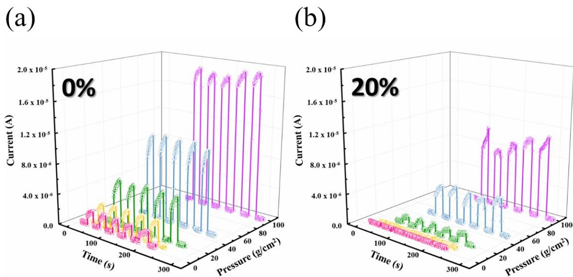
**Fig. S8** Pressure sensor performance of the PEDOT:PSS/PAA (20/80, Original) at the (a) 0%, (b) 20%.
