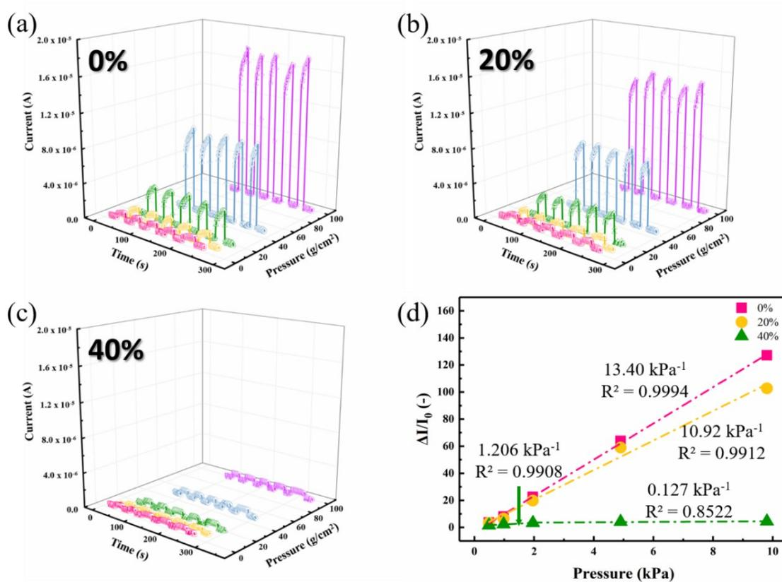
**Fig. S9** Pressure sensor performance of the PEDOT:PSS/PVA (20/80, Original) at the (a) 0%, (b) 20% (c) 40% tensile strains, and (d) linear fitting sensitivity.
