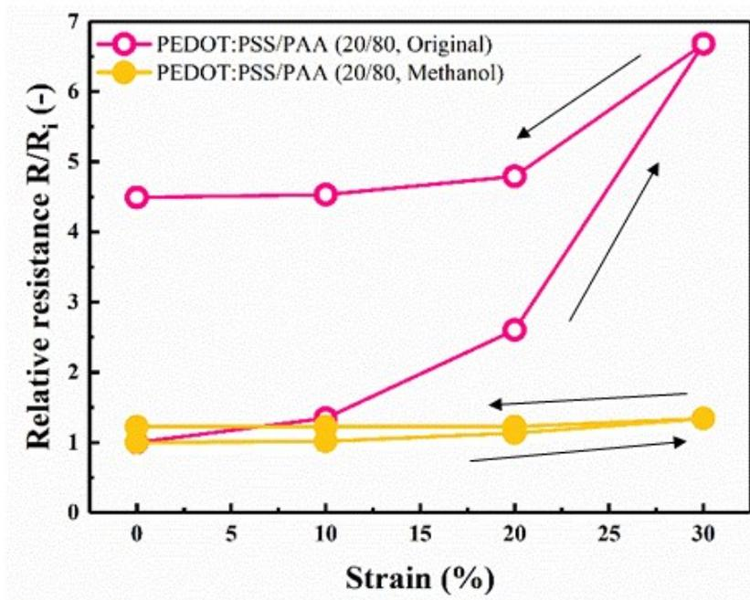
Fig. S1  $R/R_i$  under the first cycle for PEDOT:PSS/PAA (20/80) before and after methanol treatment.
