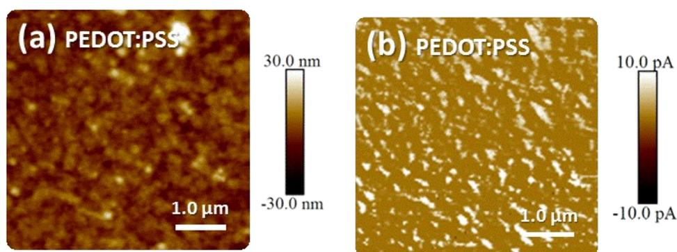
**Fig. S6** C-AFM (a) topography images and (b) current images for pristine PEDOT:PSS.
