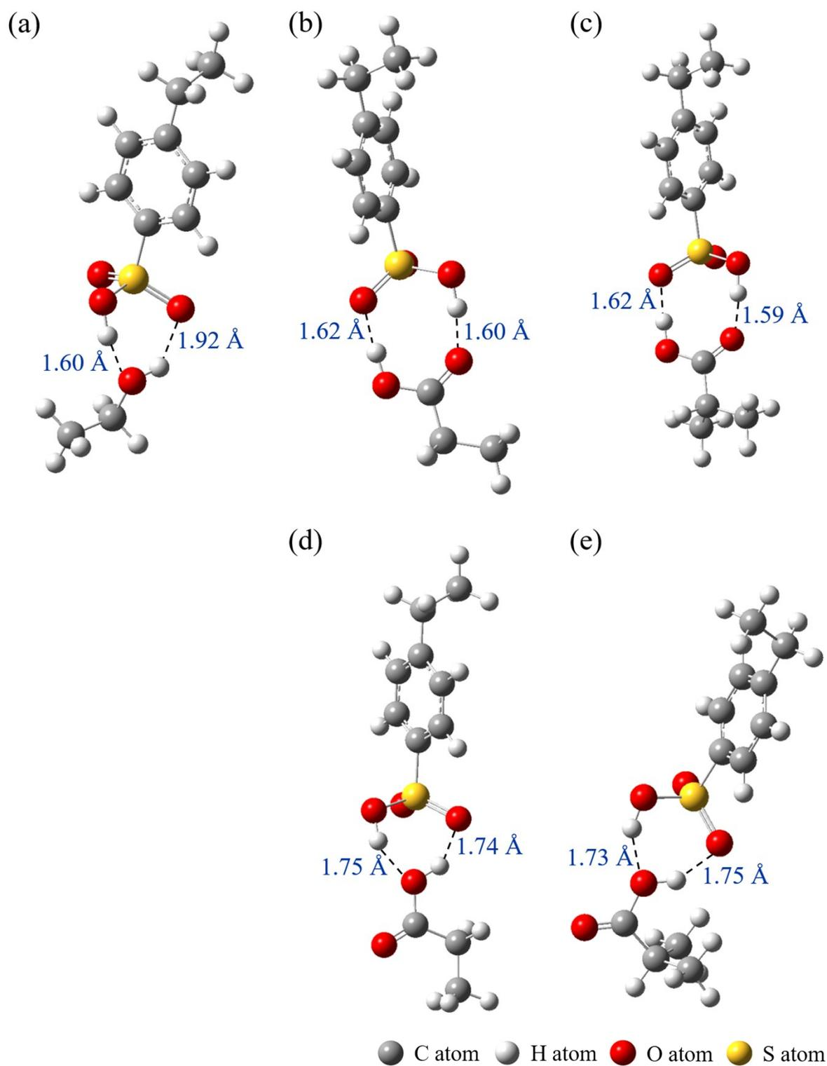
**Fig. S7** Gaussian simulation of the interaction between monomers of (a) PSS-PVA, (b) and (d) PSS-PAA, (c) and (e) PSS-PMAA.
