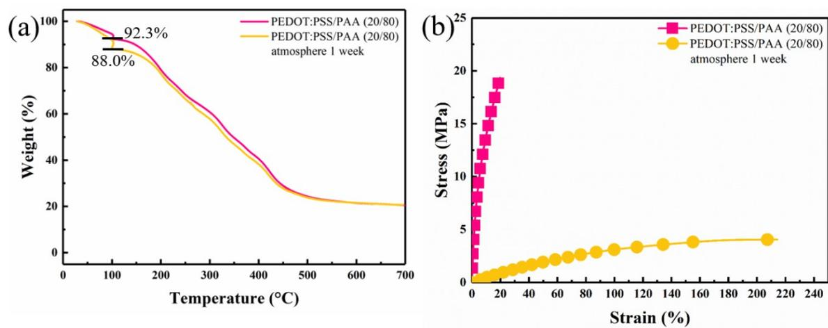
**Fig. S3** Moisture absorption test: (a) TGA and (b) stress strain curves of the PEDOT:PSS/PAA (20/80, Original) free standing bulk film stored in atmosphere 1 week before tested.
