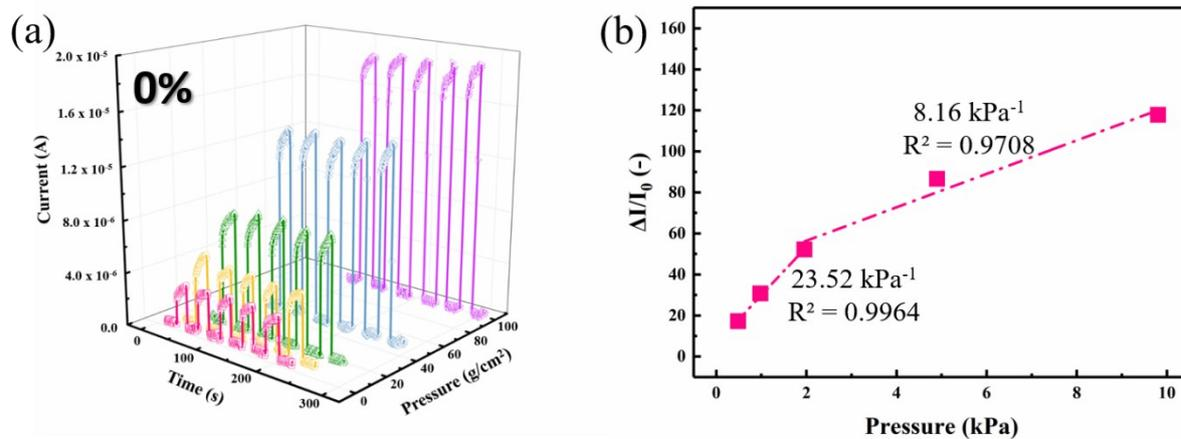
**Fig. S10** Pressure sensor performance of the PEDOT:PSS/PMAA (20/80, Original) at the (a) 0% tensile strain and (b) linear fitting sensitivity.
