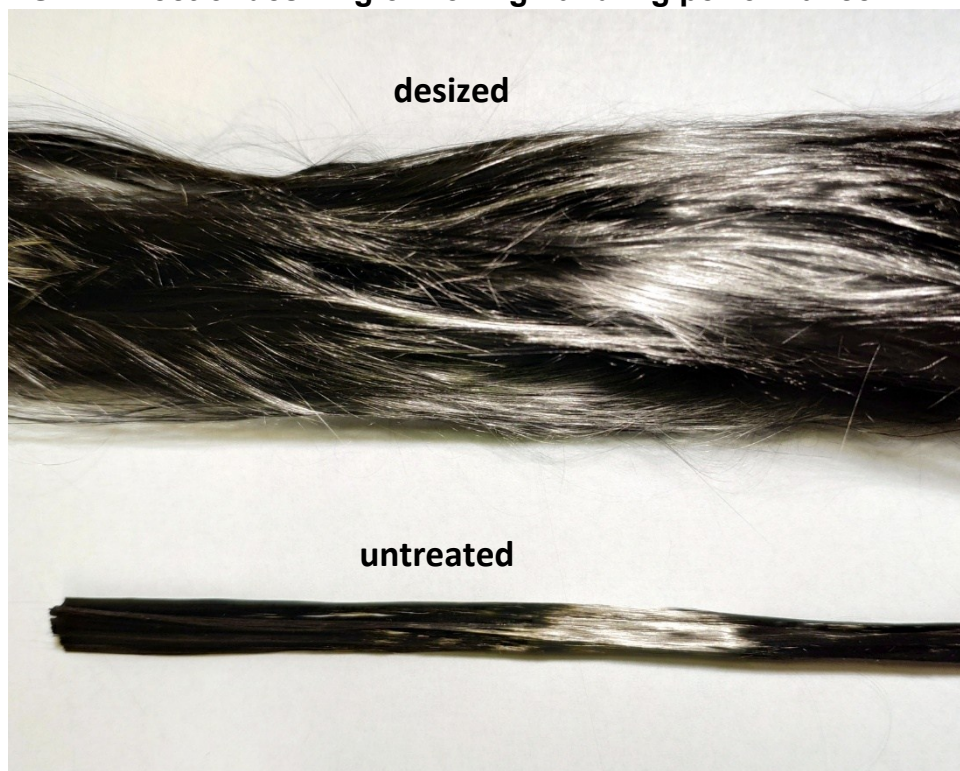
Fig. ESI-1. Desized (top) vs untreated 48k roving (bottom).
