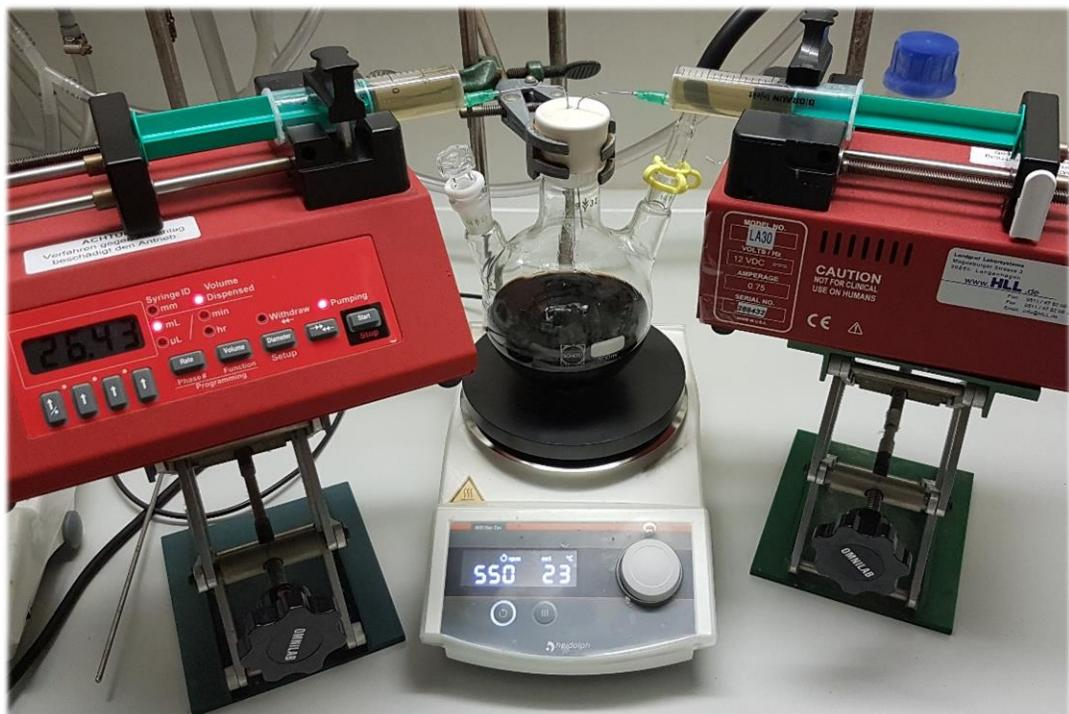
**Figure S1:** Addition of TMPMgCl·LiCl *via* syringe pumps at 23 °C to a 60 mmol (12.0 g) scale of **1-Oxa**.
