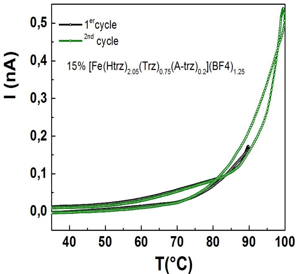
Figure S15. Pyroelectric discharge cycle for a polarized composite **5a**
