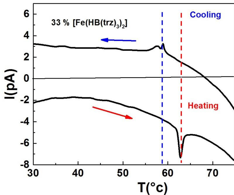
Figure S16. Pyroelectric discharge cycle for a polarized composite **5b**
