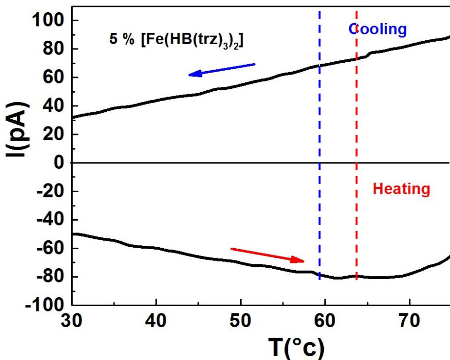
Figure S21. Pyroelectric discharge cycle for polarized composite **5a-5e**
