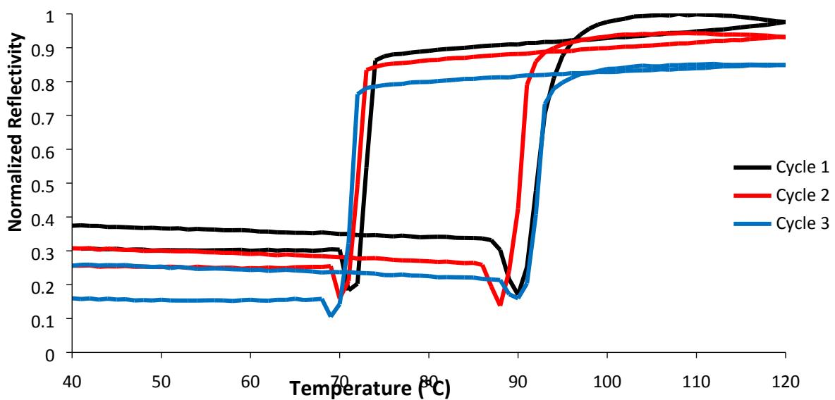
Figure S10: Variable temperature optical reflectivity measurement of the P(VDF-TrFE)/SCO composite
