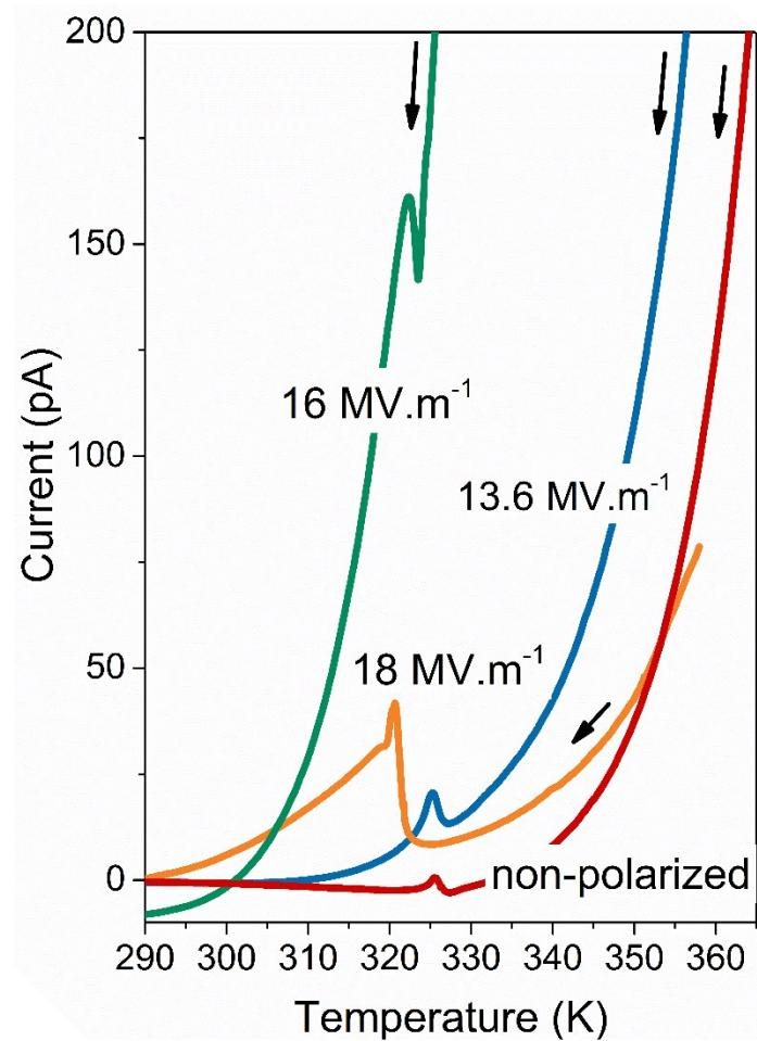
Figure S13. Pyroelectric discharge cycle for a polarized composite **3a**.
