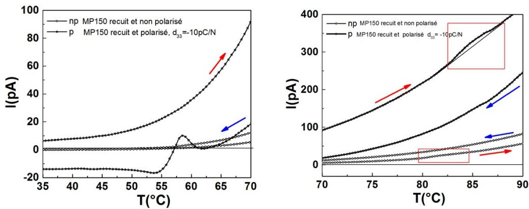
Figure S12: Pyroelectric discharge cycle for composite **2a** with different polarization intensities:
