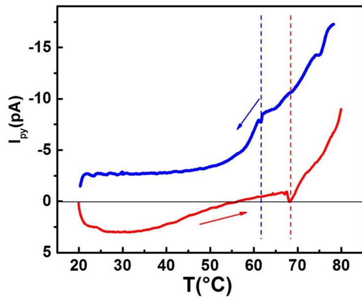
Figure S17. Pyroelectric discharge cycle for a polarized composite **5c**
