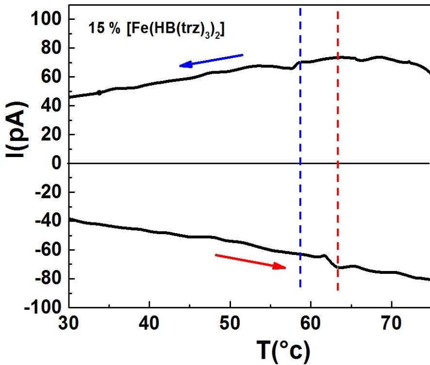
Figure S20. Pyroelectric discharge cycle for a polarized composite **5e**
