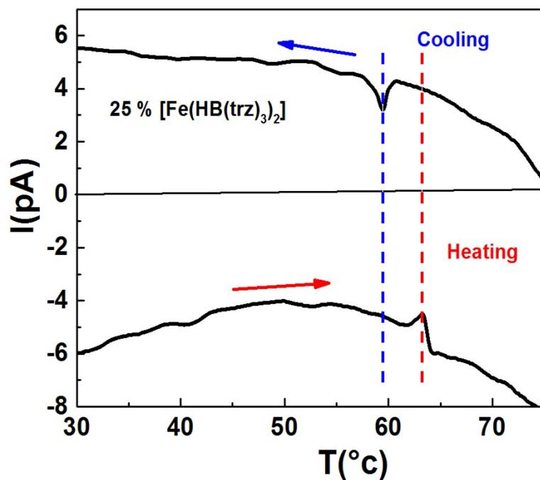
Figure S18. Pyroelectric discharge cycle for a nonpolarized Composite **5d**. Dotted lines indicate the discharge peak temperatures for cooling (left) and heating (right).
