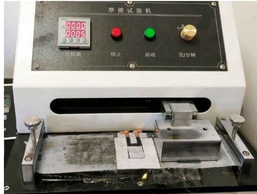
Figure S10 Photograph of the process to test leather-based e-whisker's abrasion durability.
