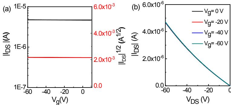
**Figure S18.** The typical transfer (a) and output characteristics (b) of **DPh-D** based devices, respectively.
