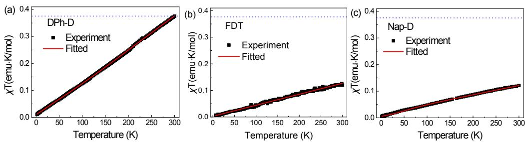
**Figure S10.** Temperature-dependent plots of  $\chi T$  for **DPh-D** (a), **FDT** (b) and **Nap-D** (c) measured at 1.0 T in the stable mode from 2 to 300 K. The solid lines are the fitting curves according to Bleaney–Bowers equation; g-factor was taken to be 2. The
