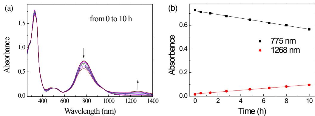
**Figure S5.** UV-Vis-NIR absorption spectra of **Nap-D** (a) in  $\text{CH}_2\text{Cl}_2$  upon irradiation with white light (400 W). The changes of the optical density at 775 and 1268 nm for **Nap-D** (b) as a function of irradiation time.
