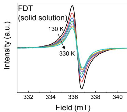
**Figure S12.** Variable temperature ESR spectra of **FDT** in benzophenone solid solution.
