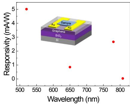
**Figure S20.** Responsivity of the photodiode fabricated from **DPh-D** at different illumination wavelength (520 nm at 6.28 mW, 650 nm at 20 mW, 780 nm at 30 mW, 808 nm at 110 mW). Inset shows the device structure of OPD was used in this study.
