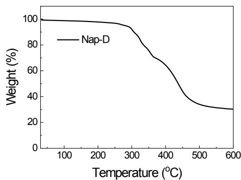
**Figure S3.** TGA of **Nap-D** under N<sub>2</sub>; heating rate = 10 °C/min.
