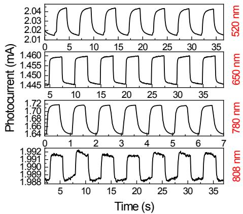
**Figure S19.** Transient photocurrent measurements of the photodiodes were fabricated from **DPh-D** upon alternative illumination with lasers at different illumination wavelength (520 nm at 6.28 mW, 650 nm at 20 mW, 780 nm at 30 mW, 808 nm at 110 mW).
