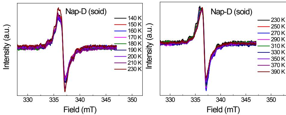
**Figure S16.** Variable temperature ESR spectra of **Nap-D** in solid state.
