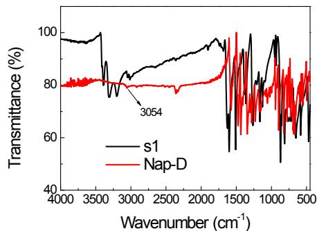
**Figure S9.** FT-IR spectra of compounds **s1** & **Nap-D**.
