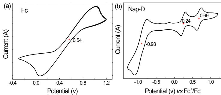
**Figure S6.** Cyclic voltammogram of ferrocene (a), **Nap-D** (b) in dry  $\text{CH}_2\text{Cl}_2$  with 0.1 M  $\text{Bu}_4\text{NPF}_6$  as supporting electrolyte, Ag/AgCl as reference electrode, glassy carbon as working electrode, Pt wire as counter electrode, and a scan rate at 100 mV/s. The red stars indicate the half-wave potential  $E_{1/2}$ .
