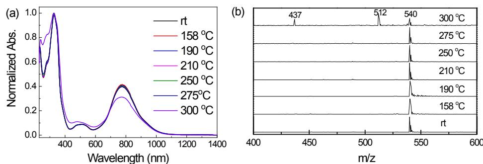
**Figure S4.** Room temperature UV-Vis-NIR absorption spectra (a) and MALDI-TOF mass spectra (b) of **Nap-D** after annealing at different temperatures under N<sub>2</sub> for 15 minutes (using TGA apparatus).
