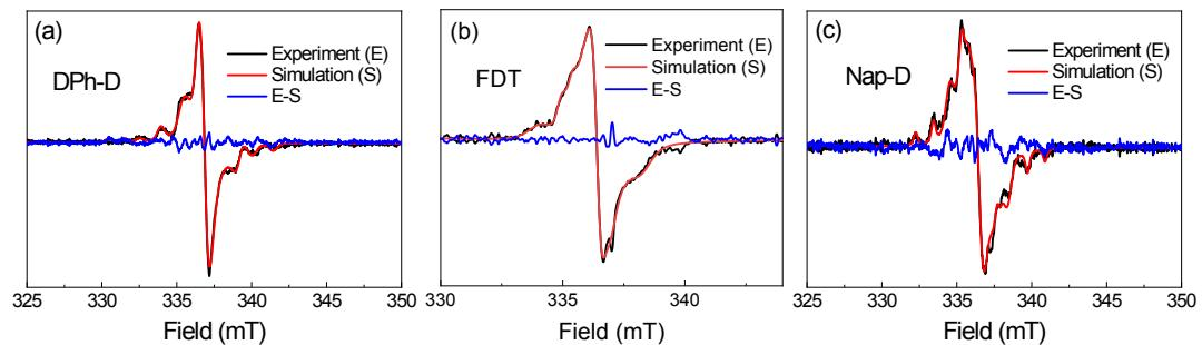
**Figure S17.** ESR spectra of **DPh-D** (a), **FDT** (b) and **Nap-D** (c) (in toluene/CHCl<sub>3</sub>, v/v = 1:1) at 130 K. The black, red and blue lines indicate experimental, simulated and difference ESR (experimental - simulated) spectra, respectively.
