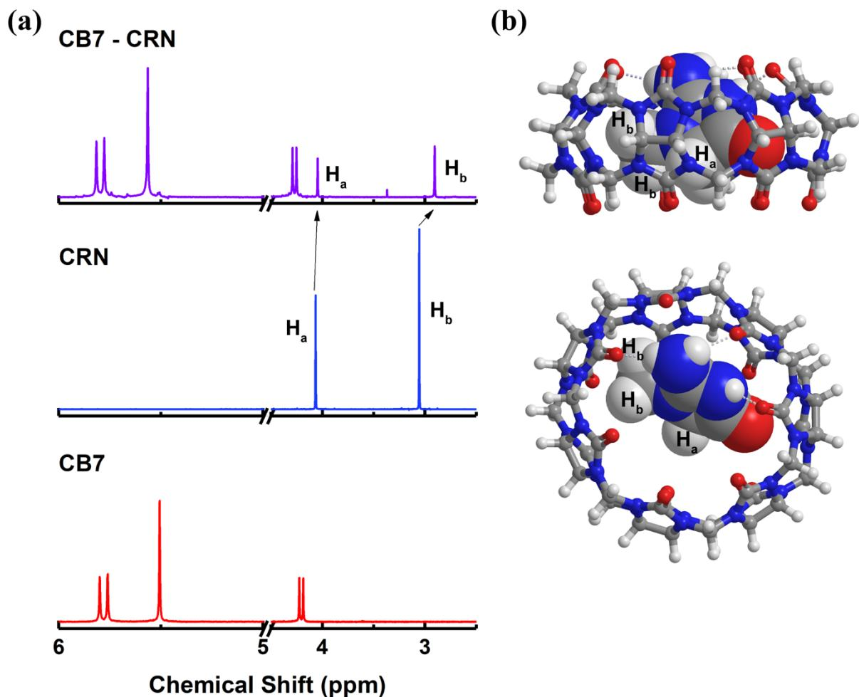
**Figure S1.** (a) <sup>1</sup>H NMR spectra of CB7, CRN and CB7-CRN inclusion complex with 1:1 stoichiometry in D<sub>2</sub>O. Characteristic upfield shifts of CRN protons were observed. (b) Side and top views of an energy-minimised [CB7-CRN-H]<sup>+</sup> inclusion complex in water modelled at CPCM/wB97XD/6-31G\* level of theory.
