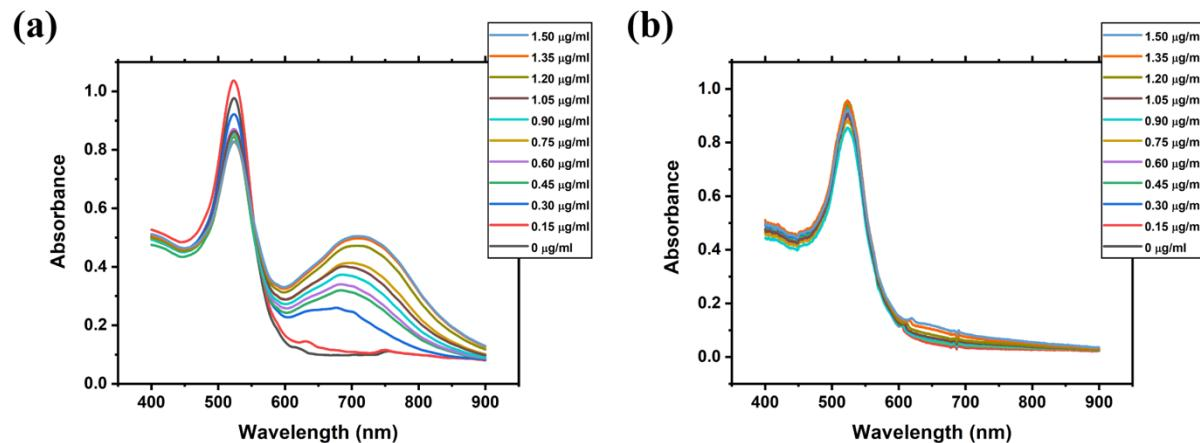
**Figure S6.** UV-Vis spectra of Au NP-CRN in (a) water and (b) SU after 2000x dilution, with CRN concentration from 0 to 1.50 µg/ml in the absence of CB7.
