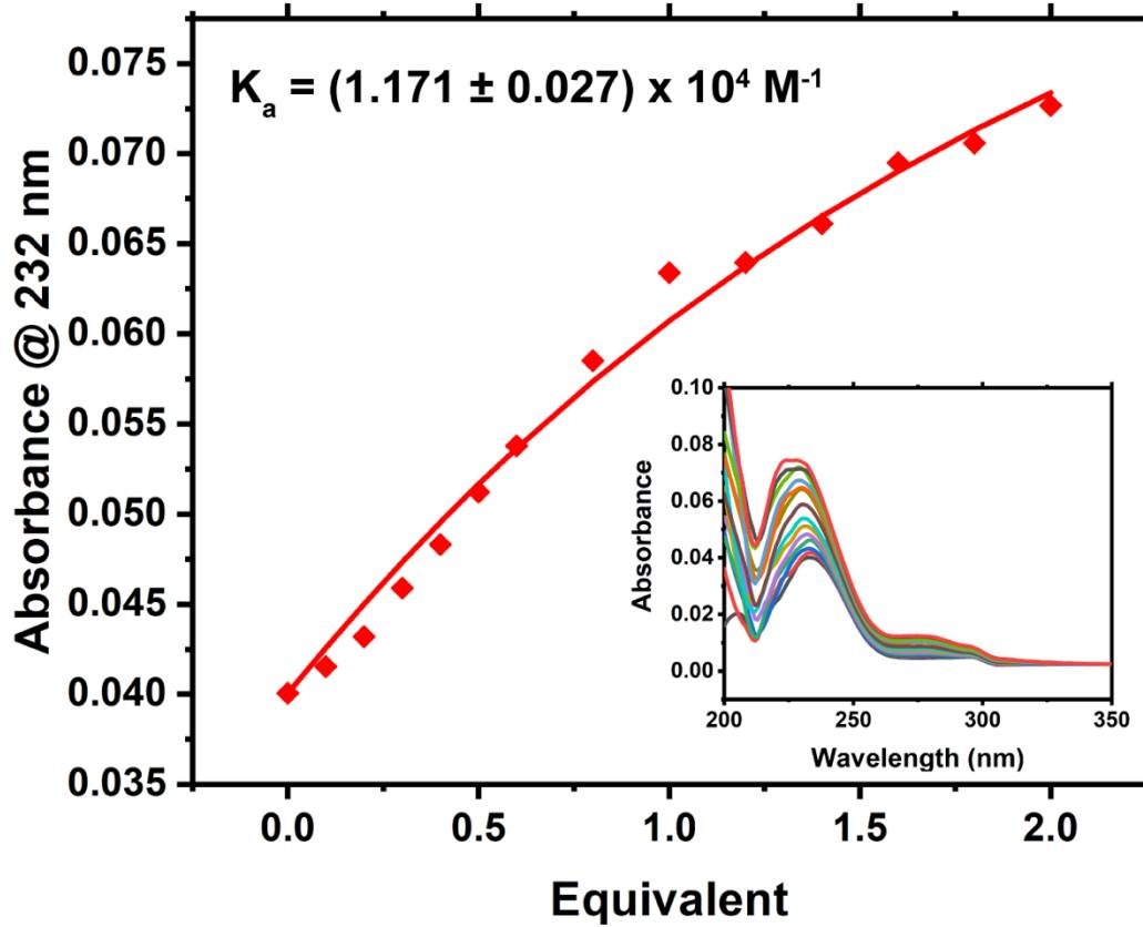
**Figure S2.** UV-Vis titration of 50  $\mu\text{M}$  CRN with up to 2 equivalents of CB7. The binding curve was fitted by assuming a 1:1 binding model from which the binding constant was derived. Inset: UV-Vis spectra of CB7-CRN with concentrations of CB7 from 0 to 100  $\mu\text{M}$ .
