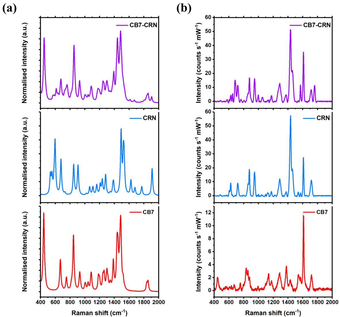
**Figure S8.** (a) Simulated Raman spectra of CB7, CRN and 1:1 CB7-CRN inclusion complex in water at CPCM/wB97XD/6-31G\* level of theory. (b) Experimental SERS spectra of CB7, CRN and CB-CRN inclusion complex with 40 nm Au NPs in water, showing general consistency with the simulated data.
