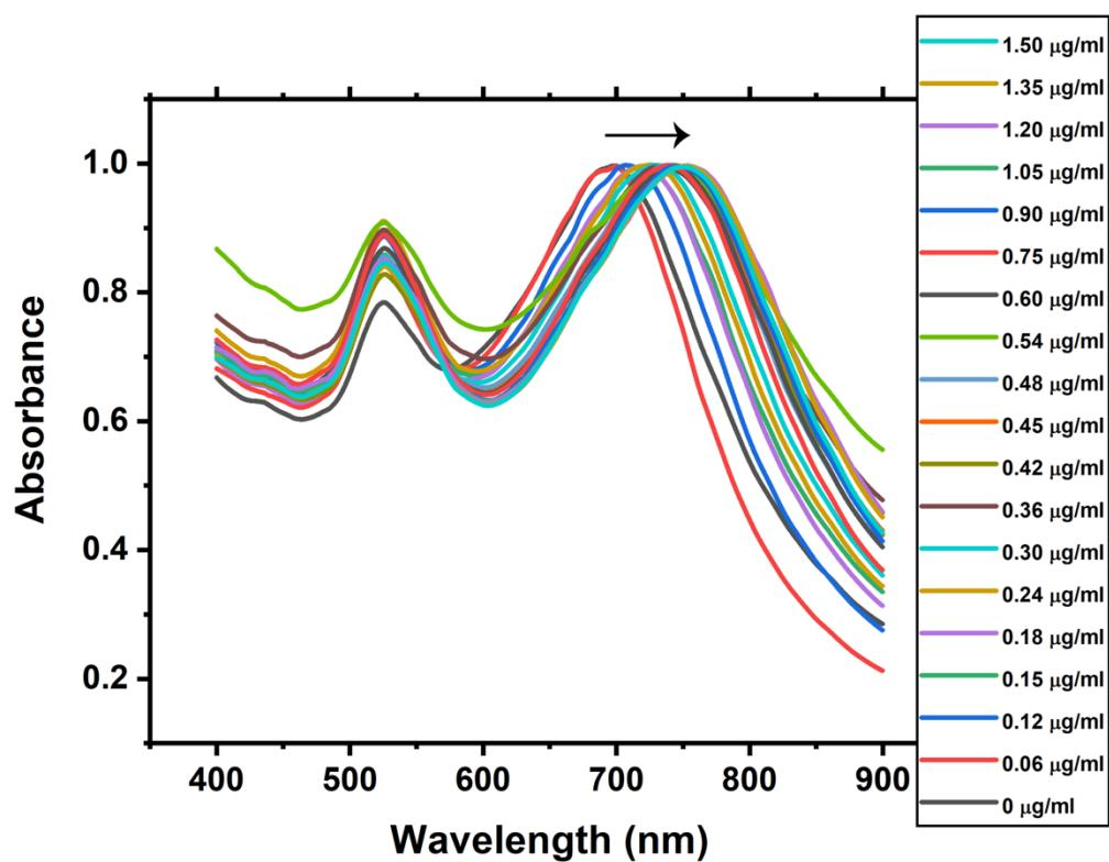
**Figure S5.** Full UV-Vis spectra of AuNP-CRN in water with CRN concentration from 0 to 1.50  $\mu\text{g/ml}$  in the presence of CB7, with an arrow indicating the shifting of the LSPR peaks.
