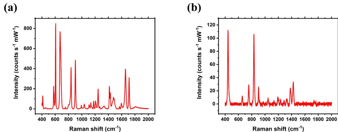
**Figure S7.** Raman spectra of (a) CRN powder and (b) CB7 powder respectively.
