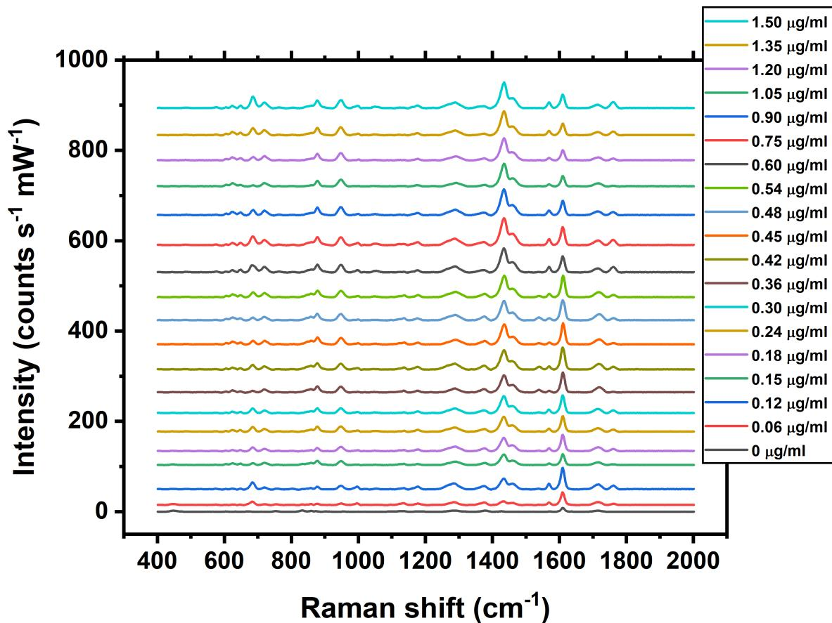
**Figure S9.** Full SERS spectra of CRN in water with concentrations from 0 to 1.50 μg/ml with aggregation of Au NPs triggered by 10 μM CB7.
