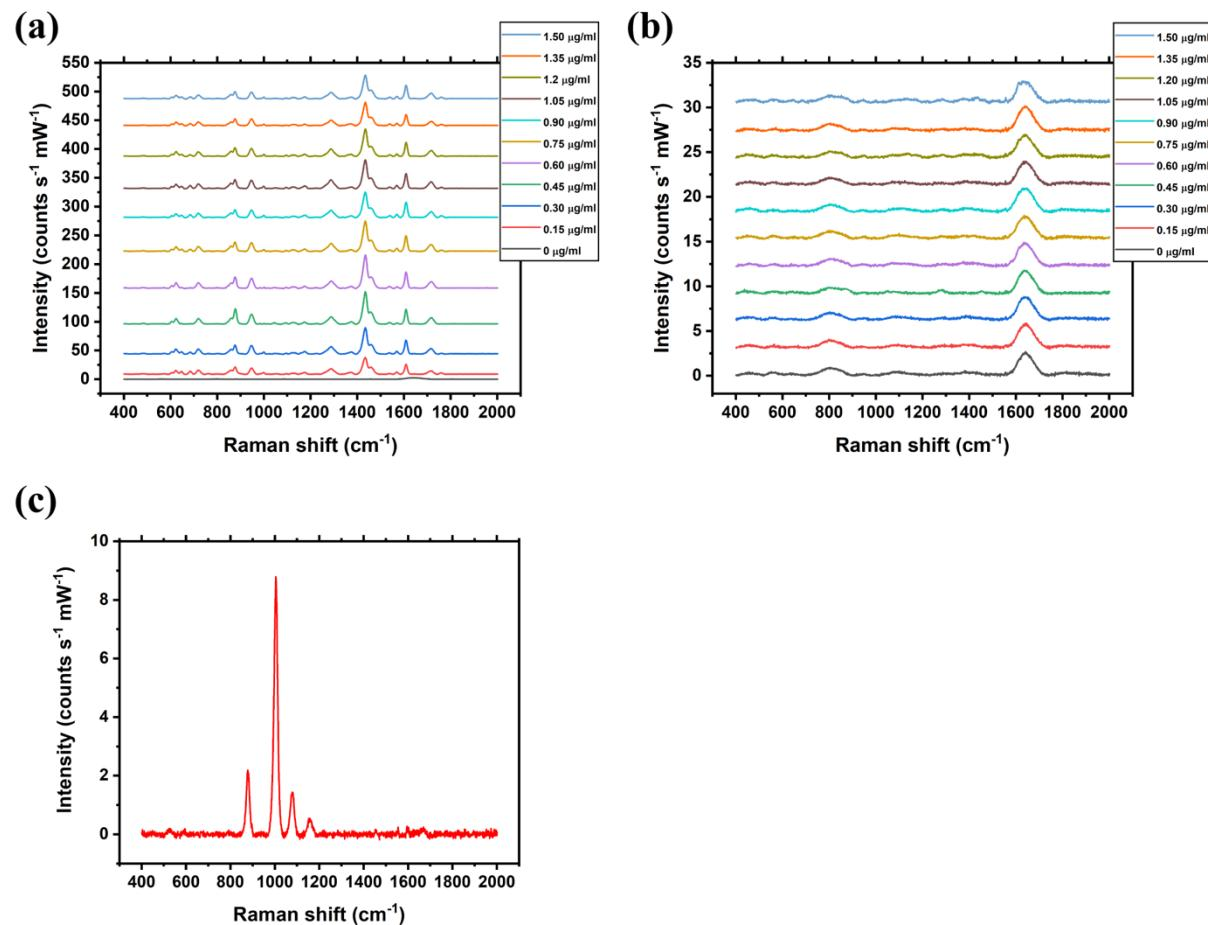
**Figure S10.** (a-b) SERS spectra of Au NP-CRN in (a) water and (b) SU after 2000x dilution, with CRN concentration from 0 to 1.50  $\mu\text{g/ml}$  in the absence of CB7. (c) Raman spectrum of SU.
