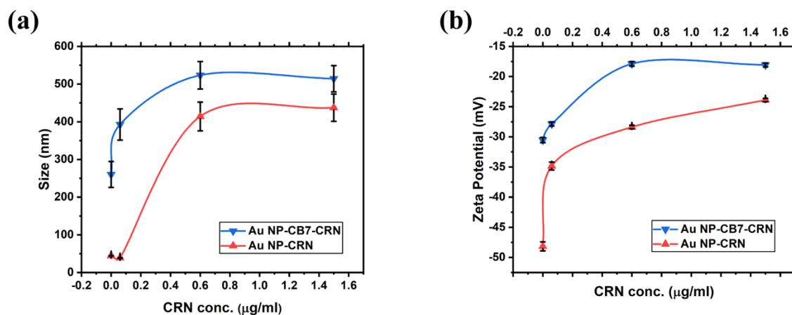
**Figure S4.** (a) Size and (b) zeta potential of Au NP-CRN and Au NP-CB7-CRN at different concentrations of CRN from 0 to 1.50  $\mu\text{g}/\text{ml}$ . (Note: solid lines are to guide the eyes.)
