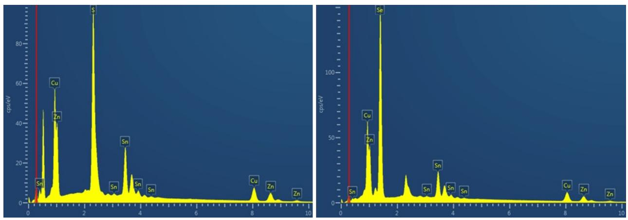
Figure S2: Surface EDX analysis (15 kV) of thin films after spin deposition (left), and after selenisation (right). The remaining peak at ~2.3 keV in the right EDX data could refer to S or Mo, but is most likely indicating Mo (See also Figure S24b).
