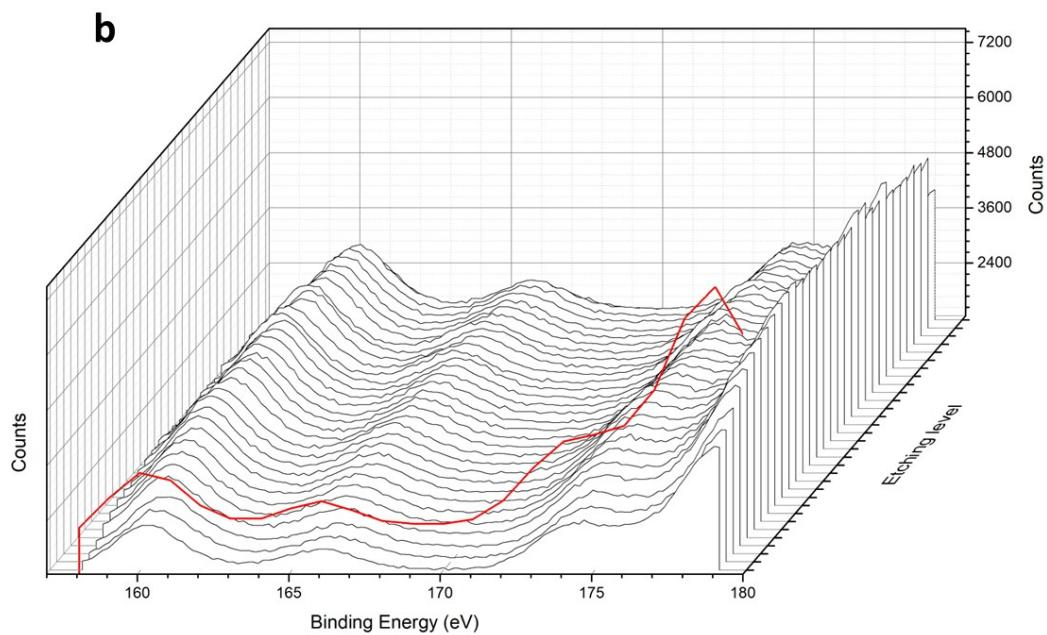
Figure S24: a) XPS analysis of a selenized CZTSe sample, Atomic % was recorded every 50 nm. b) XPS data displaying the region where peaks characteristic of S would appear, the red line is the background, the black lines are data from the sample throughout the bulk of the film. At no point is there a peak greater than the background counts, showing there is negligible levels of S in the film.
