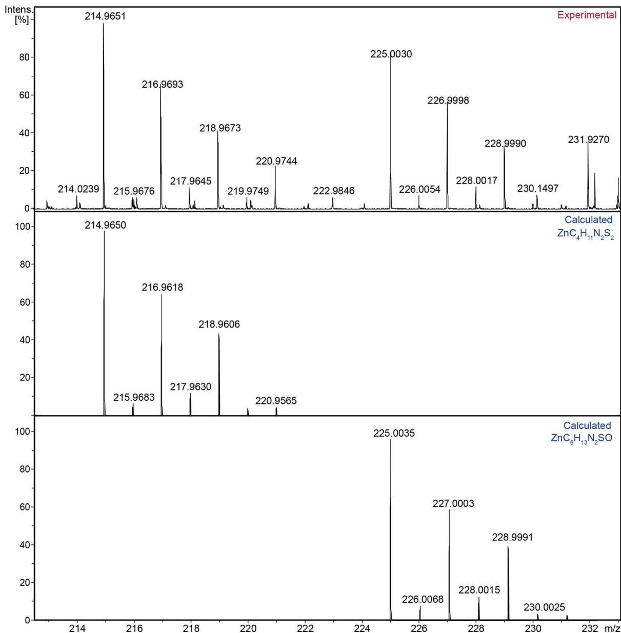
Figure S14: ESI-(+)-MS spectrum of dissolved zinc. Accurate mass for  $[M]^+$  214.9651 Da, exact mass for  $ZnC_4H_{11}N_2S_2$  214.9650 Da,  $\Delta = 0.5$  ppm; accurate mass for  $[M]^+$  225.0030 Da, exact mass for  $ZnC_6H_{13}N_2SO$  225.0035 Da,  $\Delta = 2.2$  ppm.
