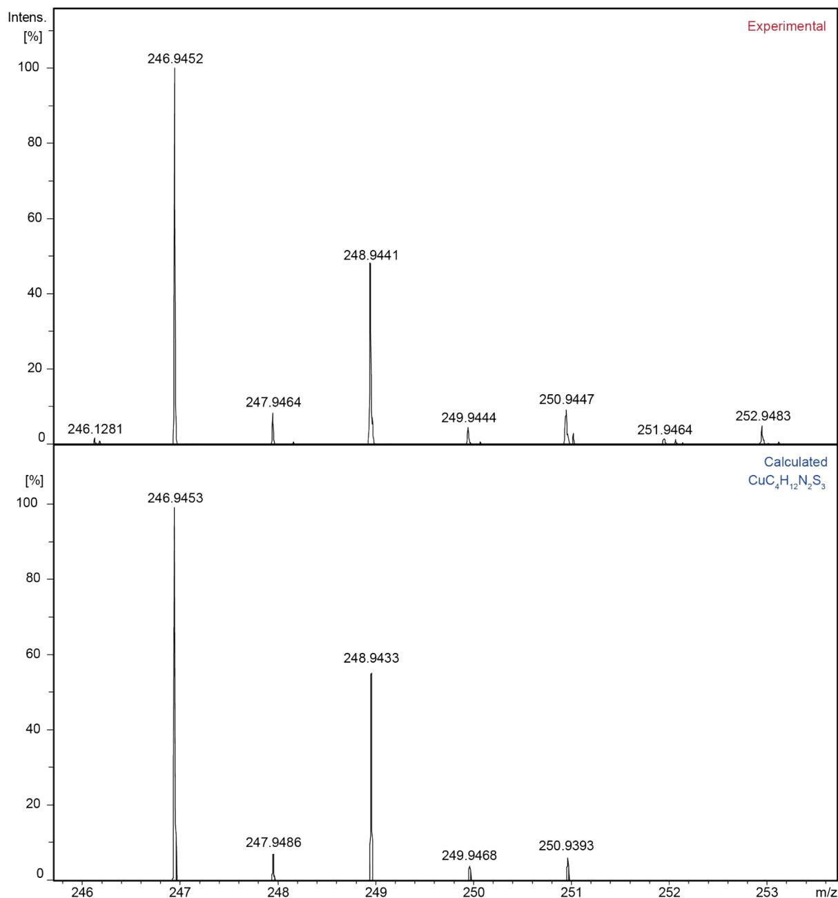
Figure S4: ESI-(+)-MS spectrum of dissolved copper, expanded to the  $\text{CuC}_4\text{H}_{12}\text{N}_2\text{S}_3$  complex. Accurate mass for  $[\text{M}]^+$  246.9452 Da, exact mass for  $\text{CuC}_4\text{H}_{12}\text{N}_2\text{S}_3$  246.9453 Da,  $\Delta = 0.4$  ppm.
