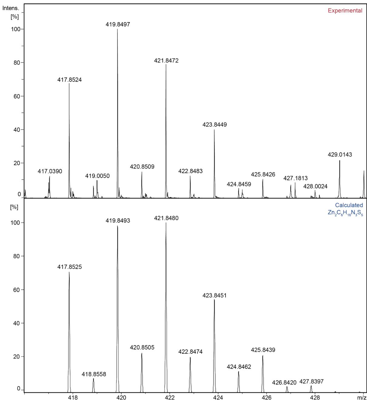
Figure S17: ESI-(+)-MS spectrum of dissolved zinc, expanded to the  $\text{Zn}_2\text{C}_6\text{H}_{16}\text{N}_3\text{S}_5$  complex. Accurate mass for  $[\text{M}]^+$  421.8472 Da, exact mass for  $\text{Zn}_2\text{C}_6\text{H}_{16}\text{N}_3\text{S}_5$  421.8480 Da,  $\Delta = 1.9$  ppm.
