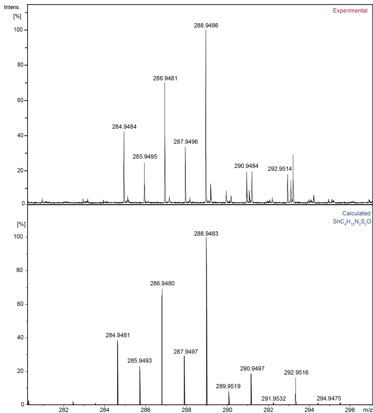
Figure S10: ESI-(+)MS spectrum of dissolved tin, expanded to the  $\text{SnC}_4\text{H}_{13}\text{N}_2\text{S}_2\text{O}$  complex. Accurate mass for  $[\text{M}]^+$  288.9486 Da, exact mass for  $\text{SnC}_4\text{H}_{13}\text{N}_2\text{S}_2\text{O}$  288.9483 Da,  $\Delta = 1 \text{ ppm}$ .
