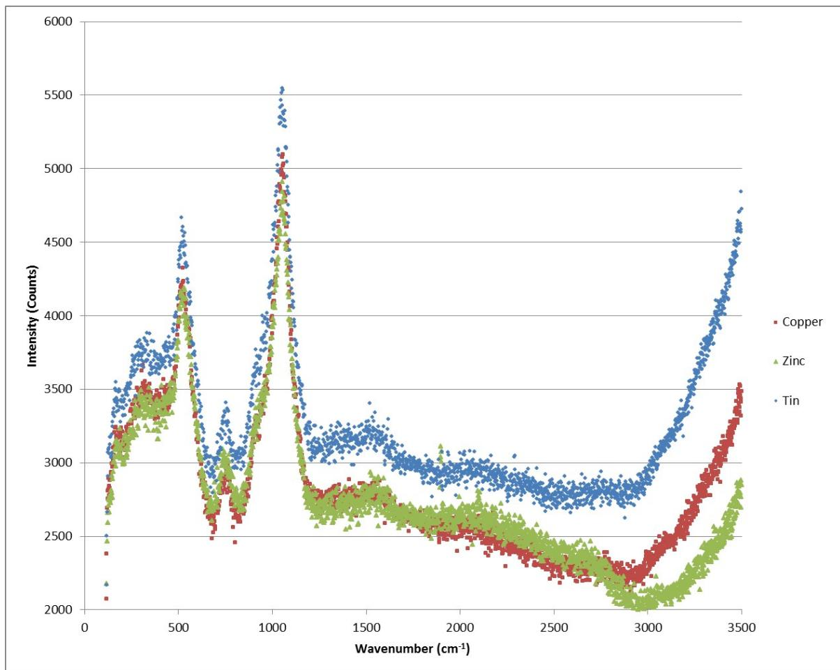
Figure S1: Raman spectroscopy data for three ethanolamine/cysteamine solutions containing one of the metals (Cu, Zn, and Sn).
