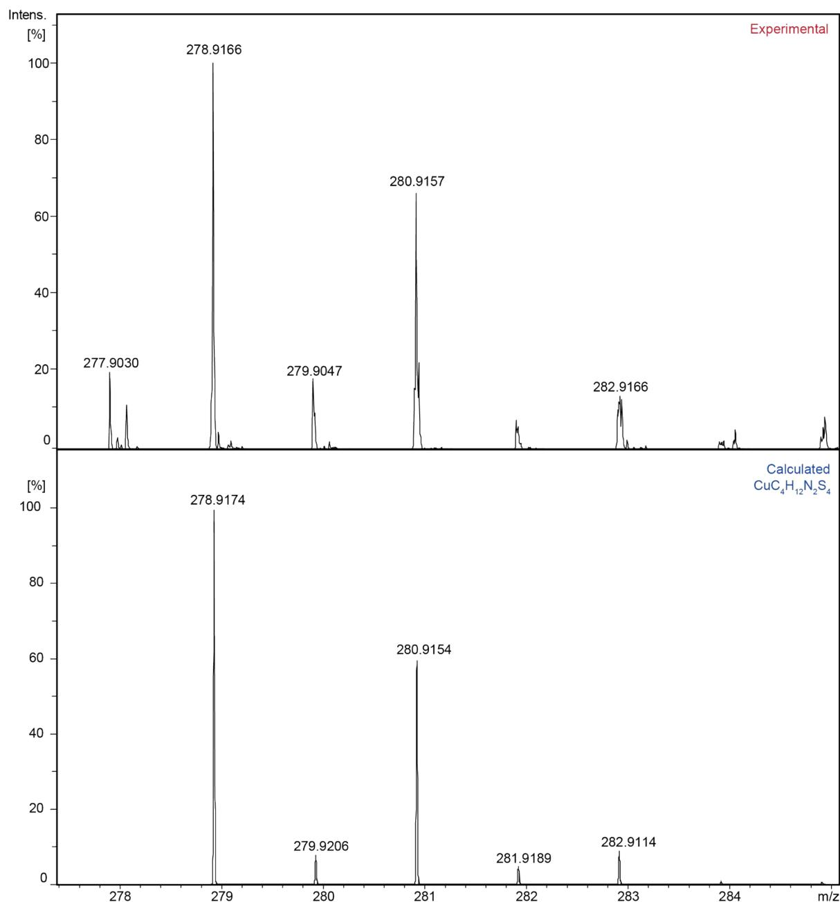
Figure S5: ESI-(+)-MS spectrum of dissolved copper, expanded to the  $\text{CuC}_4\text{H}_{12}\text{N}_2\text{S}_4$  complex. Accurate mass for  $[\text{M}]^+$  278.9166 Da, exact mass for  $\text{CuC}_4\text{H}_{12}\text{N}_2\text{S}_4$  278.9174 Da,  $\Delta = 2.9$  ppm.
