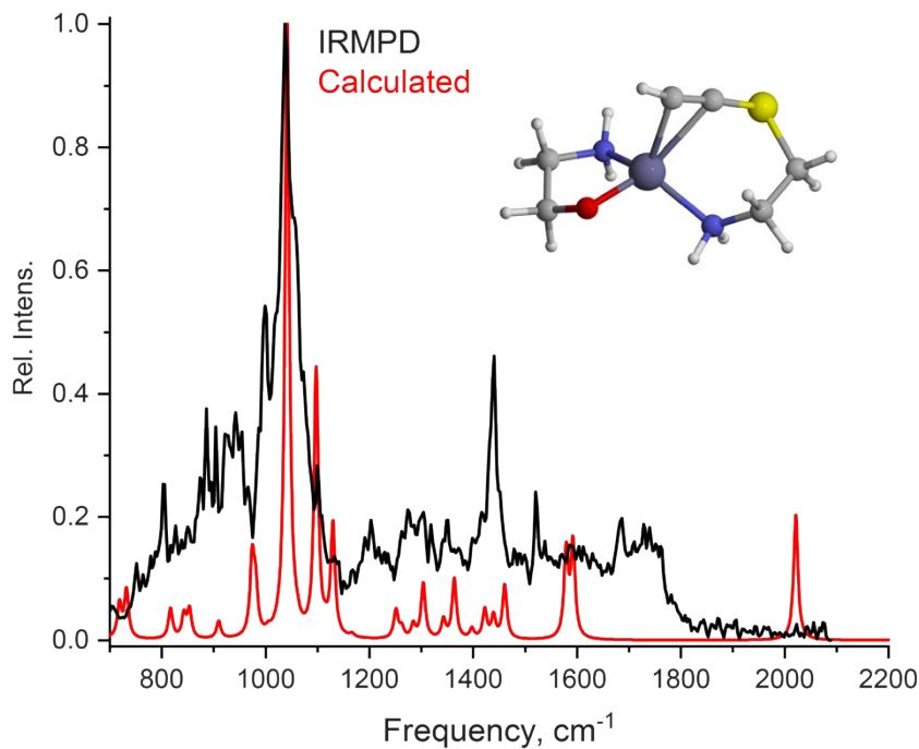
Figure S21: Alternative zinc/acetylene complex  $\text{Zn}(\mathbf{1})(\mathbf{2})\text{C}_2\text{H}$  with  $m/z$  225.0035 observed in ESI-MS: Structure of the complex optimised by DFT calculations; experimental IRMPD and calculated spectrum (both normalized) of this ion.
