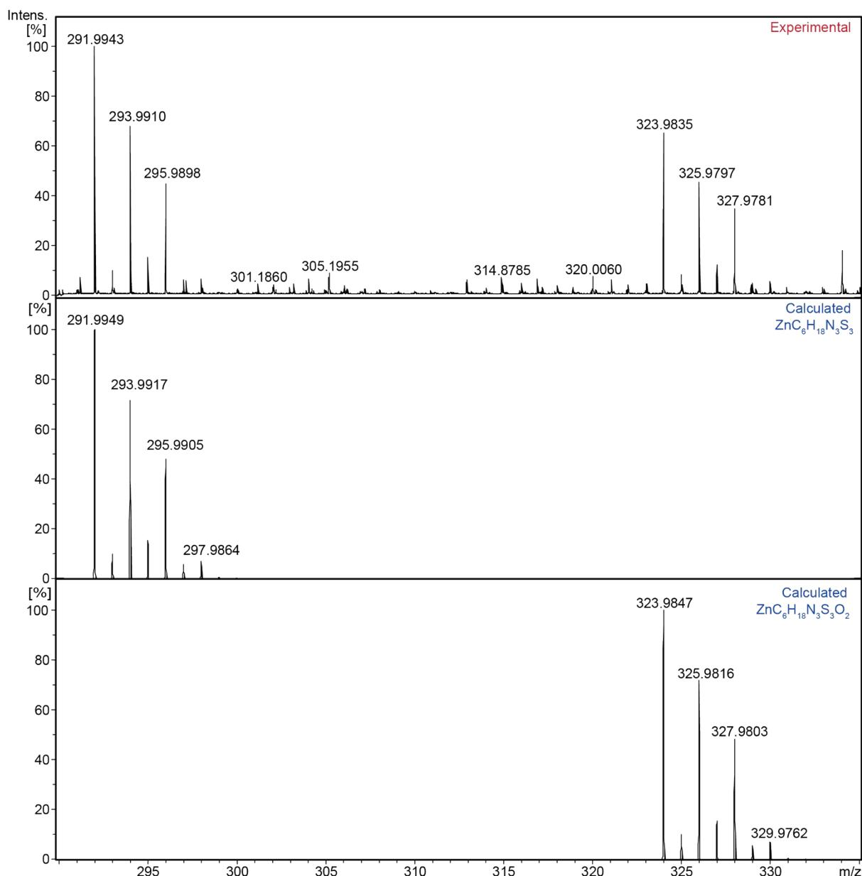
Figure S15: ESI-(+)-MS spectrum of dissolved zinc. Accurate mass for  $[M]^+$  291.9943 Da, exact mass for  $ZnC_6H_{18}N_3S_3$  291.9949 Da,  $\Delta = 2.0$  ppm; accurate mass for  $[M]^+$  323.9835 Da, exact mass for  $ZnC_6H_{18}N_3S_3O_2$  323.9847 Da,  $\Delta = 3.7$  ppm.
