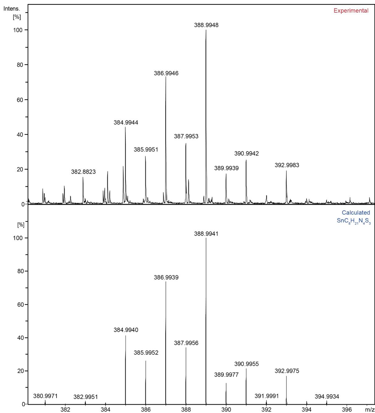
Figure S12: ESI-(+)-MS spectrum of dissolved tin, expanded to the  $\text{SnC}_8\text{H}_{21}\text{N}_4\text{S}_3$  complex. Accurate mass for  $[\text{M}]^+$  388.9948 Da, exact mass for  $\text{SnC}_8\text{H}_{21}\text{N}_4\text{S}_3$  388.9941 Da,  $\Delta = 1.8$  ppm. Low signal-to-noise ratio was observed for these ion signals, which suggests only plausible identification of the complex; however, in spite of low intensity isotopic pattern and accurate mass match reliably.
