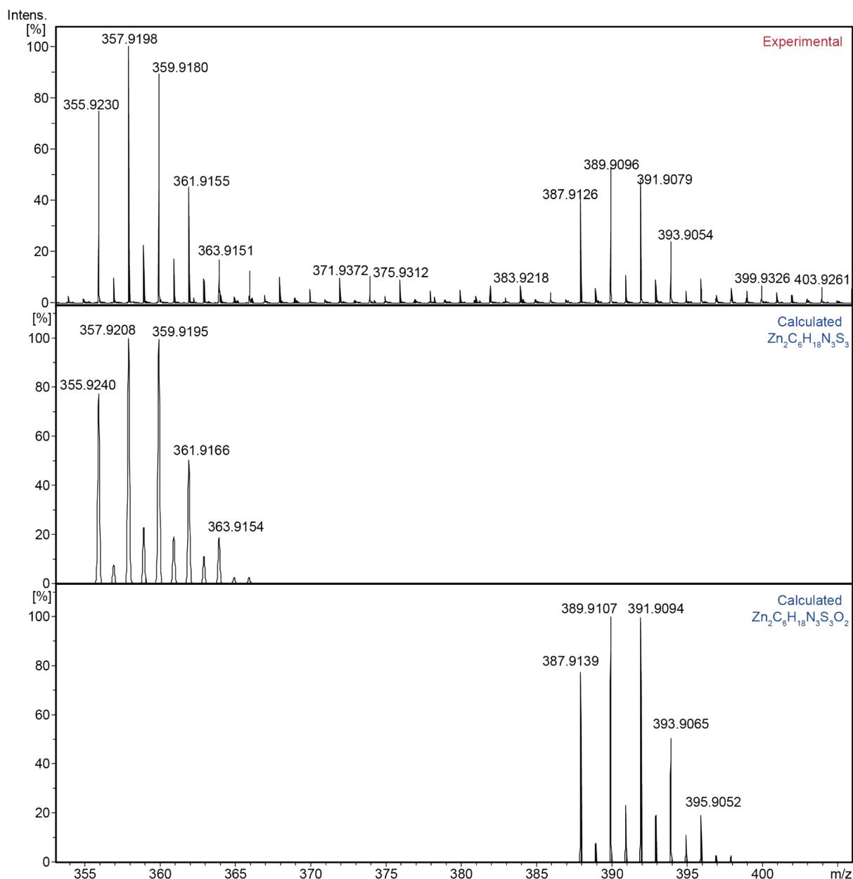
Figure S16: ESI-(+)-MS spectrum of dissolved zinc. Accurate mass for  $[M]^+$  357.9198 Da, exact mass for  $Zn_2C_6H_{18}N_3S_3$  357.9208 Da,  $\Delta = 2.8$  ppm; accurate mass for  $[M]^+$  389.9096 Da, exact mass for  $Zn_2C_6H_{18}N_3S_3O_2$  389.9107 Da,  $\Delta = 2.8$  ppm.
