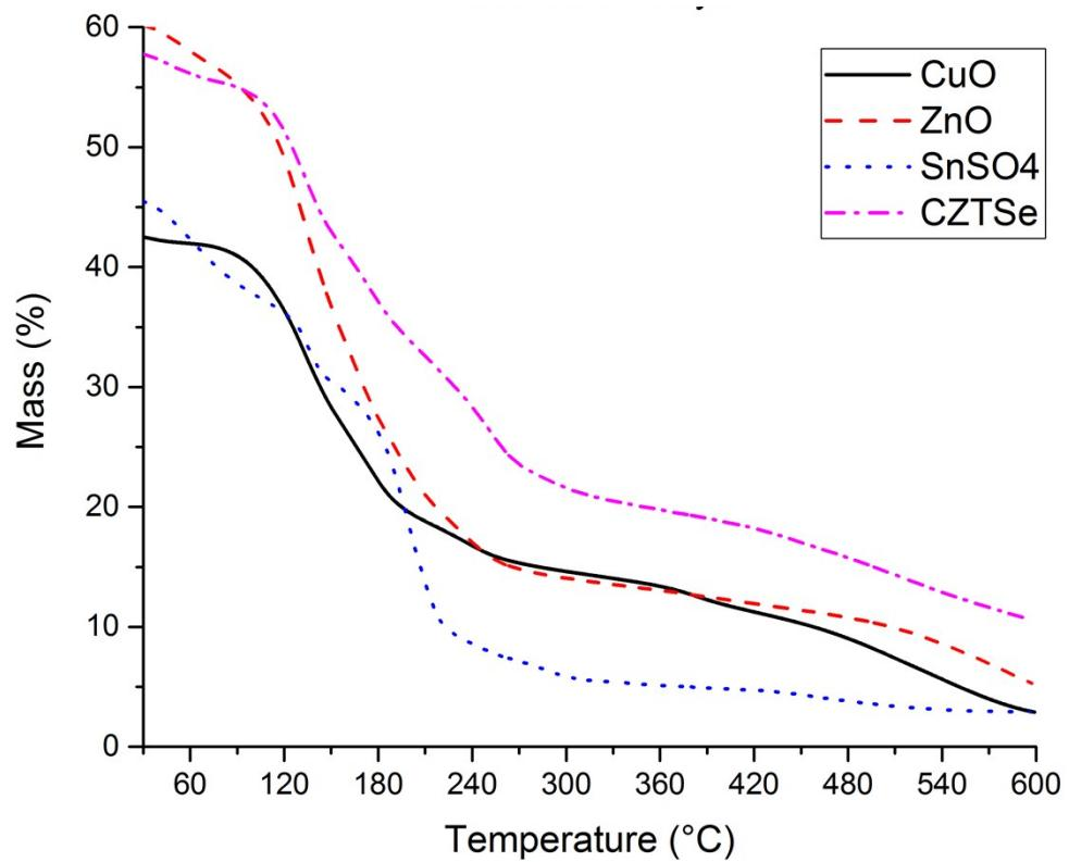
Figure S23: Thermogravimetric analysis of water based solution: Water, cysteamine, thiourea, copper (II) oxide, zinc oxide, tin (II) sulphate.
