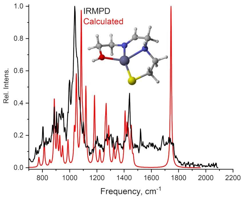
Figure S20: Alternative zinc imine complex  $\text{Zn}(\text{HOC}_2\text{H}_4\text{NHC}_2\text{H}_2\text{NHC}_2\text{H}_4\text{S})$  with  $m/z$  225.0035 observed in ESI-MS: Structure of the complex optimised by DFT calculations; experimental IRMPD and calculated spectrum (both normalized) of this ion.
