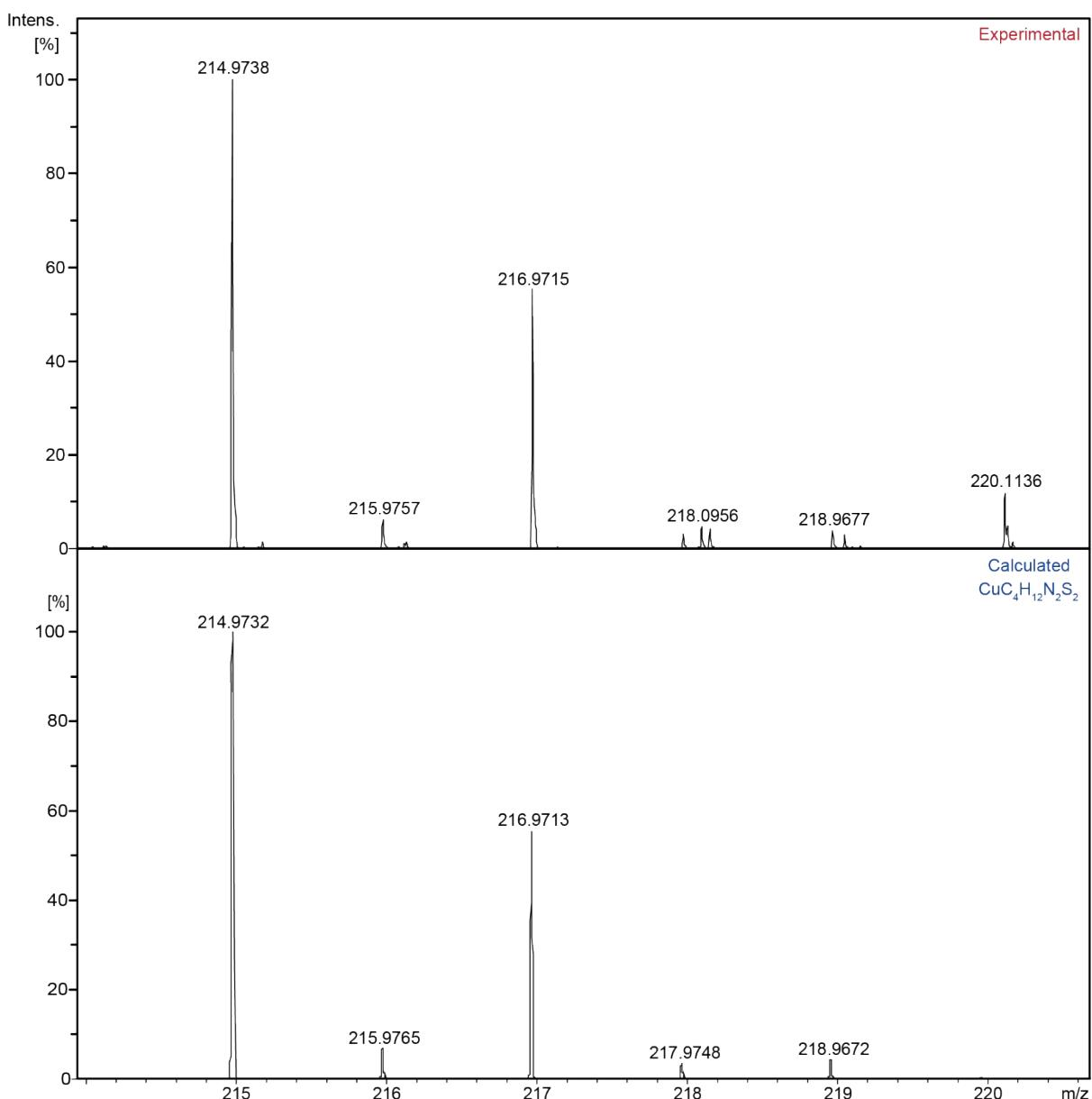
Figure S3: ESI-(+)-MS spectrum of dissolved copper, expanded to the  $\text{CuC}_4\text{H}_{12}\text{N}_2\text{S}_2$  complex. Accurate mass for  $[\text{M}]^+$  214.9738 Da, exact mass for  $\text{CuC}_4\text{H}_{12}\text{N}_2\text{S}_2$  214.9732 Da,  $\Delta = 2.8$  ppm.
