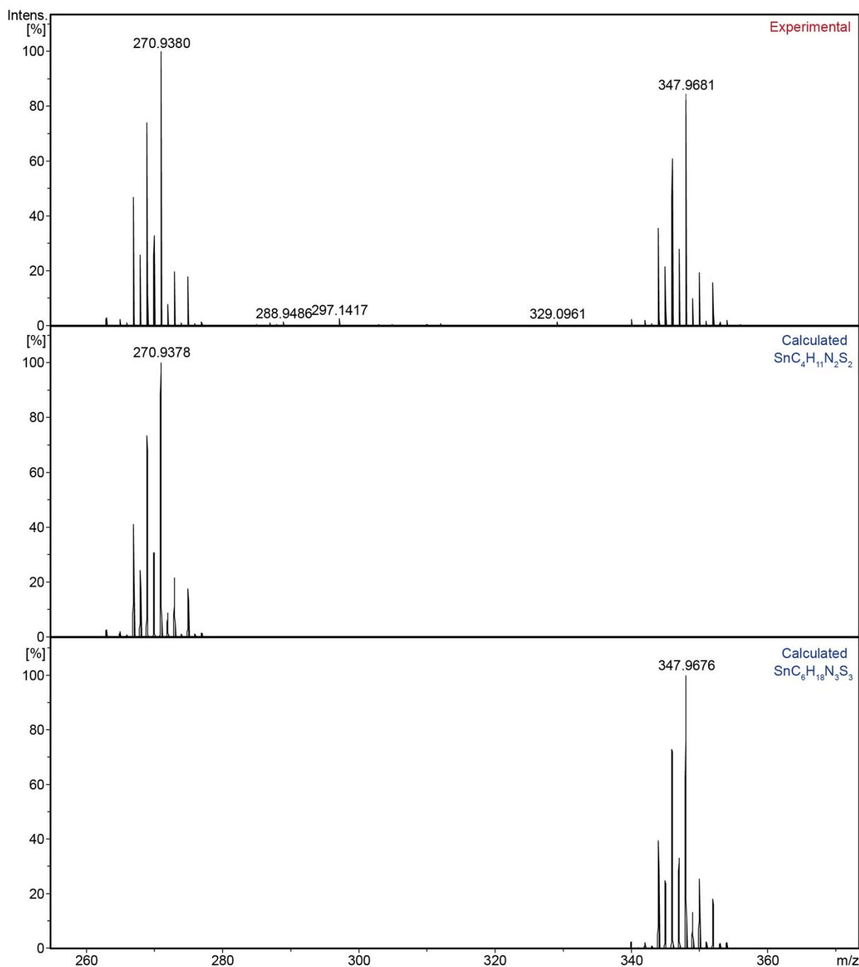
Figure S9: ESI-(+)-MS spectrum of dissolved tin. Accurate mass for  $[\text{M}]^+$  270.9380 Da, exact mass for  $\text{SnC}_4\text{H}_{11}\text{N}_2\text{S}_2$  270.9378 Da,  $\Delta = 0.7$  ppm; accurate mass for  $[\text{M}]^+$  347.9681 Da, exact mass for  $\text{SnC}_6\text{H}_{18}\text{N}_3\text{S}_3$  347.9676 Da,  $\Delta = 1.4$  ppm.
