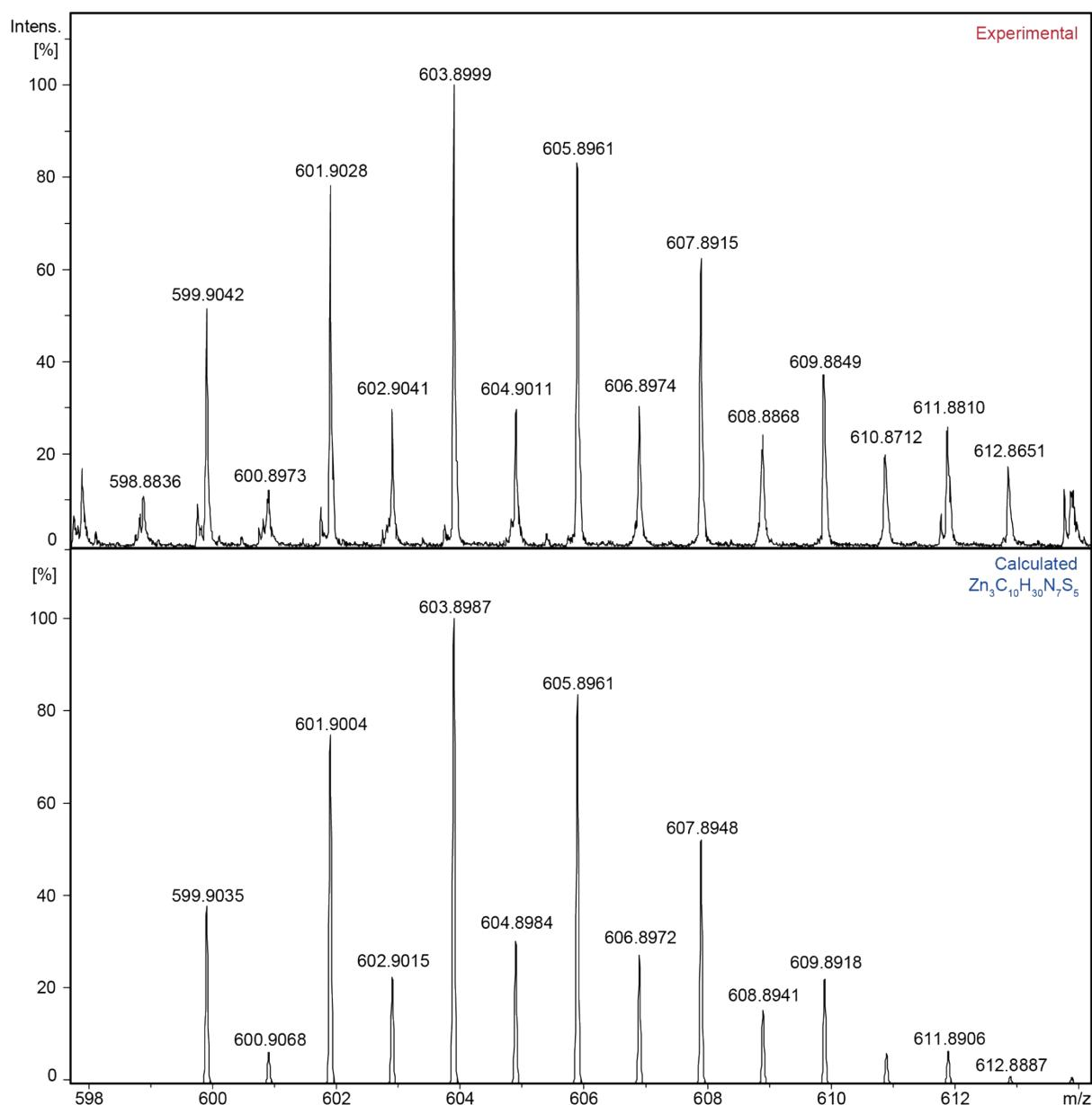
Figure S18: ESI-(+)-MS spectrum of dissolved zinc, expanded to the  $Zn_3C_{10}H_{30}N_7S_5$  complex. Accurate mass for  $[M]^+$  603.8999 Da, exact mass for  $Zn_3C_{10}H_{30}N_7S_5$  603.8987 Da,  $\Delta = 2$  ppm. Low signal-to-noise ratio was observed for these ion signals, which suggests only plausible identification of the complex; however, in spite of low intensity, the isotopic pattern and accurate mass match reliably.
