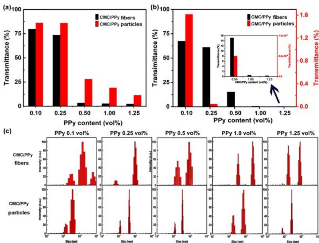
**Fig. S4** Transmittances of CMC/PPy fibers and CMC/PPy particles after processed with KPS at (a) 660 nm and (b) 365 nm; (c) DLS of CMC/PPy fibers and CMC/PPy particles with the various PPy contents
