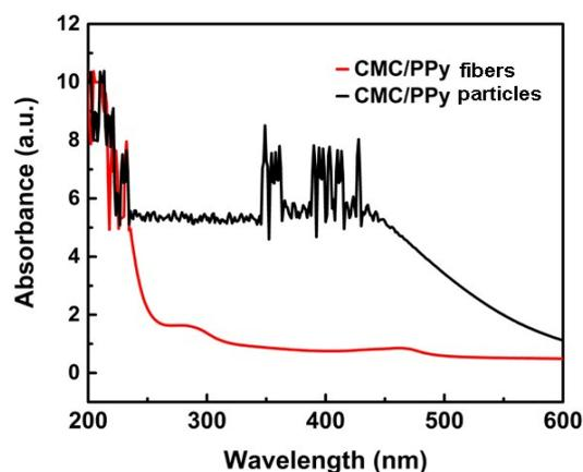
**Fig. S1** The UV-Vis absorption spectra of CMC/PPy fibers and uniformly distributed CMC/PPy particles after processed with KPS.
