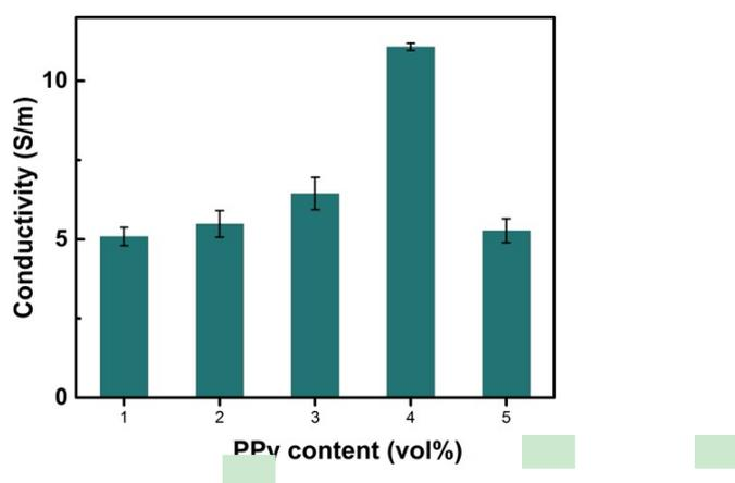
**Fig. S6** The electrical conductivity of hydrogel with various PPy contents.
