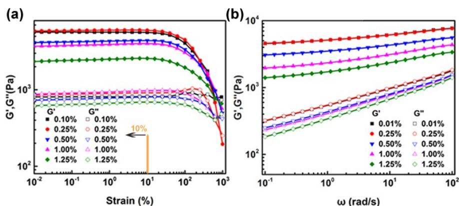
**Fig. S5** The a) amplitude sweep and b) frequency sweep curves of PAAm/CMC/PPy hydrogel with various PPy contents.
