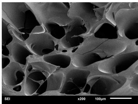
**Fig. S3** The SEM photography of dehydrated PAAm/CMC/PPy hydrogel.
