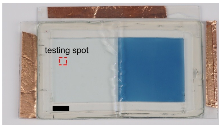
Figure S4 An optical photograph of the shoulder-by-shoulder device after being cycled for 15,000 processes, where the red dashed square denoted the in situ monitored spot of the film transmittance during life cycling as shown in Figure 3 c in the manuscript. Scale bar, 1 cm.
