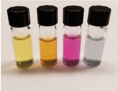
Image S1: Alumina colloid supported AgNP photoproducts. From left to right: Initial seeds, 455 nm, 525 nm and 625 nm products.
