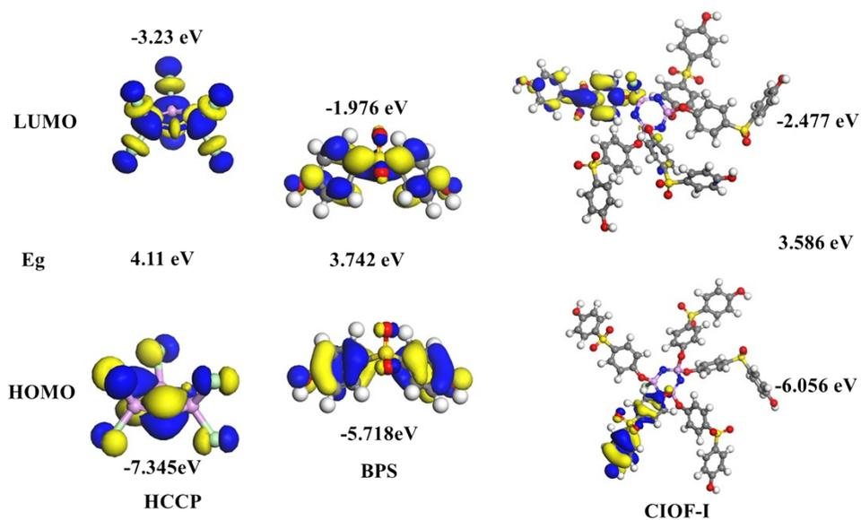
**Fig. S2.** Optimized structure for HCCP, BPS, and ClO-F-I along with their frontier electron densities and their potentials calculated by using GGA/PBE/DNP 4.4 basis set on DMoL<sup>3</sup> DFT package in Materials Studio.
