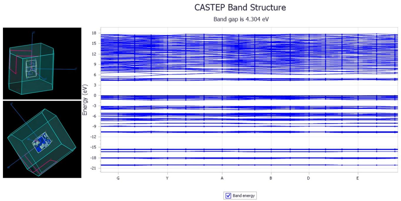
**Fig. S6.** The optimized crystal structure for TATA (obtained from PubChem database) with electron densities and their band structure calculated by using the CASTEP Plane Wave DFT package in Materials Studio.
