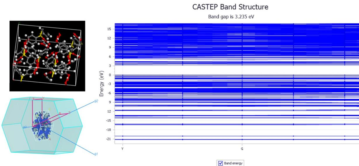
**Fig. S5.** The optimized crystal structure for BPS (obtained from PubChem database) with electron densities and their band structure calculated by using the CASTEP Plane Wave DFT package in Materials Studio.
