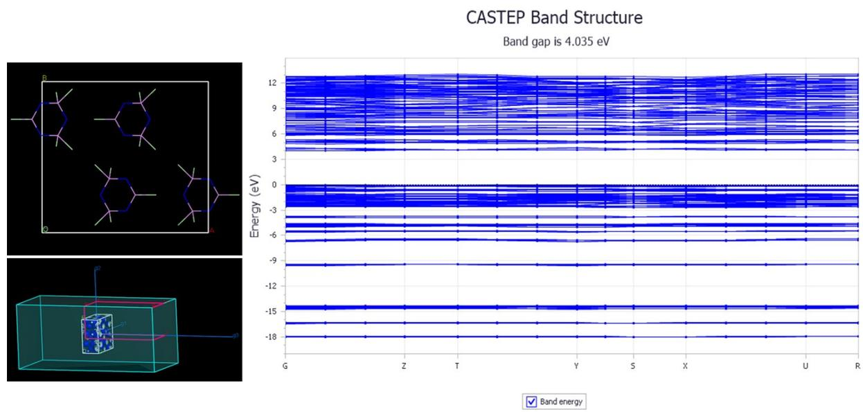
**Fig. S4.** The optimized crystal structure for HCCP (obtained from PubChem database ) with electron densities and their band structure calculated by using the CASTEP Plane Wave DFT package in Materials Studio.
