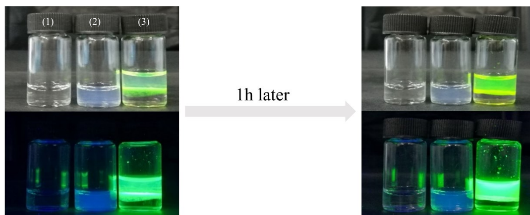
Figure S1. Photographs showing the transformation process of \text{Cs}_4\text{PbBr}_6 NCs to \text{CsPbBr}_3 NCs. The samples were illuminated with natural light (top) and UV 365nm irradiation (bottom). (1) Water, (2) \text{Cs}_4\text{PbBr}_6 nanocrystals dispersed in octane. (3) Solution with injecting \text{Cs}_4\text{PbBr}_6 nanocrystals into water
