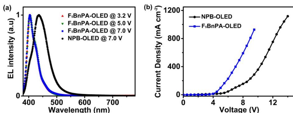
**Fig. S2** (a) the EL spectra and (c) the current density-voltage (J-V) characteristics of  $F_5BPA$ -OLED and NPB-OLED.
