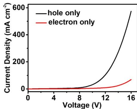
**Fig. S3** The current density-voltage (J-V) characteristics of hole-only device and electron-only device with the configuration of ITO/NPB(15 nm)/F-2CzB(30 nm)/NPB(15 nm)/Al(100 nm) (**hole-only device**) and ITO/TPBi(15 nm)/F-2CzB(30 nm)/TPBi(15 nm)/LiF(1 nm)/Al(100 nm) (**electron-only device**)
