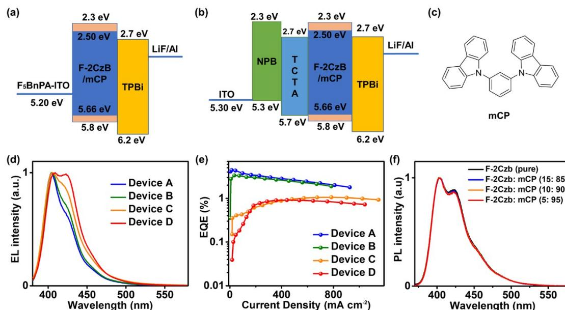
**Fig. S5** Device schematic and energy band diagram of (a) Device B and (b) Device D. (c) Molecular structure of mCP. (d) EL spectra at 10 mA cm<sup>-2</sup> and (e) EQE-current density characteristics of the devices. (f) PL spectra of pure F-2CzB film and doped film of F-2CzB: mCP (5, 10 and 15 wt%, 30 nm).
