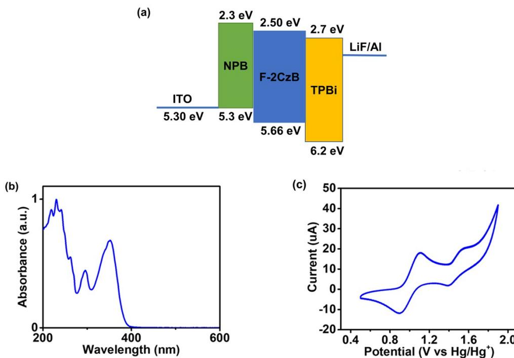
**Fig. S1** (a) Device schematic and energy band diagram of NPB-OLED. (b) UV-vis absorption spectrum and (c) cyclic voltammetry curve of F-2CzB.
