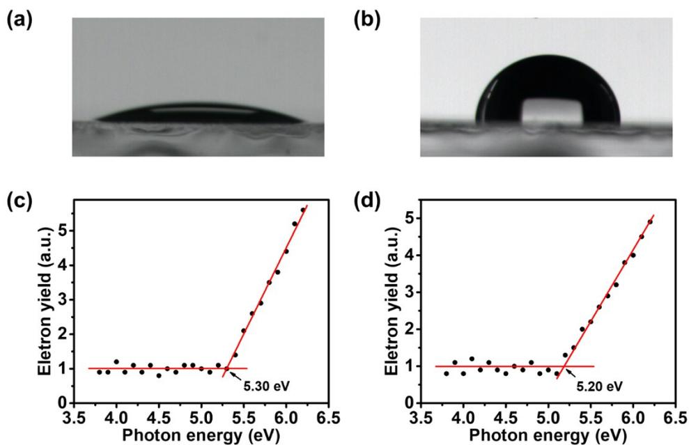
**Fig. S4** Photographs of water contact angle for (a) ITO treated with oxygen plasma and (b) F<sub>5</sub>BnPA-ITO. The work function of (c) ITO treated with oxygen plasma and (d) F<sub>5</sub>BnPA-ITO.
