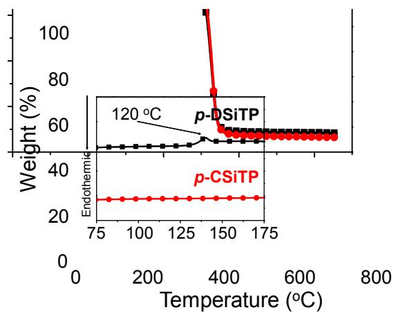
**Fig. S1** TGA traces of *p*-DSiTP and *p*-CSiTP recorded at heating rate of 20 °C min<sup>-1</sup> under N<sub>2</sub>. Inset: DSC traces of *p*-DSiTP and *p*-CSiTP recorded at heating rate of 10 °C min<sup>-1</sup> under N<sub>2</sub>.
