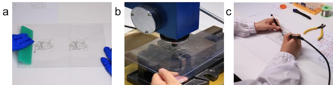
Figure S9. The fabrication process of the double-sided circuit board by the solidified circuit printing method with low-melting metal. (a) Circuit board aligning and bonding. (b) Circuit board punching. (c) Low-temperature welding of the via holes.
