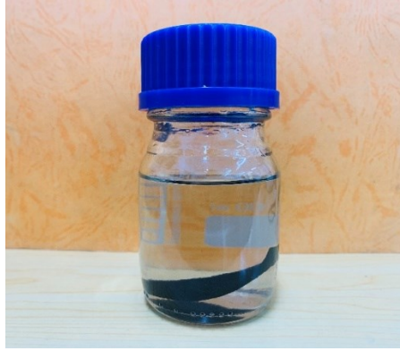
Fig. S4 Image of the acetone etchant after soaking the TPU/PCL/MWCNT blending composite for 24 h.
