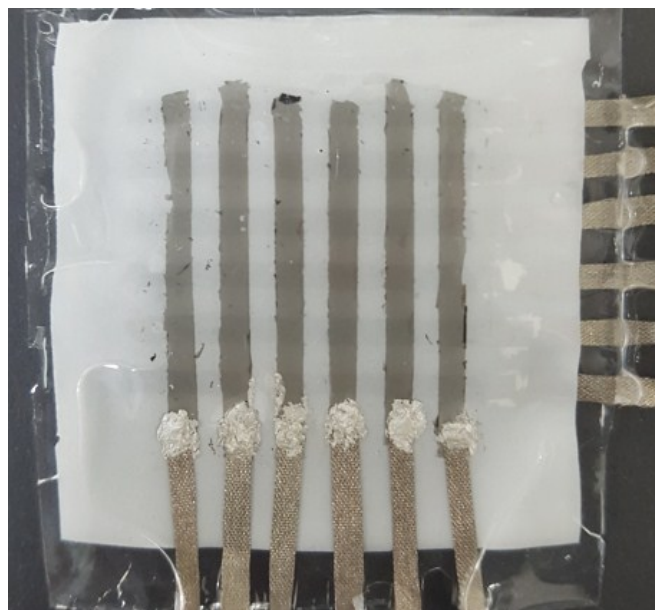
Figure S11: 6 × 6 pixelated ACEL device at off state.
