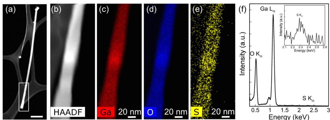
**Figure S4.** EDS elemental maps of single crystalline  $\text{Ga}_2\text{O}_3$  nanowires. (a) HAADF-STEM image of representative  $\text{Ga}_2\text{O}_3$  nanowires (scale bar: 200 nm). (c) - (e) EDS elemental maps of one of the  $\text{Ga}_2\text{O}_3$  nanowires showing the distribution of Ga (red), oxygen (blue) and sulfur (yellow). (f) EDS spectrum from the nanowire. The inset shows the magnified sulfur  $\text{K}_\alpha$  region of the spectrum.
