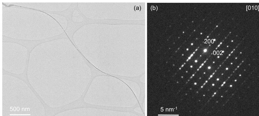
**Figure S2. Morphology of single crystalline  $\text{Ga}_2\text{O}_3$  nanowires grown on  $\text{SiO}_2/\text{Si}$  (100) substrate covered with nominally 2 nm Ag film. (a) Overview TEM image of a typical  $\text{Ga}_2\text{O}_3$  nanowire on amorphous carbon film (growth temperature:  $550^\circ\text{C}$ ). (b) Electron diffraction pattern of the  $\text{Ga}_2\text{O}_3$  nanowire along the [010] zone axis.**
