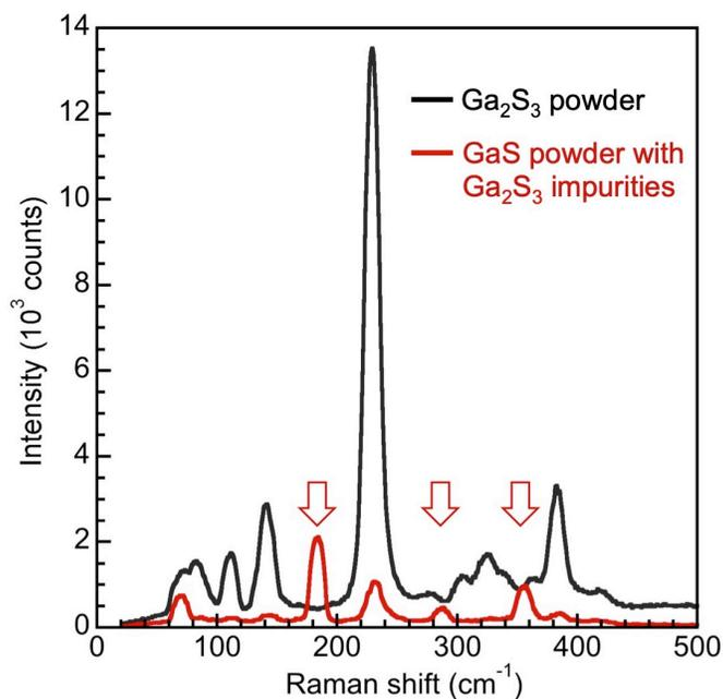
**Figure S3. Raman spectrum of the  $\text{Ga}_2\text{S}_3$  precursor powder.** The observed modes (black curve) are consistent with pure  $\text{Ga}_2\text{S}_3$ , see ref. 1. Comparison with the spectrum of a GaS powder containing a small amount of  $\text{Ga}_2\text{S}_3$  impurities (red curve) shows no detectable GaS in our  $\text{Ga}_2\text{S}_3$  precursor (absence of GaS peaks marked by red arrows).
