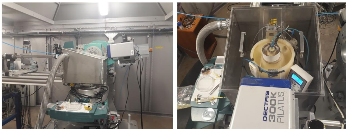
Figure S1: Photographs of the setup at XRD2/LNLS beamline for in situ GIWAXS measurements.
