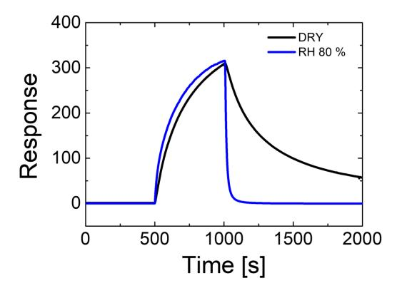
Figure S3. Variation in the response of the  $SnS_2$  sensor towards 1 ppm NO<sub>2</sub> gas in atmosphere with relative humidity of 0 and 80 %, respectively.
