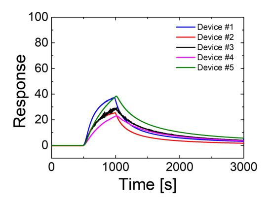
Figure S1. Variation in the response of five different  $SnS_2$  gas sensors towards 100 ppb  $NO_2$  at room temperature.
