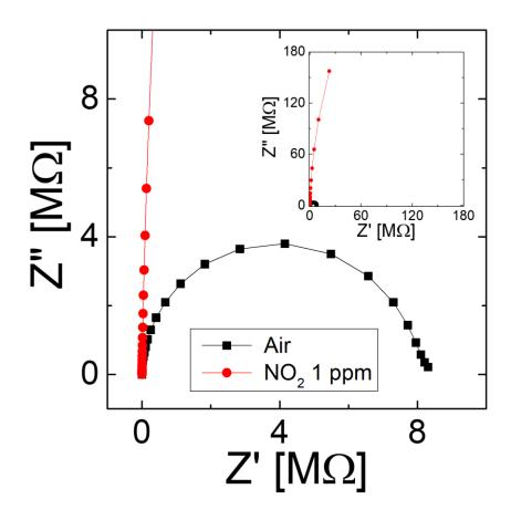
Figure S2. Nyquist plots of the  $SnS_2$  sensors with and without exposure of 1 ppm NO<sub>2</sub>. The AC impedance analysis was performed at a frequency range from 0.1 Hz to 1 MHz at room temperature.
