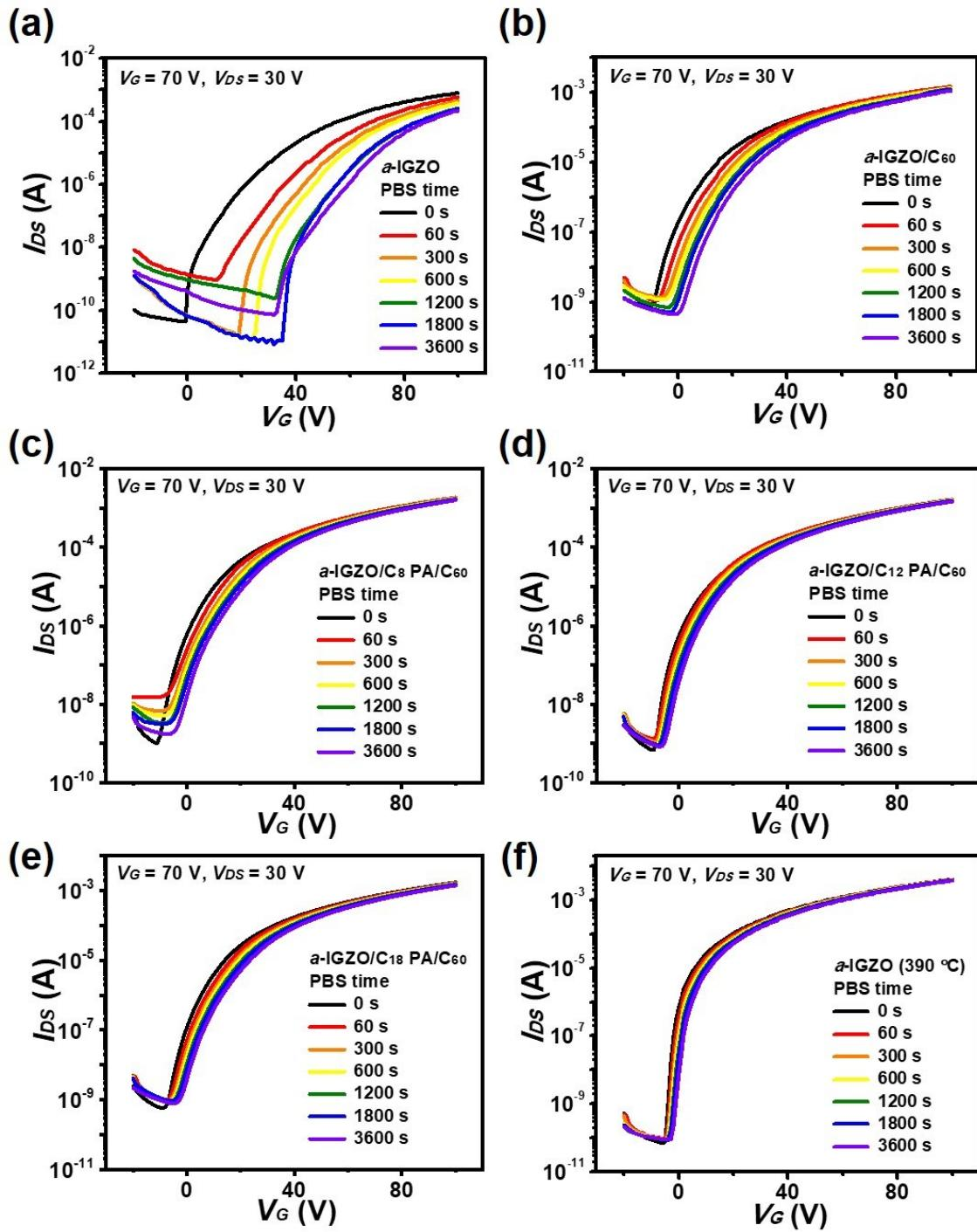
**Fig. S4** Transfer curve shifts during PBS test of (a)  $a\text{-IGZO}$ , (b)  $a\text{-IGZO}/C_{60}$ , (c)  $a\text{-IGZO}/C_8 \text{ PA}/C_{60}$ , (d)  $a\text{-IGZO}/C_{12} \text{ PA}/C_{60}$ , (e)  $a\text{-IGZO}/C_{18} \text{ PA}/C_{60}$ , and (f)  $a\text{-IGZO}$  ( $390^\circ\text{C}$ ) devices.
