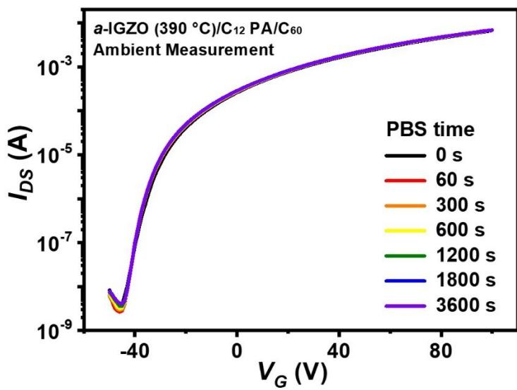
**Fig. S5** Transfer curve shifts during PBS test of ambient measured *a*-IGZO (390 °C)/C<sub>12</sub> PA/C<sub>60</sub>
