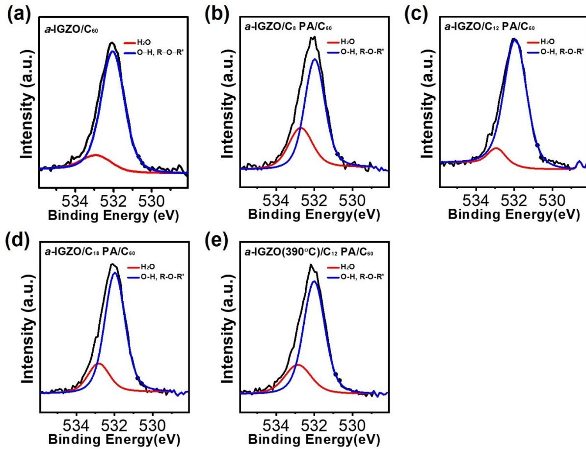
**Fig. S3** O 1s XPS spectra of (a) *a*-IGZO/C<sub>60</sub>, (b) *a*-IGZO/C<sub>8</sub> PA/C<sub>60</sub>, (c) *a*-IGZO/C<sub>12</sub> PA/C<sub>60</sub>, (d) *a*-IGZO/C<sub>18</sub> PA/C<sub>60</sub>, and (e) *a*-IGZO (390 °C)/C<sub>12</sub> PA films.
