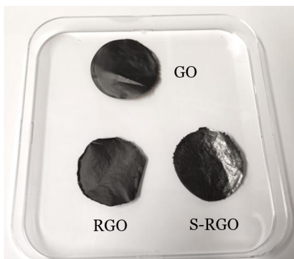
Figure S4. Digital image of free-standing GO, RGO, and S-RGO prepared by vacuum filtration.
