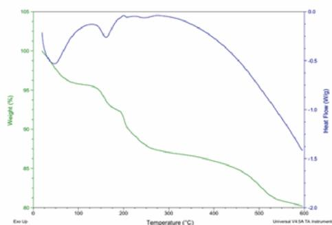
Figure S5. (a) TGA image of gel part that generated with 3.33 wt.% SDS. (b) TGA image of gel part that generated with 35 wt.% SDS.
