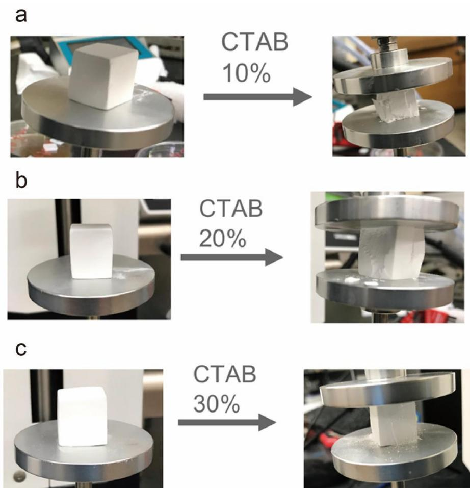
Figure S9. Optical images of (a) 10, (b) 20 and (c) 30 wt.% CTAB samples before and after mechanical compressive test.
