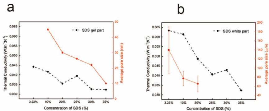
Figure S7. (a) Thermal conductivity of gel part and average pore size changing with increasing the concentration of the surfactant SDS. (b) Thermal conductivity of white part and average pore size changing with increasing the concentration of the surfactant SDS.
