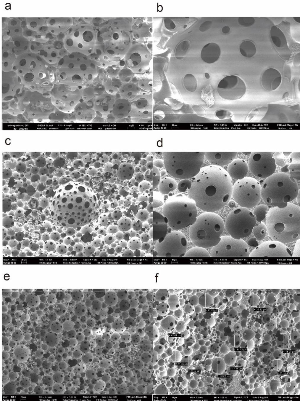
Figure.S6. (a-b) SEM images of opaque aerogel synthesized with 3.33 wt.% SDS at 30  $\mu\text{m}$  and 10  $\mu\text{m}$  respectively; (c-d) SEM images of opaque aerogel synthesized with 10 wt.% SDS at 30  $\mu\text{m}$  and 10  $\mu\text{m}$  respectively; (e-f) Shows SEM images of opaque aerogel synthesized with 20 wt.% SDS at 20  $\mu\text{m}$  and 10  $\mu\text{m}$  respectively.
