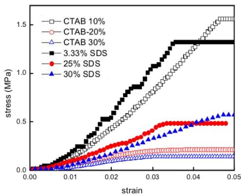
Figure S8. Stress-strain curves show mechanical strength of opaque monolith synthesized with different concentration of surfactant SDS and CTAB.
