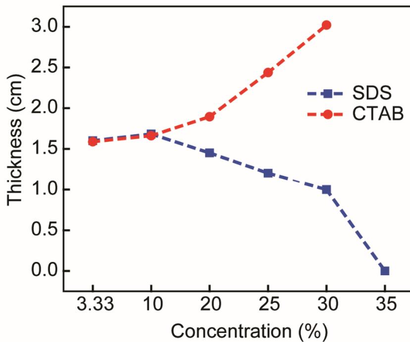
Figure S1. Thickness change of the opaque part with increase of concentration change of surfactant SDS and CTAB.
