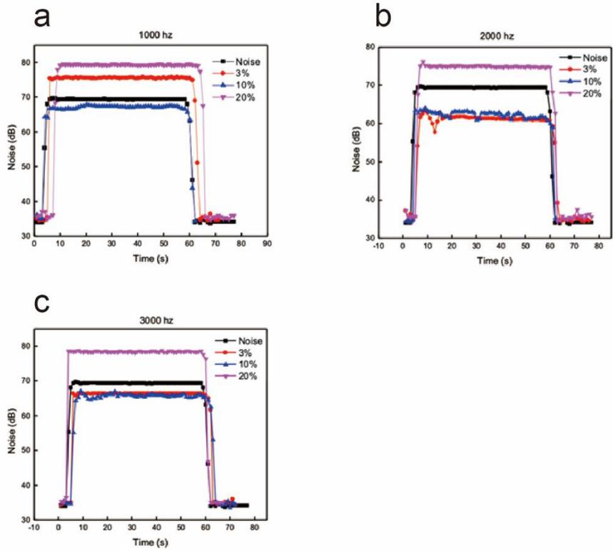
Figure S10. Soundproof performance of different concentration of SDS under sound frequency of (a) 1000 Hz, (b) 2000 Hz, (c) 3000 Hz.
