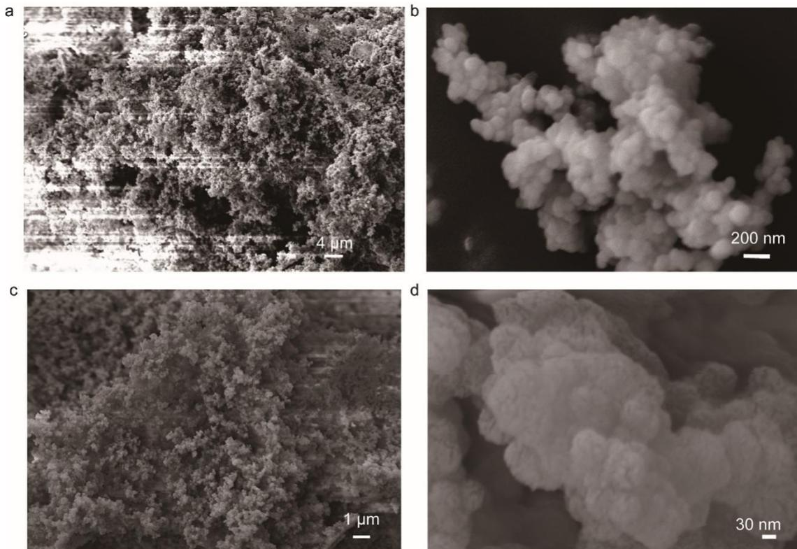
Figure S2. (a-b) SEM images of opaque aerogel synthesized with 10 wt.% CTAB; (c-d) SEM images of opaque aerogel synthesized with 20 wt.% CTAB. Scale bars are labelled in images.
