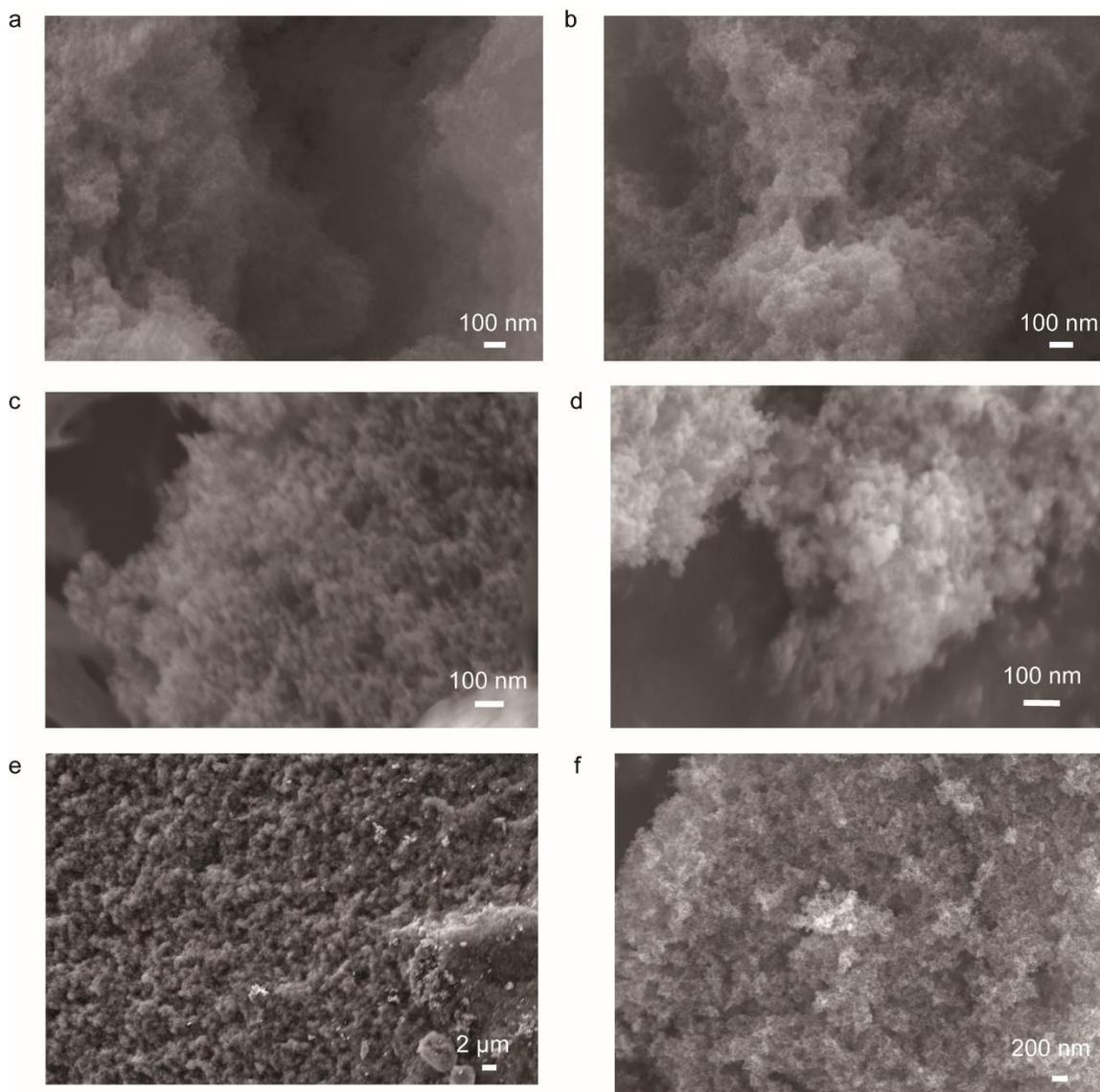
Figure S3. (a-b) SEM images of transparent aerogel synthesized with 3.33 wt.% SDS; (c-d) SEM images of transparent aerogel synthesized with 20 wt.% SDS; (e-f) SEM images of transparent aerogel synthesized with 35 wt.% SDS. Scale bars are labelled in images.
