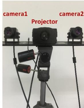
**Fig. S7.** The experimental setup 3D scanner (PD13D) for verifying the accuracy of strain and strain rate detected by the piezoelectric sensor.
