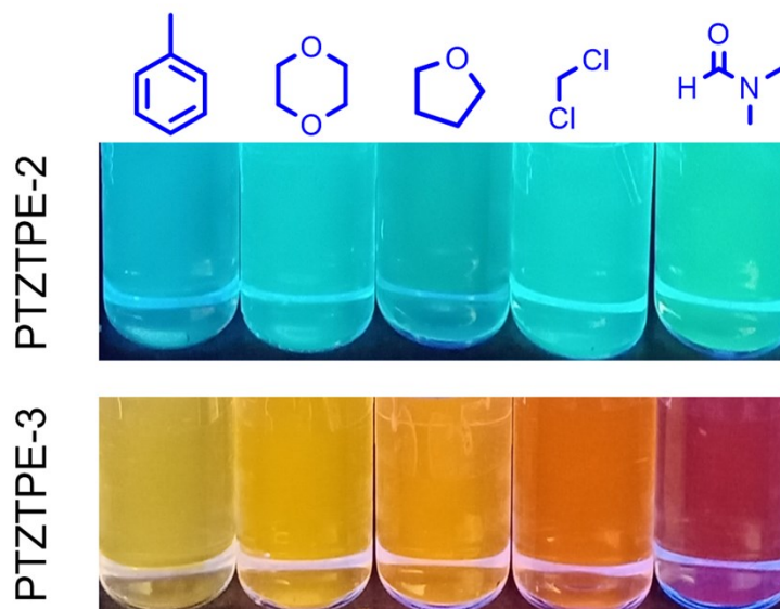
Figure S2 Photograph of compounds PTZTPE-2 and PTZTPE-3 in solvents of different polarity (from left to right, toluene to DMF) taken under 365 nm UV illumination.
