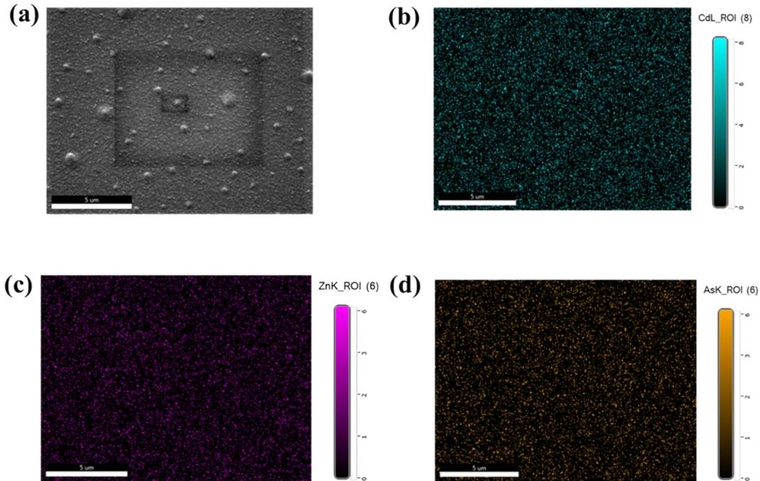
**Fig. S3** EDS mapping of  $(\text{Cd}_{1-x}\text{Zn}_x)_3\text{As}_2$  thin films. (a) Image of test area. (b), (c), (d) The EDS mapping images of Cd, Zn and As element, respectively.
