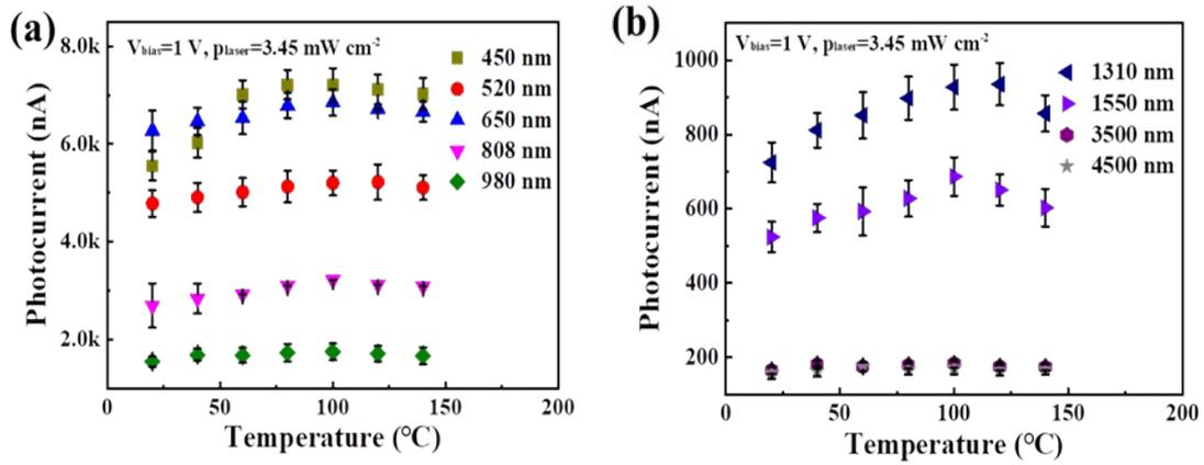
**Fig. S5** (a), (b) The performance influence of different annealing temperatures ( $20^{\circ}\text{C}$ ,  $40^{\circ}\text{C}$ ,  $60^{\circ}\text{C}$ ,  $80^{\circ}\text{C}$ ,  $100^{\circ}\text{C}$ ,  $120^{\circ}\text{C}$ ,  $140^{\circ}\text{C}$ ) on  $(\text{Cd}_{1-x}\text{Zn}_x)_3\text{As}_2/\text{MoO}_3$  thin film heterojunction device.
