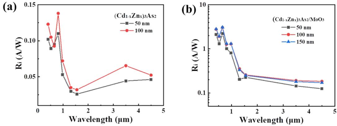
**Fig. S8** (a) The  $R_i$  curves of different thickness  $(\text{Cd}_{1-x}\text{Zn}_x)_3\text{As}_2$  thin film photodetectors at different wavebands. (b) The  $R_i$  curves of 100 nm  $(\text{Cd}_{1-x}\text{Zn}_x)_3\text{As}_2$  with different thickness of  $\text{MoO}_3$  at different wavebands.
