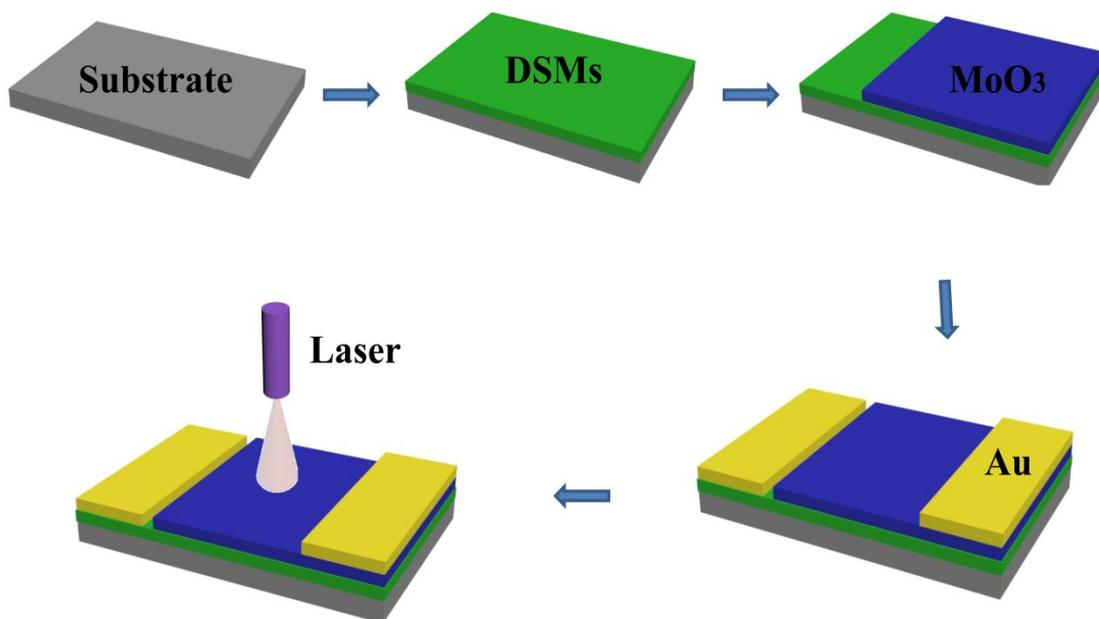
**Fig. S1** Schematic diagram of the fabrication process of DSMs thin film/MoO<sub>3</sub> composite thin film and array device.
