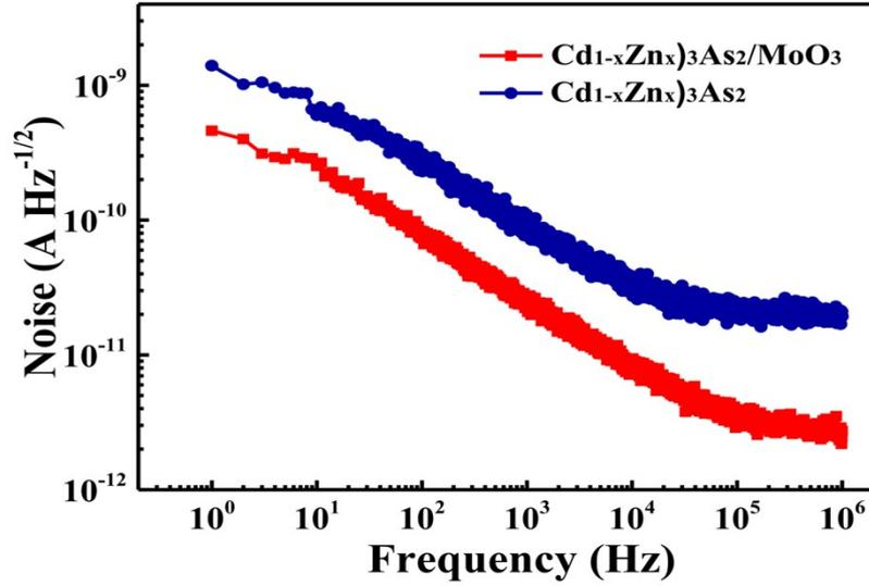
**Fig. S10** The noise diagram of pure DSMs thin film device and DSMs/MoO<sub>3</sub> thin film heterojunction device.
