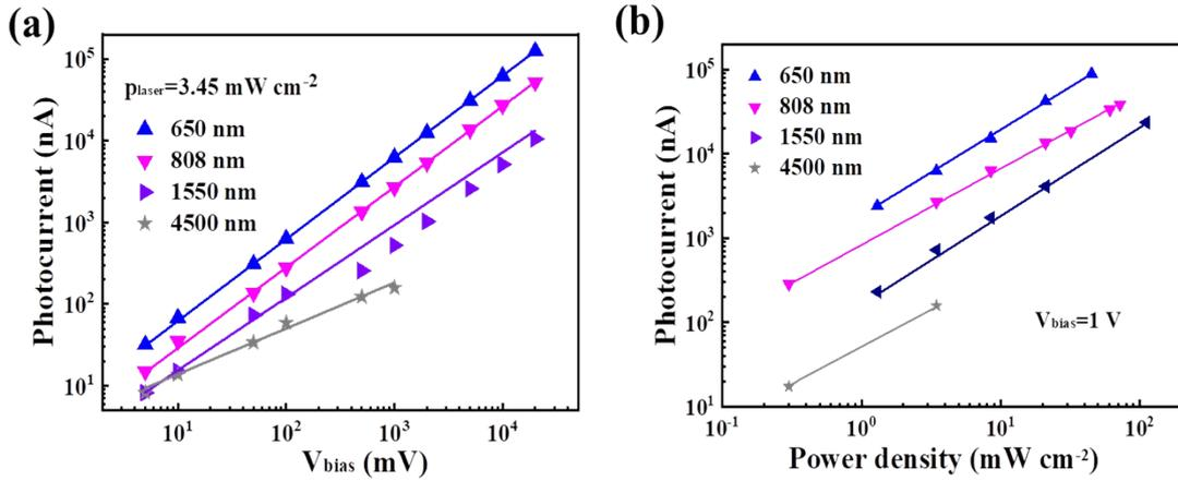
**Fig. S4** (a) The  $I_{ph}$  curves of device as a function under different  $V_{bias}$ . (b) The  $I_{ph}$  curves of device as a function under different power density, while  $V_{bias} = 1 \text{ V}$ .
