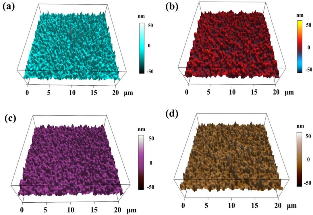
**Fig. S6** (a), (b), (c), (d) The surface topography of  $(\text{Cd}_{1-x}\text{Zn}_x)_3\text{As}_2$  thin film at different temperatures (20 °C, 80 °C, 100 °C, 140 °C). The test area was  $20\ \mu\text{m}\times 20\ \mu\text{m}$ . The RMS roughness of  $(\text{Cd}_{1-x}\text{Zn}_x)_3\text{As}_2$  thin film under different post-growth anneal temperatures is 22.2 nm, 19.3 nm, 17.0 nm, 18.8 nm, respectively.
