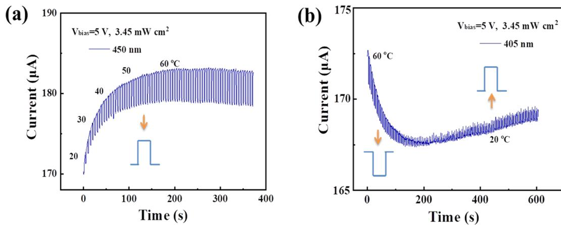
**Fig. S7** Current variation characterization of  $(\text{Cd}_{1-x}\text{Zn}_x)_3\text{As}_2/\text{MoO}_3$  (50 nm/100 nm) device. (a), (b) The heating and cooling process of  $(\text{Cd}_{1-x}\text{Zn}_x)_3\text{As}_2/\text{MoO}_3$  (50 nm/100 nm) device, respectively.
