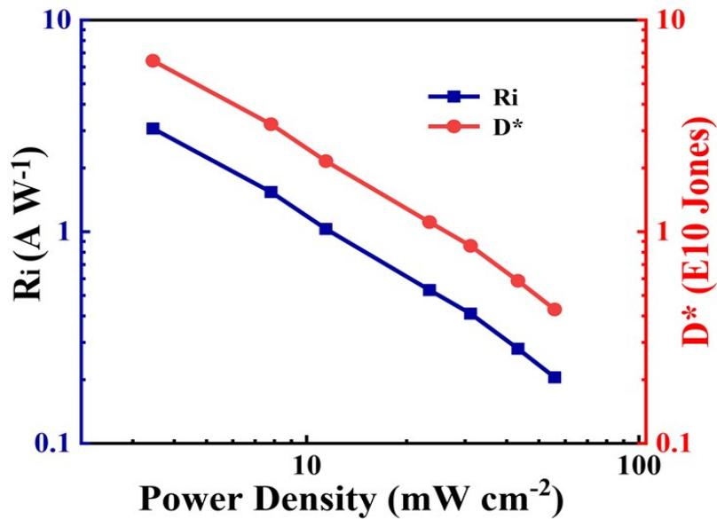
**Fig. S11** The relationship between the  $R_i$  and  $D^*$  of the DSMs/MoO<sub>3</sub> thin film heterojunction device and the laser power density changes. With the decrease of the laser power, the  $R_i$  and  $D^*$  increase linearly.
