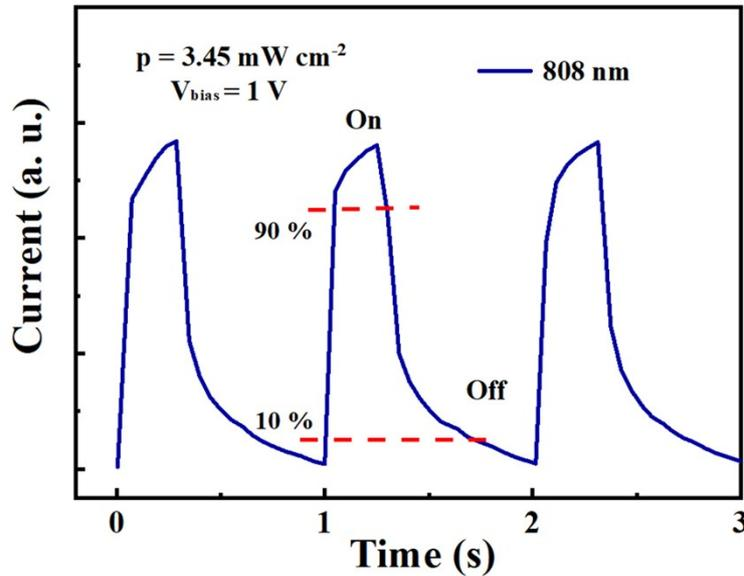
**Fig. S9** The response time of  $(\text{Cd}_{1-x}\text{Zn}_x)_3\text{As}_2/\text{MoO}_3$  heterojunction thin film photodetector @ 808 nm. The rise time ( $\tau_{\text{on}}$ ) and decay time ( $\tau_{\text{off}}$ ) are obtained by defining the time for the photocurrent rising from 10 % to 90 % and declining from 90 % to 10 %, respectively
