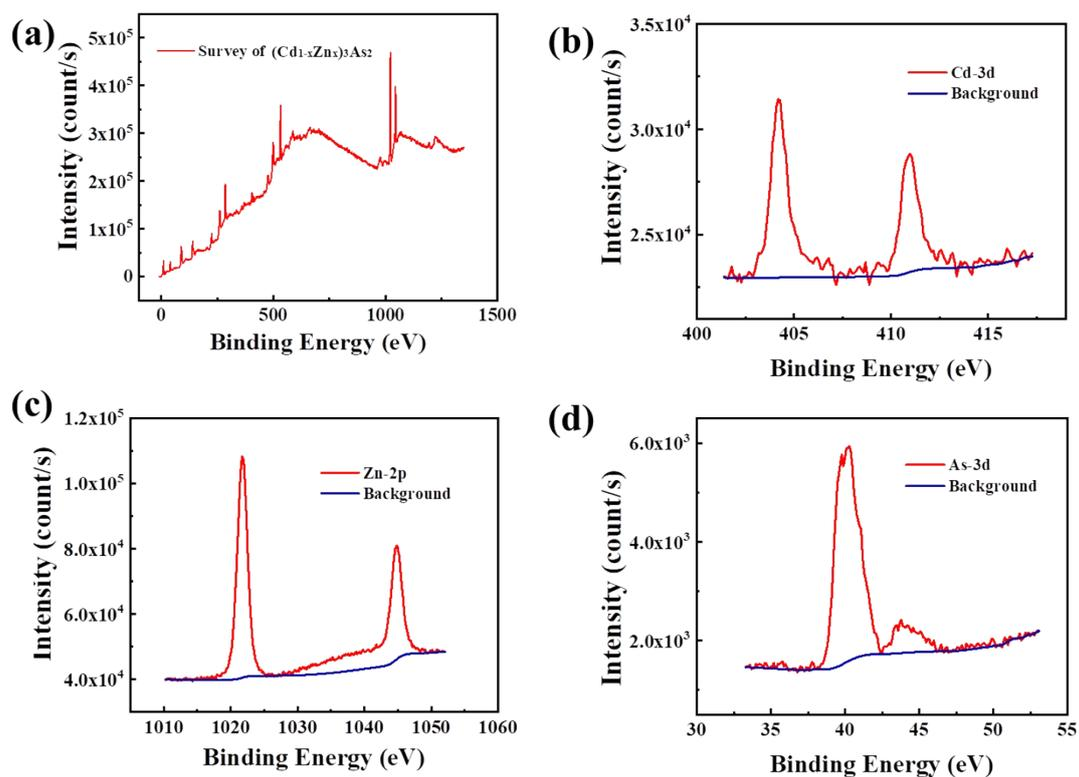
**Fig. S2** XPS pattern of 100 nm Cd<sub>1-x</sub>Zn<sub>x</sub>)<sub>3</sub>As<sub>2</sub> thin film. (a) The XPS survey curve of Cd<sub>1-x</sub>Zn<sub>x</sub>)<sub>3</sub>As<sub>2</sub> thin film. (b),(c),(d) The XPS peak curve of Cd, Zn, As element.
