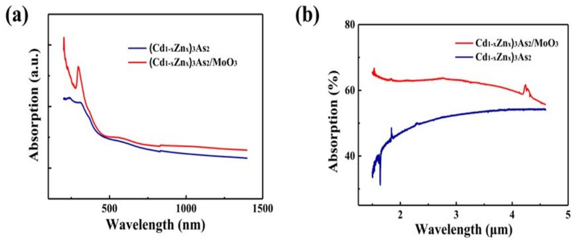
**Fig. S12** The absorption curves of  $(\text{Cd}_{1-x}\text{Zn}_x)_3\text{As}_2/\text{MoO}_3$  combined thin films from VL to MLIR region. (a) The region from 200 nm to 1400 nm. (b) The region from 1.5  $\mu\text{m}$  to 4.6  $\mu\text{m}$ .
