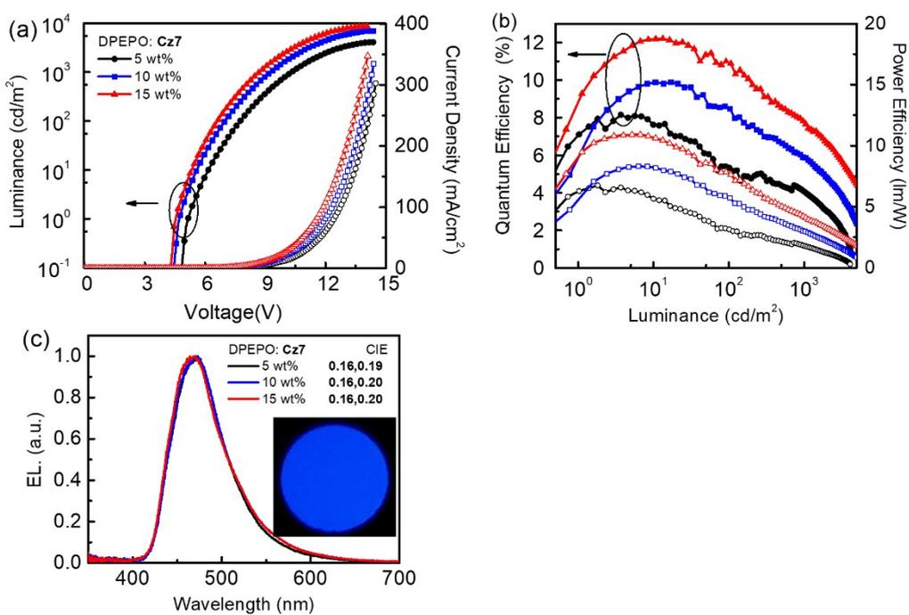
**Figure S5.** (a) J-V-L characteristics, (b) EQE-PE-L characteristics, and (c) normalized EL spectra of devices with DPEPO host doped with x wt.% of Cz7.
