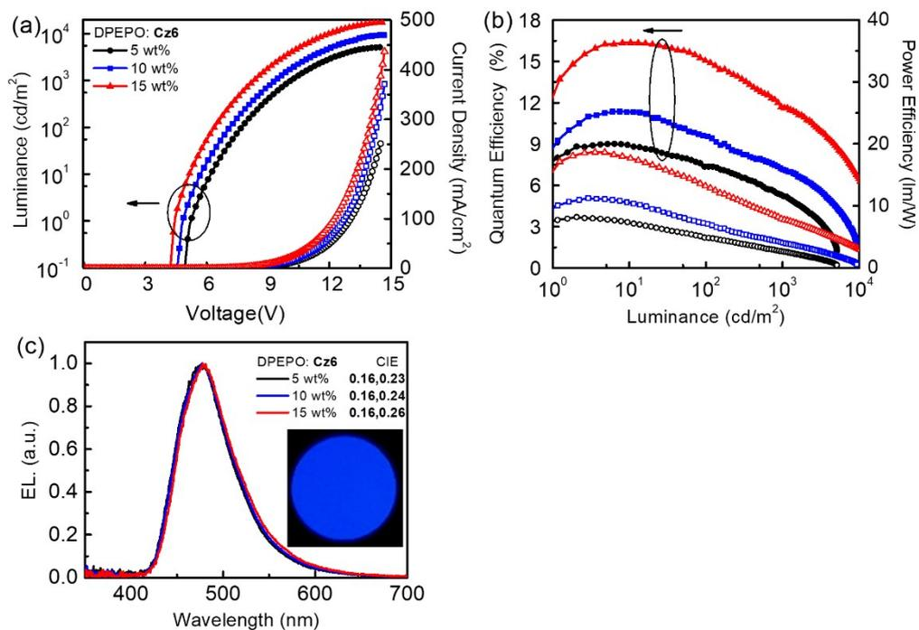
**Figure S4.** (a) J-V-L characteristics, (b) EQE-PE-L characteristics, and (c) normalized EL spectra of devices with DPEPO host doped with x wt.% of Cz6.
