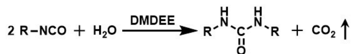
Figure S2. The reaction equation for the reaction of isocyanate groups with moisture to form carbon dioxide.
