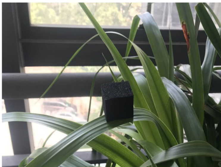
Figure S5. Green leaf stably supports the AgNPs/CNTs-CNCs@TA-PU sponge.
