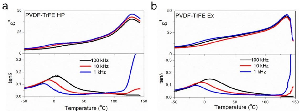
**Figure S2.** The temperature dependence of dielectric permittivity of the (a) hot pressed and (b) extruded PVDF-TrFE films.
