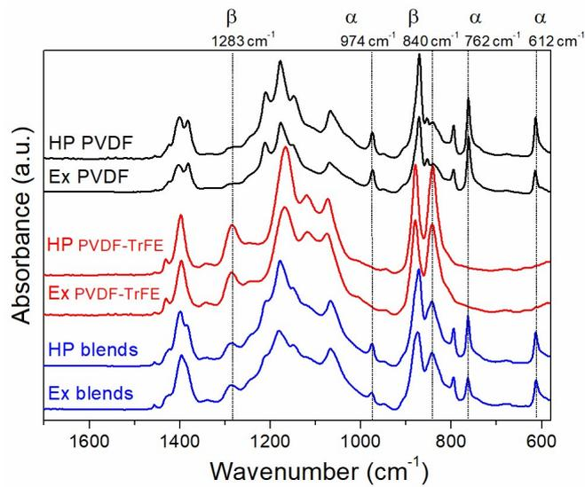
**Figure S1.** FTIR of PVDF, PVDF-TrFE and 50/50 blended films processed via melt-extrusion (Ex) and hot-compression (HP).
