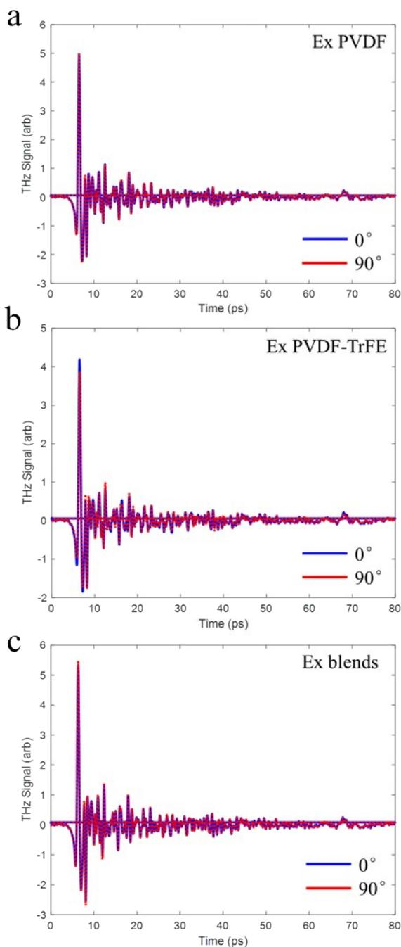
**Figure S4.** The 0° and 90° THz spectroscopy of extruded PVDF, PVDF-TrFE and their blends, which demonstrate that there is no difference in the THz-TDS spectra during the 90° rotation of samples.
