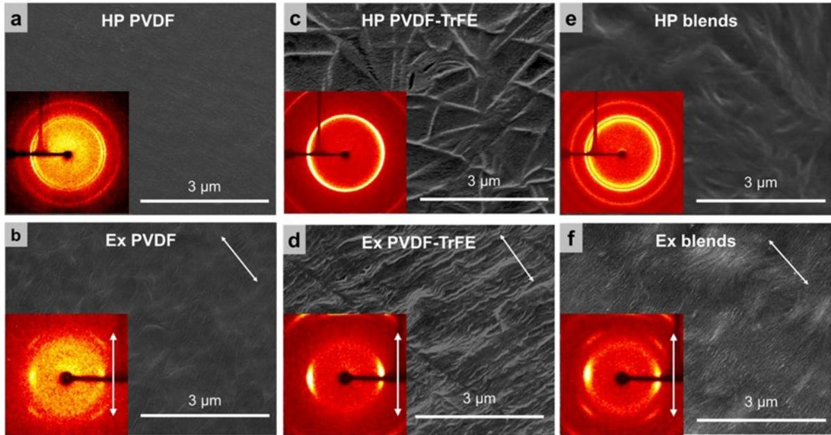
**Figure S3.** Surface SEM morphology images of samples processed using hot-compression (HP) and melt-extrusion (Ex) with the inset images of 2D-XRD ring patterns taken with an incident beam normal to the film surface: (a) HP PVDF; (b) Ex PVDF; (c) HP PVDF-TrFE; (d) Ex PVDF-TrFE; (e) HP blends and (f) Ex blends. The white arrows in SEM images and 2D-XRD ring patterns denote the direction of extrusion.
