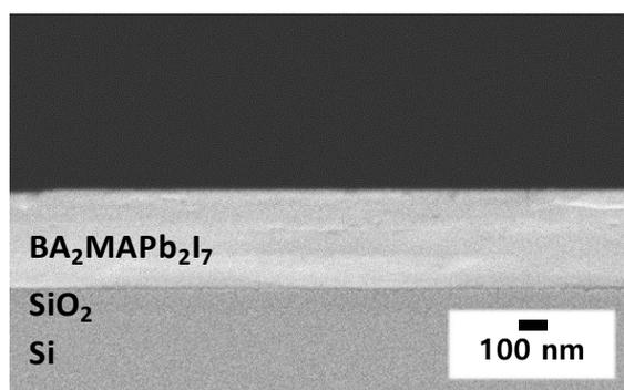
**Fig. S2.** Cross-sectional SEM image of the perovskite film that was formed using  $P_{\text{DMSO}} = 1$ .
