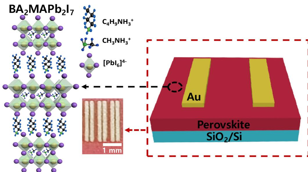
**Fig. S4.** Schematic illustration and optical image of fabricated photodetector device, and the structure of BA<sub>2</sub>MAPb<sub>2</sub>I<sub>7</sub> (atom colors: Pb = yellow; I = purple; C = black; N = green; H = blue).
