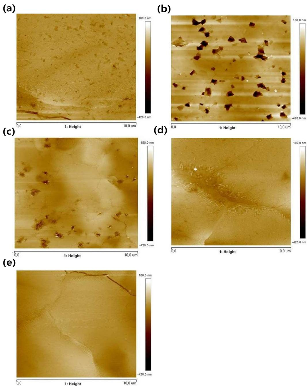
**Fig. S3.** Atomic force microscopy (AFM) images of the films that were cast from (a)  $P_{\text{DMSO}} = 0$ , (b)  $P_{\text{DMSO}} = 0.3$ , (c)  $P_{\text{DMSO}} = 0.5$ , (d)  $P_{\text{DMSO}} = 0.7$ , and (e)  $P_{\text{DMSO}} = 1$ .
