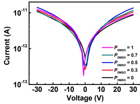
**Fig. S5.** (a)  $I$ - $V$  characteristics of the photodetectors based on  $P_{\text{DMSO}} = 0, 0.3, 0.5, 0.7,$  and  $1$  in darkness.
