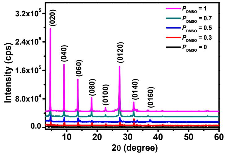
**Fig. S1.** X-ray diffraction patterns of the BA<sub>2</sub>MAPb<sub>2</sub>I<sub>7</sub> films that were cast from  $P_{\text{DMSO}} = 0$ , 0.3, 0.5, 0.7, and 1.
