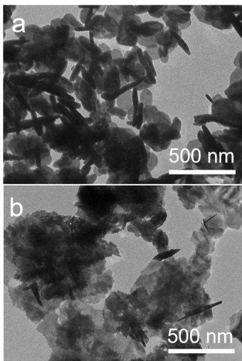
Fig. S4 TEM images of the Bi<sub>2</sub>O<sub>2</sub>Se nanosheets obtained from (a) 9 g NaNO<sub>3</sub>, and (b) 10 g KNO<sub>3</sub>.
