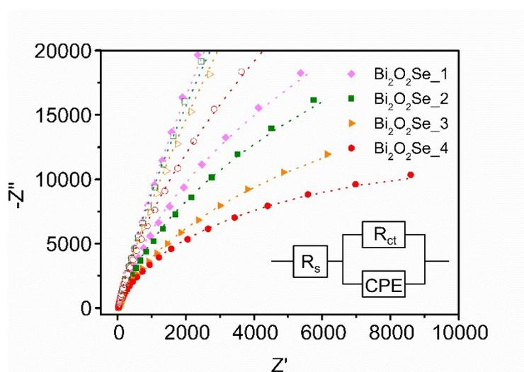
Fig. S9 The fitted plots for the EIS spectra by ZSimpWin software using the proposed equivalent circuit model.
