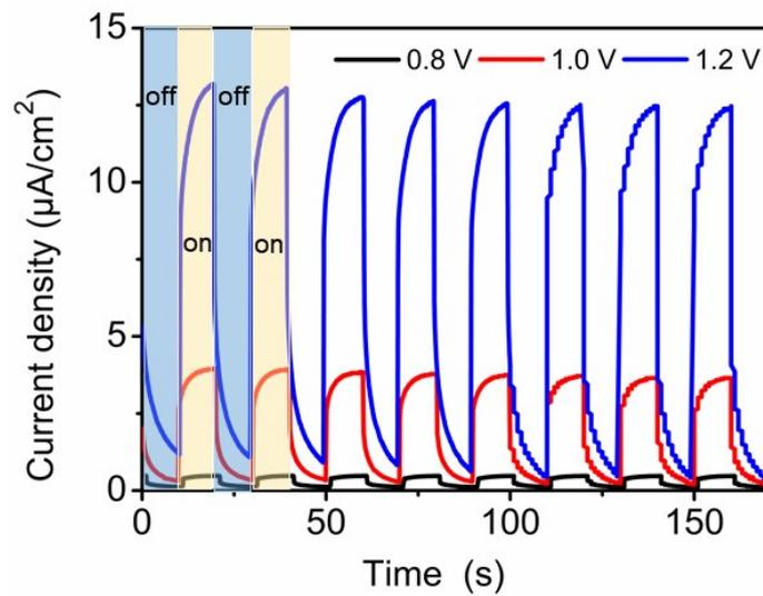
Fig. S6 Time-dependent photocurrent response curves of the Bi<sub>2</sub>O<sub>2</sub>Se<sub>4</sub> photoelectrode at different applied potentials.
