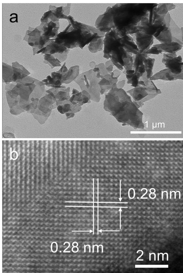
Fig. S11 (a) TEM image and (b) HRTEM image of the  $\text{Bi}_2\text{O}_2\text{Se}_4$  nanosheets after stability test.
