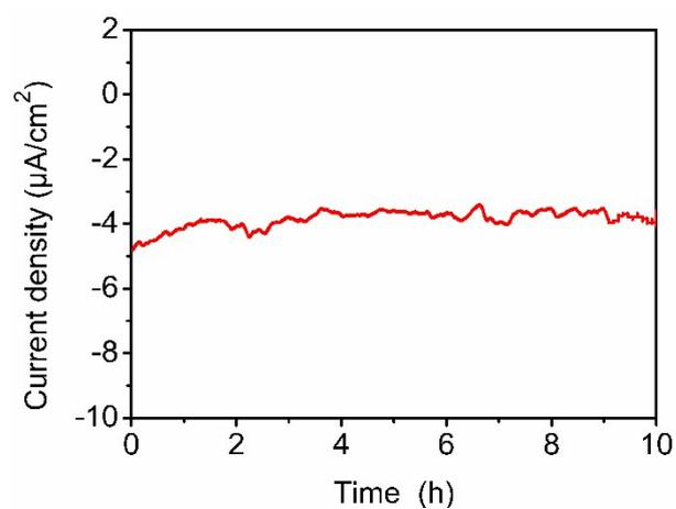
Fig. S10 The amperometric *i*-*t* curve of the Bi<sub>2</sub>O<sub>2</sub>Se<sub>4</sub> electrode with light illumination at applied voltage of 1.0 V.
