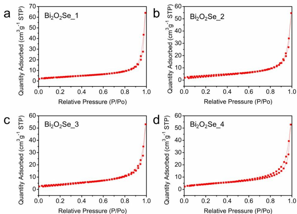
Fig. S8 N<sub>2</sub> adsorption/desorption isotherms of the (a) Bi<sub>2</sub>O<sub>2</sub>Se\_1, (b) Bi<sub>2</sub>O<sub>2</sub>Se\_2, (c) Bi<sub>2</sub>O<sub>2</sub>Se\_3 and (d) Bi<sub>2</sub>O<sub>2</sub>Se\_4 nanosheets. The corresponding BET surface areas are
