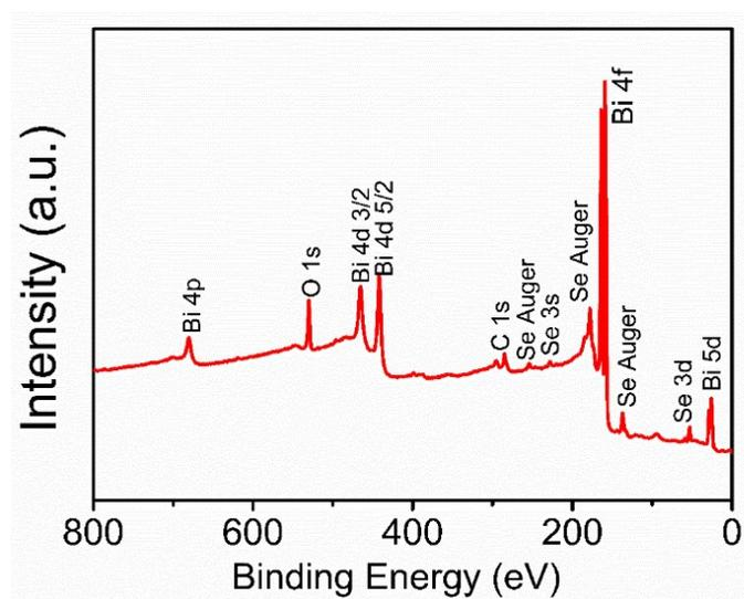
Fig. S1 XPS survey spectrum of the ultrathin Bi<sub>2</sub>O<sub>2</sub>Se nanosheets.
