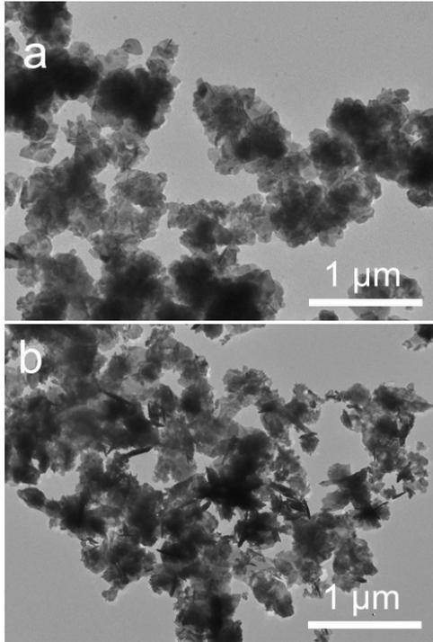
Fig. S5 TEM images of the Bi<sub>2</sub>O<sub>2</sub>Se nanosheets obtained from (a) 6.8 g LiNO<sub>3</sub> and (b) 10 g KNO<sub>3</sub>.
