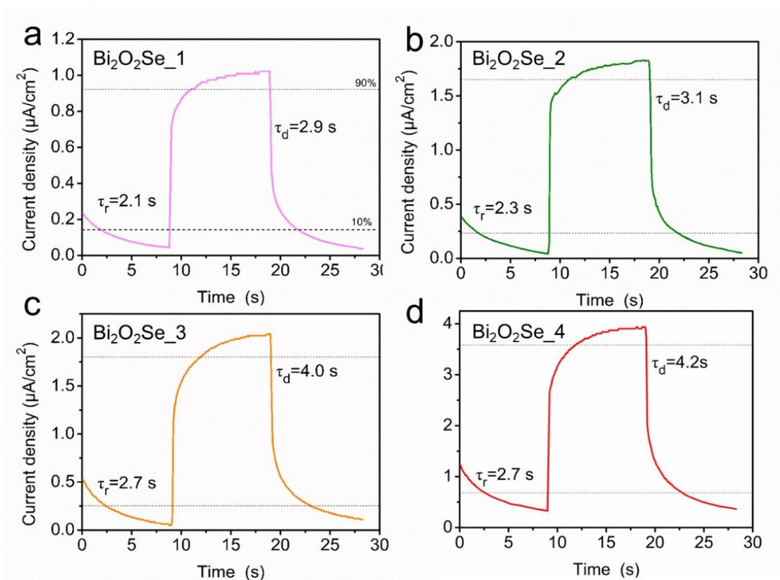
Fig. S7 A single photocurrent response curve with marked rising and decay times for the (a)Bi<sub>2</sub>O<sub>2</sub>Se\_1, (b)Bi<sub>2</sub>O<sub>2</sub>Se\_2, (c)Bi<sub>2</sub>O<sub>2</sub>Se\_3 and (d)Bi<sub>2</sub>O<sub>2</sub>Se\_4 photoelectrodes.
