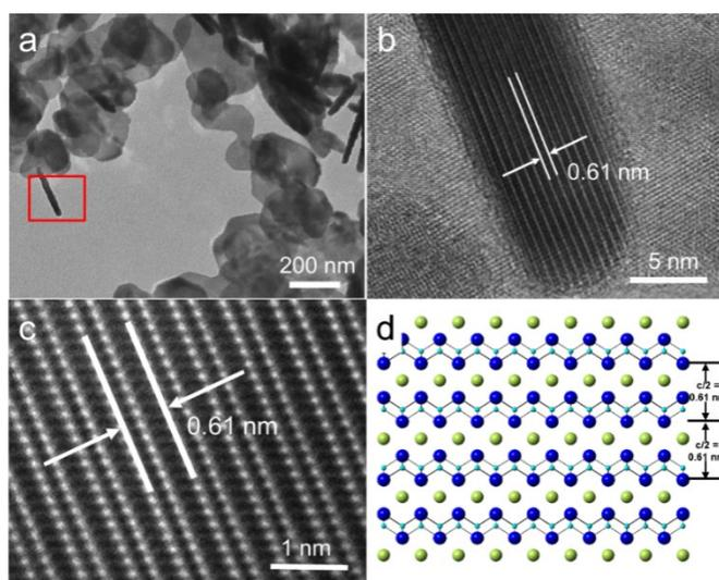
Fig. S2 (a)TEM image of the Bi<sub>2</sub>O<sub>2</sub>Se<sub>2</sub>, (b) HRTEM image of the Bi<sub>2</sub>O<sub>2</sub>Se<sub>2</sub>, from the marked area in a, (c) HAADF-STEM image of the Bi<sub>2</sub>O<sub>2</sub>Se<sub>2</sub> observing from the side direction, (d) side view of Bi<sub>2</sub>O<sub>2</sub>Se crystal structure from [100]. The atomic arrangement in c is not identical to d, due to a rotation in viewing direction.
