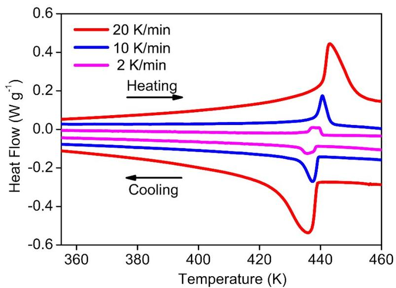
**Figure S5.** Characterizations of the phase transition behavior of **1**. DSC curves measured at different scanning rates.
