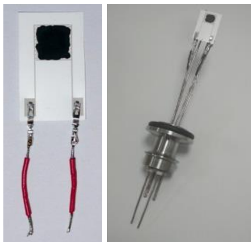
Figure SI 2. Picture of the printed sensors with connection for gas sensing (crocodile clips and soldered electrical wires) and the whole system soldered on the gas chamber feedthrough
