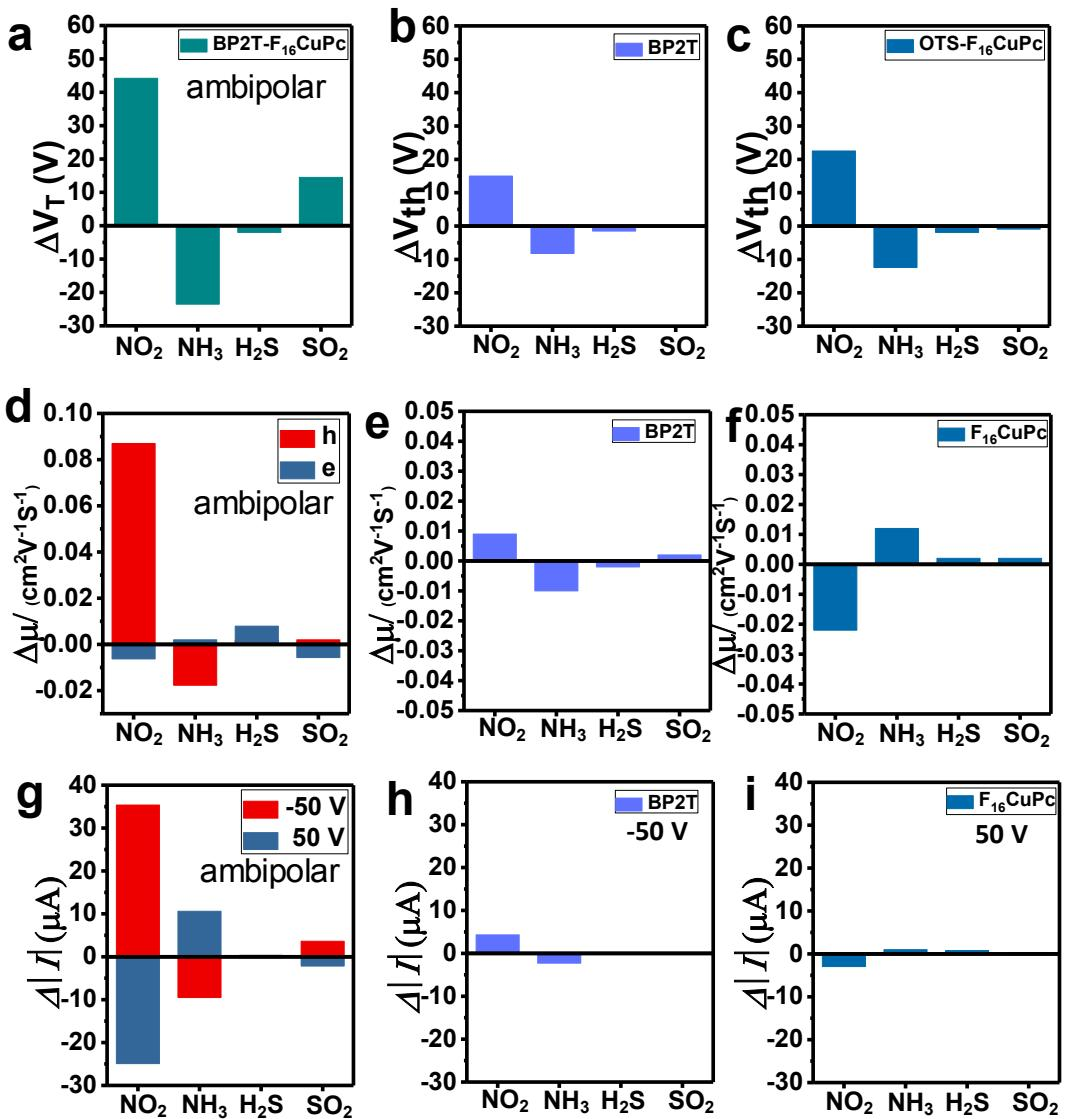
Figure S9. (a-c)  $V_T$  shifting of a) ambipolar OFET device, b)  $V_{th}$  shifting of BP2T based OFET device, c)  $V_{th}$  shifting of F<sub>16</sub>CuPc based OFET device in response to four gases; (d-f) charge mobility changes and (g-i) saturation current changes of d, g) ambipolar, e, h) BP2T, f, i) F<sub>16</sub>CuPc in exposure to 10 ppm  $\text{NO}_2$ , 40 ppm  $\text{NH}_3$ ,  $\text{H}_2\text{S}$  and  $\text{SO}_2$ .
