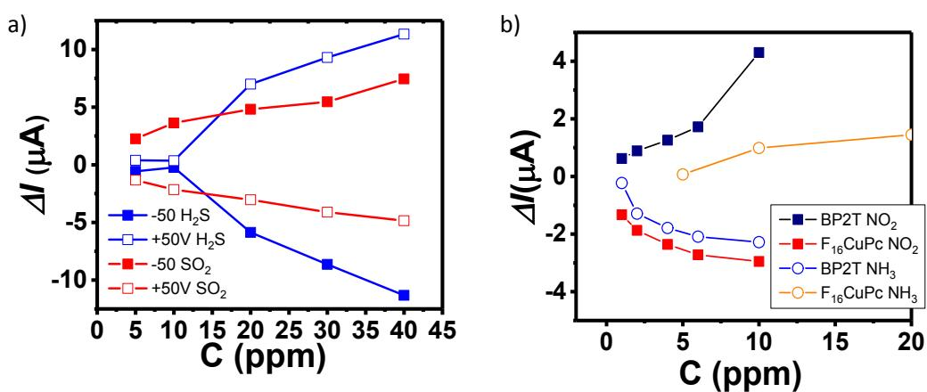
Figure S7. Responses of a) ambipolar b) unipolar OFET-based sensors upon exposure
