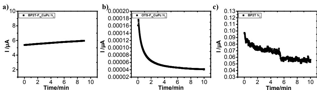
Figure S4 The voltage bias stability of ambipolar and unipolar transistors. a)
