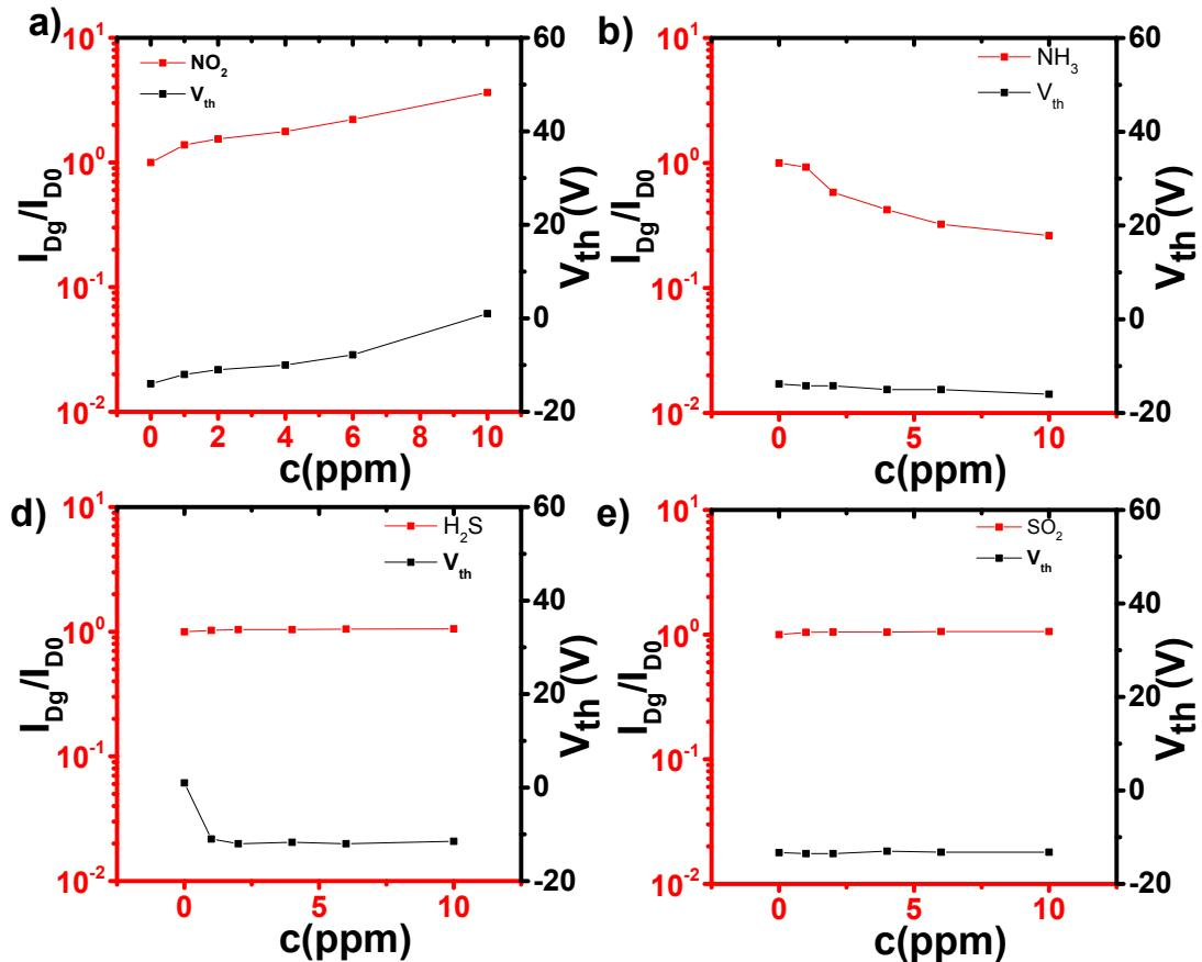
Figure S5. Sensing performance of BP2T OFET-based sensors upon exposure to different vapors. (a-d) the responsivity  $R$  ( $I_{Dg}/I_{D0}$ ) at gate voltage = -50 V and the shift of  $V_{th}$  as the function with various a)  $\text{NO}_2$ , b)  $\text{NH}_3$ , c)  $\text{H}_2\text{S}$ , d)  $\text{SO}_2$  concentrations.
