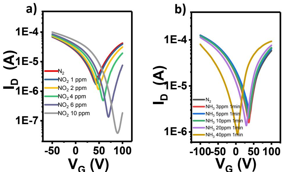
Figure S2. Responses of the ambipolar OFET-based sensors in n-channel transport upon exposure to different vapors at various concentrations. Transfer curves of ambipolar transistor under exposure to a) NO<sub>2</sub>, b) NH<sub>3</sub> at different concentrations.
