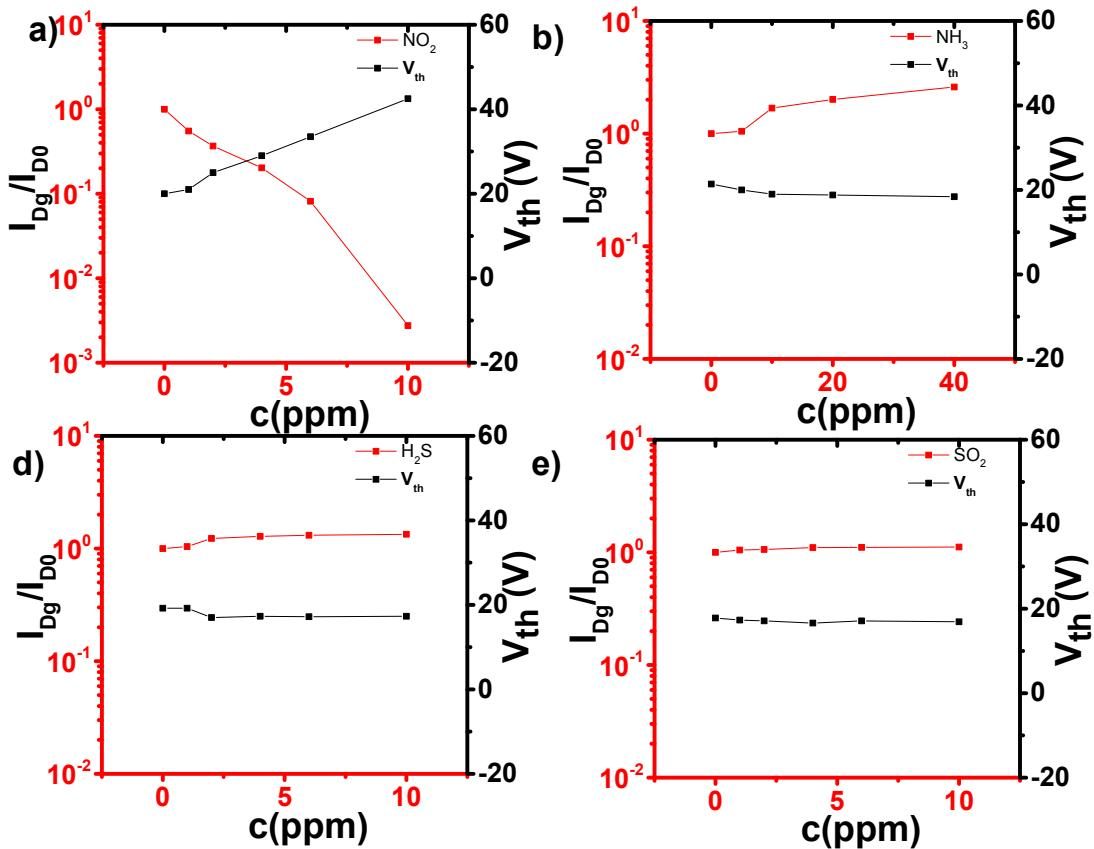
Figure S6. Sensing performance of OTS-F<sub>16</sub>CuPc OFET-based sensors upon exposure to different vapors. (a-d) the responsivity  $R$  ( $I_{Dg}/I_{D0}$ ) at gate voltage = 50 V and the shift of  $V_{th}$  as the function with various a)  $\text{NO}_2$ , b)  $\text{NH}_3$ , c)  $\text{H}_2\text{S}$ , d)  $\text{SO}_2$  concentrations.
