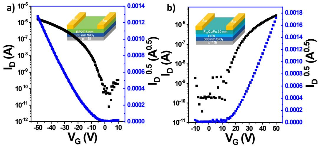
Figure S1. Device configuration of the unipolar transistors and typical transfer characteristic curve of a) BP2T, b) OTS-F<sub>16</sub>CuPc.
