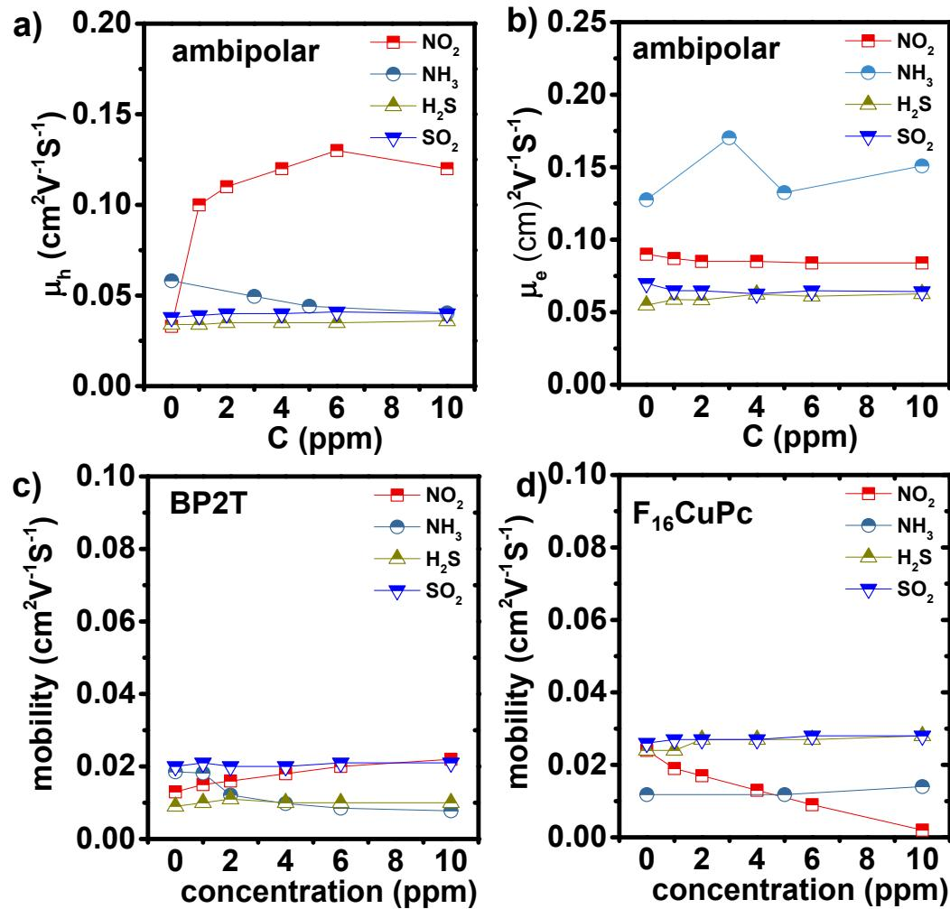
Figure S8. Charge mobility evolution with the gas concentration of the series of transistors. a) Hole and b) electron charge mobility of ambipolar OFET. (c-d) Charge mobility of c) BP2T OFET d) OTS-F<sub>16</sub>CuPc OFET as the function with various gas concentrations.
