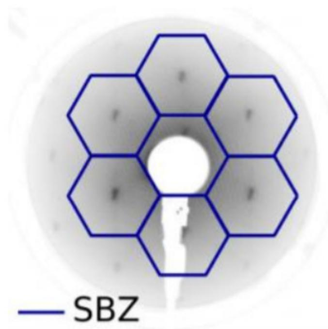
**Figure S6.** Low-energy electron diffraction (LEED) image of a freshly cleaved  $\text{Cd}_3\text{As}_2$  crystal. The first-order diffraction spots are arranged in the pseudo-hexagonal symmetry characteristic of the (112) natural cleavage plane. Blue hexagons denote the surface Brillouin zone (SBZ). Taken from our previous publication on Ref. <sup>1</sup>. (Copyright American Physical Society, 2018)
