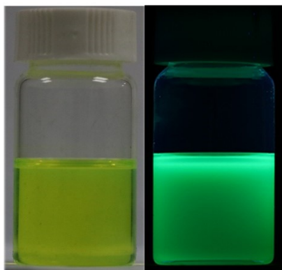
Fig. S1 Photographs of CsPbBr 3 NCs dispersed in toluene under daylight (left) and UV light (right, \lambda = 365 nm).
