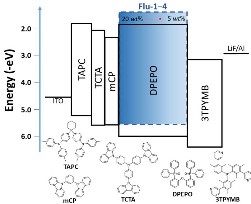
**Fig. S5.** Device configuration and chemical structures of materials used. ITO/TAPC(20 nm)/TCTA (10 nm)/mCP (10 nm)/ DPEPO: 20-5 wt% dopant (30 nm)/3TPYMB (50 nm)/LiF (1 nm)/Al (120 nm), doping concentration of EML (emissive layer) is linearly decreasing from 20 wt% at the mCP/EML interface to 5 wt% at the EML/3TPYMB interface (shown by gradually fading the color and arrow in EML).
