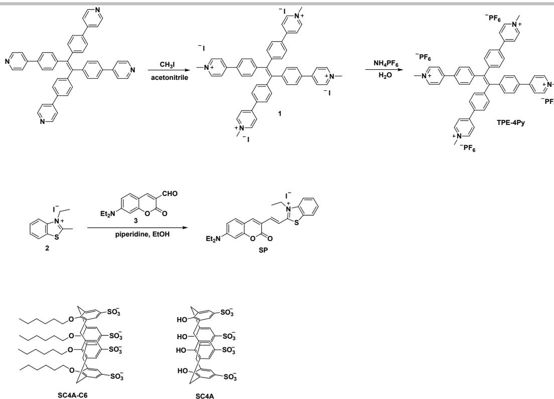
**Scheme S1.** Synthesis of **TPE-4Py** and **SP**, and the structure of **SC4A-C6**, **SC4A**.
