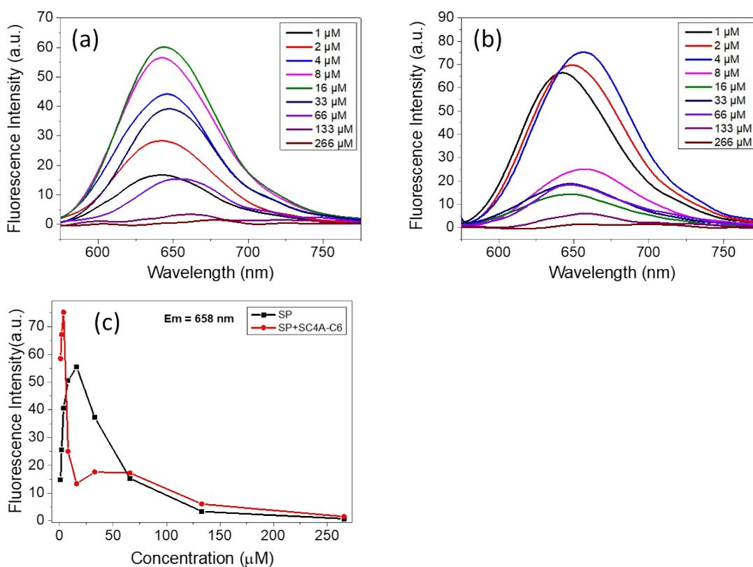
**Figure S12.** Fluorescence spectra of **SP** (a) and **SC4A-C6/SP** (b) at different concentrations in PBS buffer solution. (c) The fluorescence intensity of **SP** and **SC4A-C6/SP** at 658 nm in different concentration. ( $\lambda_{\text{ex}}$  = 533 nm; slit: 2.5/5 nm).
