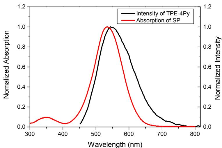
**Figure S8.** Normalized emission spectrum of **TPE-4Py** and absorption spectrum of **SP**.
