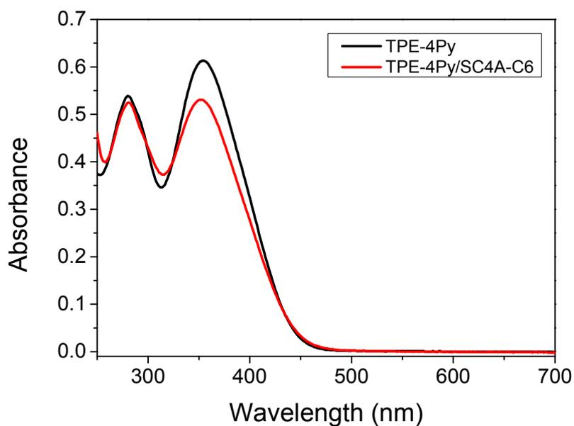
**Figure S2.** UV-vis absorption spectrum of **TPE-4Py** (14  $\mu$ M) and **TPE-4Py/SC4A-C6** ([**SC4A-C6**] = 12  $\mu$ M, [**TPE-4Py**] = 14  $\mu$ M) in PBS buffer solution.
