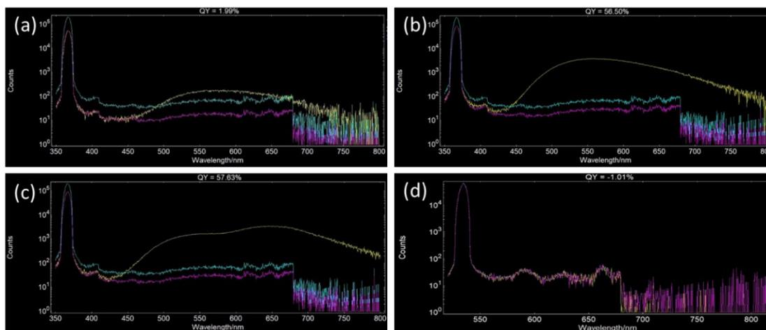
**Figure S7.** Quantum yields of (a) TPE-4Py, (b) TPE-4Py/SC4A-C6, (c) TPE-4Py/SC4A-C6/SP and (d) SP in PBS buffer solution (pH 7.4, 10 mM).
