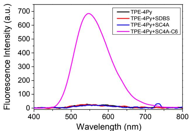
**Figure S6.** Fluorescence spectra of TPE-4Py (12  $\mu$ M) in the presence SC4A (14  $\mu$ M); SC4A-C6 (14  $\mu$ M), SDBS [sodium dodecyl benzene sulfonate (14  $\mu$ M)] in PBS buffer solution ( $\lambda_{\text{ex}}$  = 365 nm; slit: 2.5/5 nm).
