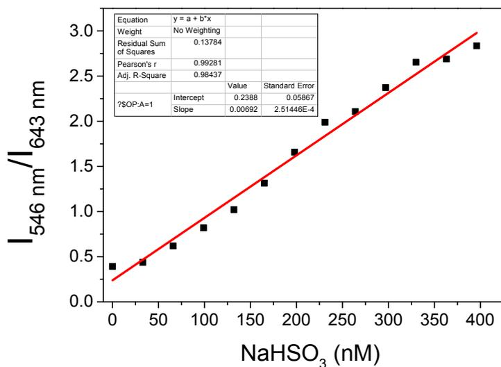
**Figure S13.** Fluorescent intensity ratio ( $I_{546 \text{ nm}}/I_{643 \text{ nm}}$ ) changes of **TPE-4Py/SC4A-C6/SP** as a function of the concentration of  $\text{NaHSO}_3$  in PBS buffer (pH 7.4, 10 mM). Each spectrum was recorded after 8 min ( $\lambda_{\text{ex}} = 365 \text{ nm}$ ; slits: 2.5/5 nm).
