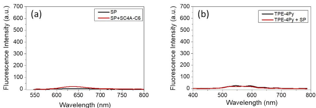
**Figure S9.** Fluorescence spectra of **SC4A-C6/SP** (**[SC4A-C6]** = 12  $\mu$ M, **[SP]** = 216 nM) and **TPE-4Py/SP** (**[TPE-4Py]** = 12  $\mu$ M, **[SP]** = 216 nM) in PBS buffer solution (10 mM, pH 7.4). (a) ( $\lambda_{\text{ex}}$  = 533 nm slit: 2.5/5 nm); (b) ( $\lambda_{\text{ex}}$  = 365 nm; slit: 2.5/5 nm).
