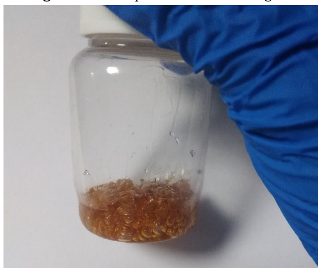
Figure S2. The eugenol-containing polysiloxane prepared by Hydrosilylation-PR process.
